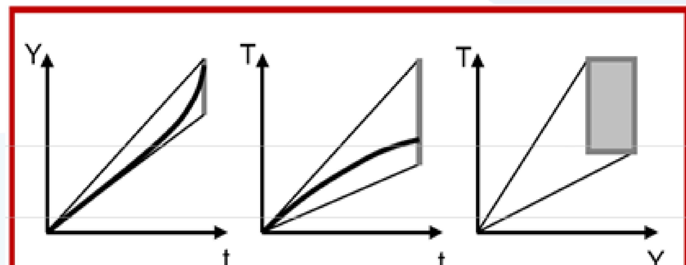
In retrospect, the simplest linear dynamical emission-temperature model is able to forecast precisely only intervals for emissions,  $Y$ , (left) and temperature,  $T$ , (middle). As a result, we get an unsharp emission-temperature forecast – the grey square in the  $(Y, T)$  plane (right).
