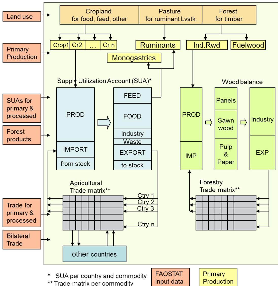
LANDFLOW operates on an annual basis. It uses for calculations a detailed commodity list and then generates results for aggregate commodity groups allowing a complete land balance of agricultural and forestry production. In addition, flows of selected important commodities of interest can be traced separately.
