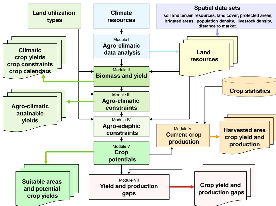
Overall model structure and data integration of GAEZ v3.0 (Module I-VII)
