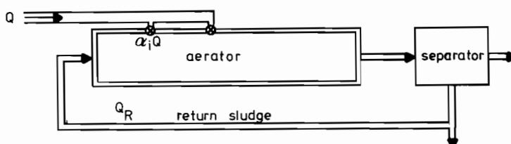
Fig. 6.2 The activated sludge process.
