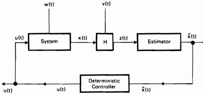
Fig. 2 Optimal closed-loop control showing the separation principle.
