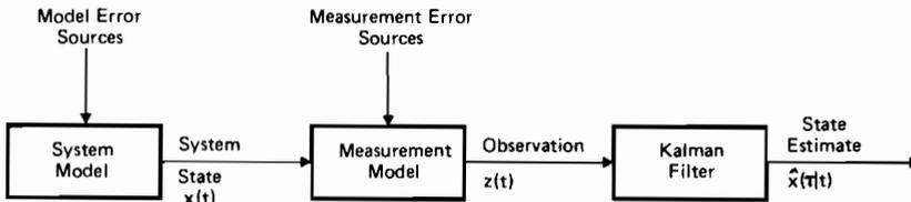
Fig. 1.1 Procedure of system measurement and estimation (after Gelb, 1974).
