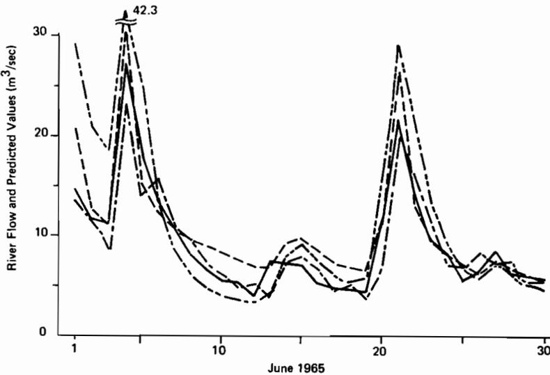
Fig. 10.6 The tracking behavior of predicted values  $q_4(t)$  and  $q_5(t)$  from hydrologic models together with  $q_3(t)$  and the actual flow  $q(t)$ . — =  $q(t)$ ; - - - =  $q_3(t)$ ; - · - · =  $q_4(t)$ ; - - - - =  $q_5(t)$ . Reprinted, by permission, from Ikeda et al. (1976a).
