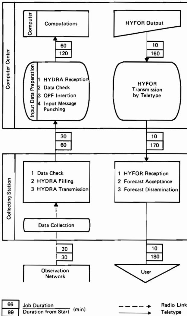
Fig. 17.5 A diagram of data collection, transmission, processing, and dissemination for the Sola and Dunajec River forecasting systems. HYDRA is the input data message; HYFOR is the output data message. QPF stands for quantitative precipitation forecasts.
