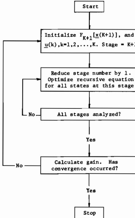
Fig. 13.4 General flowchart of the algorithm for computation of the gain of the system.
