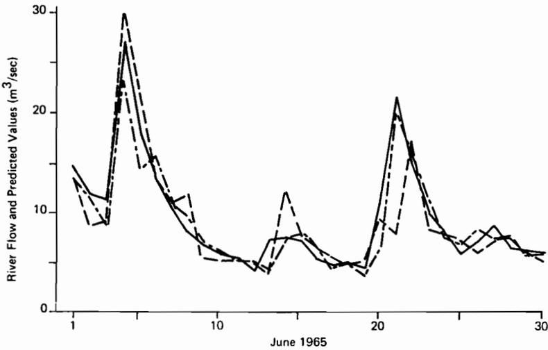
Fig. 10.5 The tracking behavior of predicted values  $q_i(t)$  ( $i = 2,3$ ) together with the actual flow  $q(t)$ .
