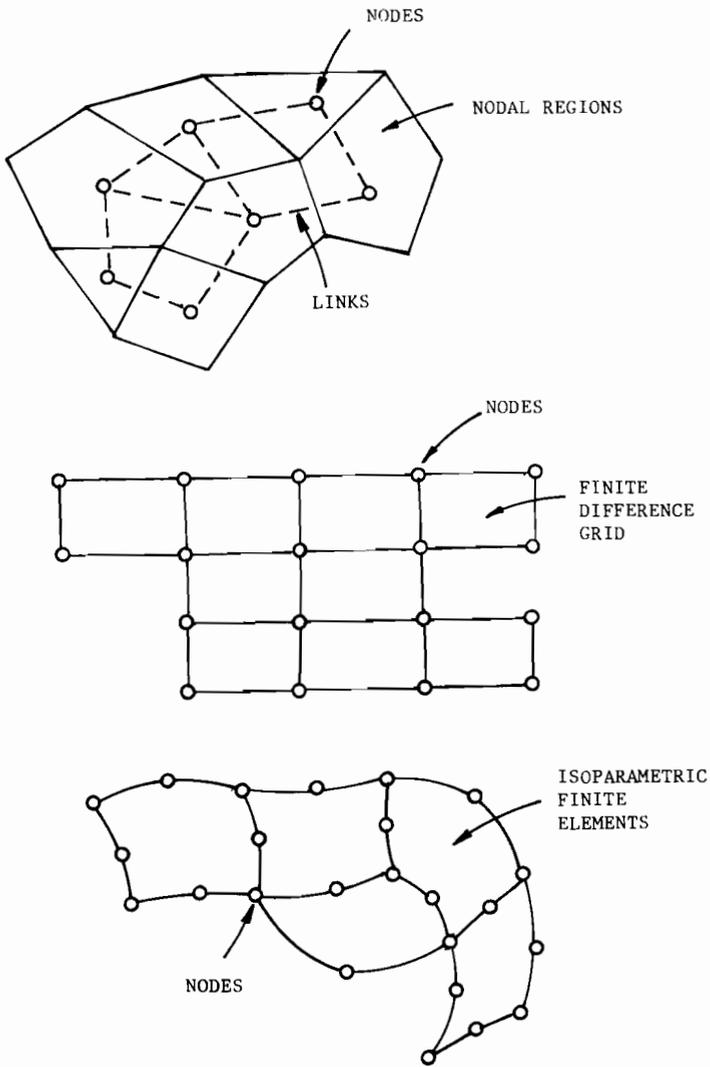
Fig. 7.1 Common spatial techniques for making equations discrete.
