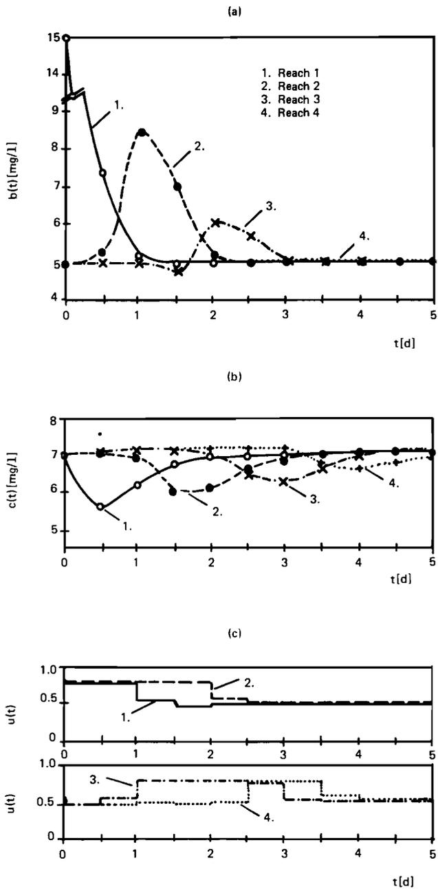
Fig. 14.4 Optimal emergency control. (a) BOD, (b) DO, (c) treatment efficiency and BOD discharge (from Rinaldi et al. 1978).
