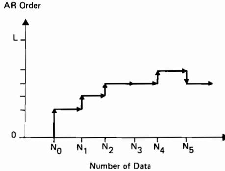
Fig. 3.2 Evolution of the AR model with increasing data.
