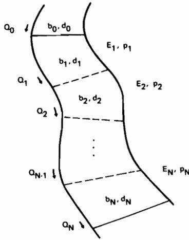
Fig. 3.1 A stretch of a river composed of N reaches.
