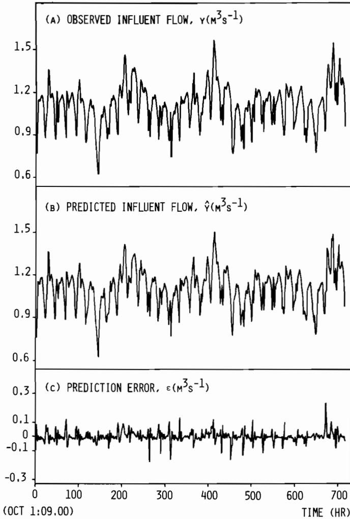
Fig. 11.13 The results of the one-step-ahead predictor for data for the month of October 1973 from the K ppala sewer system in Stockholm: (A) observed influent flow  $y(\text{m}^3\text{sec}^{-1})$ ; (B) predicted influent flow  $\hat{y}(\text{m}^3\text{sec}^{-1})$ ; (C) prediction error  $\epsilon(\text{m}^3\text{sec}^{-1})$ .
