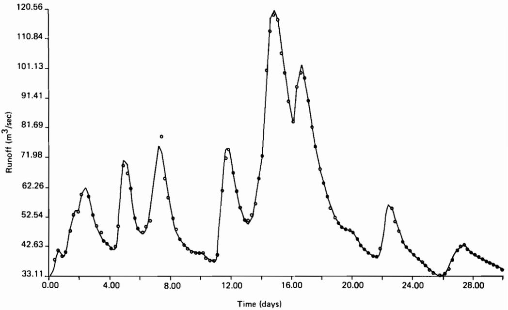
Fig. 9.5 One-step-ahead self-tuning predictor for the Brosna Catchment with  $m = 2$ ,  $n = 2$ , and  $l = 2$ .
