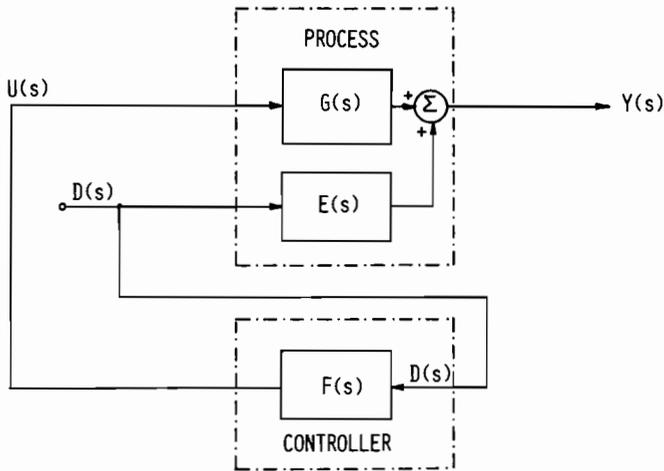
Fig. 11.7 The feedforward controller principle.
