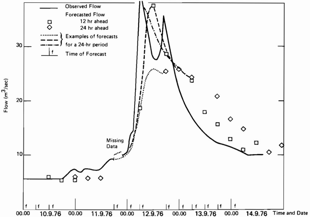
Fig. 16.9 Specimen hydrograph and forecasts of the Dee at Manley Hall for September 10 to 13, 1976 (from the Dee Weather Radar and Real-Time Hydrological Forecasting Project Report 1977).
