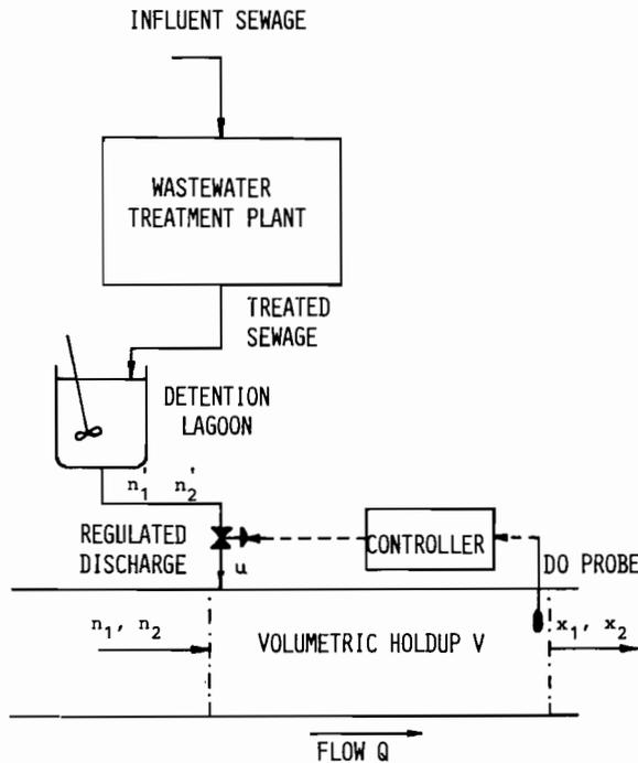
Fig. 11.9 A schematic diagram for in-stream DO control by flow detention of treated effluent; all variables are as defined for Eqs. (11.12) and (11.13).
