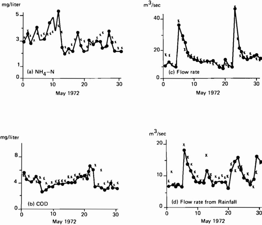
Fig. 10.8 One-day-ahead forecasts of water quality by the modified GMDH. (a)  $\text{NH}_4\text{-N}$  concentration; (b) COD concentration; (c) and (d) flow rates. ● - observed value; x - predicted value.
