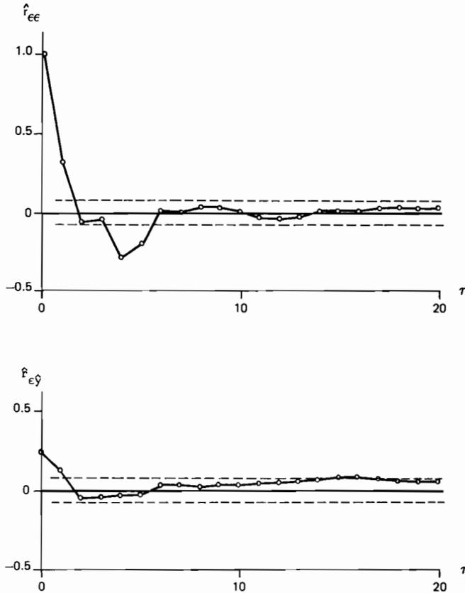
Fig. 9.1 Two-step ahead self-tuning predictor with  $n = 3$ ,  $m = 2$ , and  $l = 2$ . The dashed lines indicate the 95% confidence interval in which the covariances can be regarded as zero.  $\hat{f}_{\epsilon\epsilon}$  is the autocorrelation function and  $\hat{f}_{\epsilon\hat{y}}$  is the cross-correlation function.
