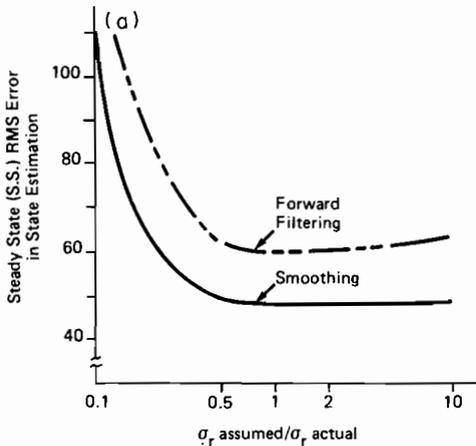
Fig. 2.4a Effect of errors in measurement noise variance on steady-state RMS error in state estimation.  $\sigma_r$  = measurement noise standard deviation. (from Mehra 1968).
