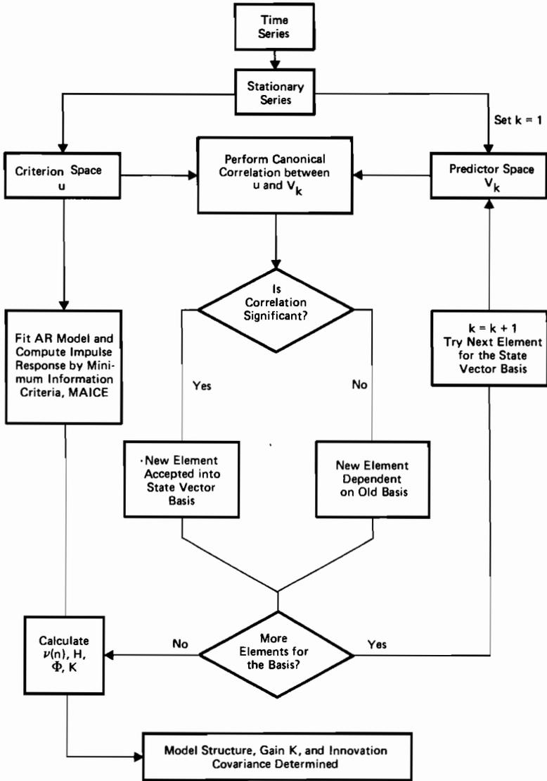
Fig. 2.7 Akaike's procedure for model structure determination in MIMO linear systems.
