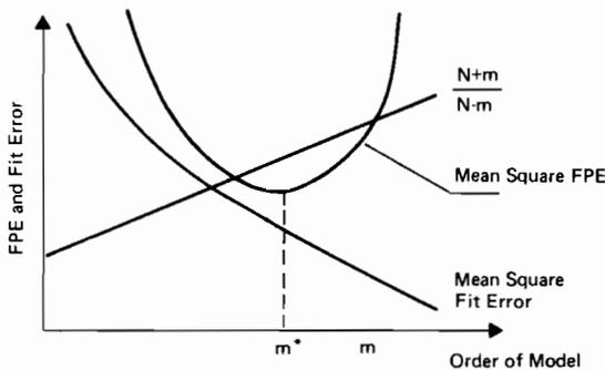
Fig. 2.6 Final prediction error and fit error versus order of the AR model.  $M^*$  is the optimal order of the models.
