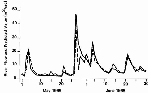
Fig. 10.4 The tracking behavior of predicted value  $q_1(t)$  together with the actual flow  $q(t)$ . — =  $q(t)$ ; --- =  $q_1(t)$ . Reprinted, by permission, from Ikeda et al. (1976a).
