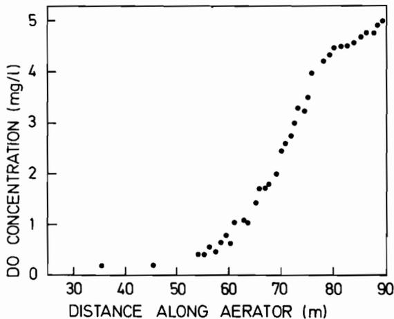
Fig. 6.3 Typical profile of dissolved oxygen in the activated sludge process of the Käppala wastewater treatment plant, Stockholm.
