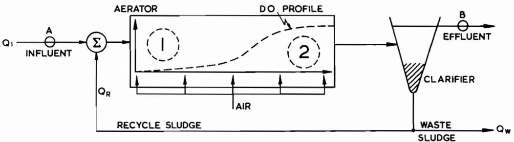
Fig. 11.12 A schematic diagram of the activated sludge process; zone 1 in the aerator is potentially an anaerobic environment; zone 2 is a predominantly aerobic environment.
