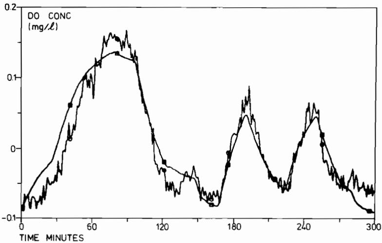
Fig. 6.5 Dissolved oxygen levels in an experiment in the Käppala wastewater treatment plant. The experimental DO output is compared with a first-order model output. The water flow rate and the MLSS concentration (see Fig. 6.4) are the inputs.
