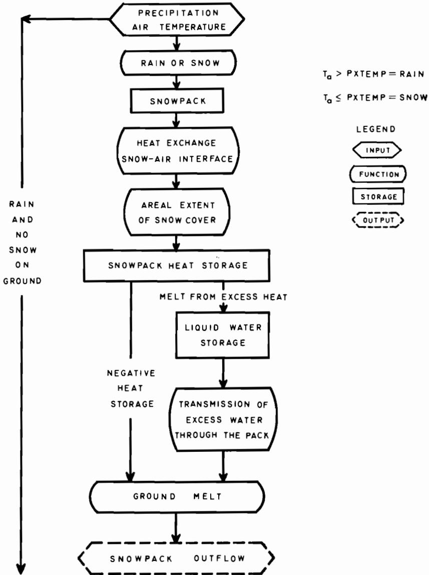
Fig. 18.5 Snow accumulation and ablation model.
