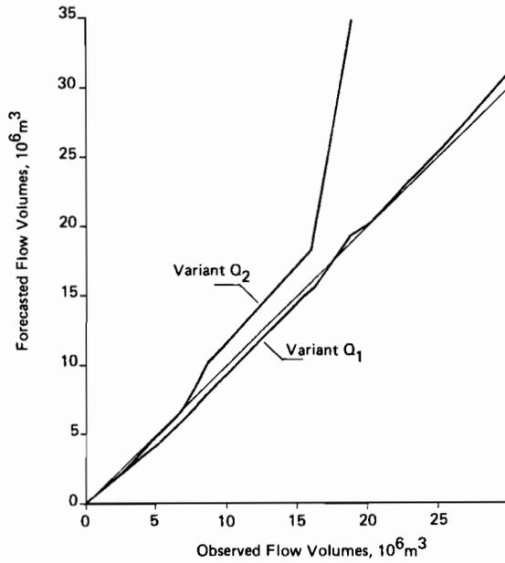
Fig. 17.7 A double mass plot of forecasted versus observed monthly flow volumes. (Dunajec River, cross section Kowaniec, 1-31 July 1976).
