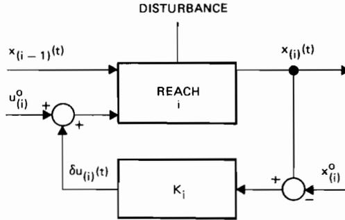
Fig. 14.1 Structure of the local feedback control scheme resulting from the second variation problem (from Rinaldi et al. 1978).
