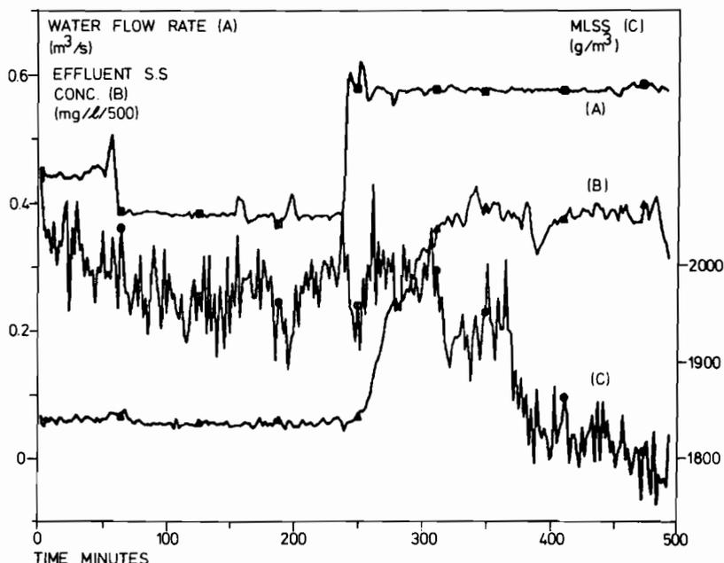
Fig. 6.1 Input and output signals of a water flow experiment in a wastewater treatment plant. The water flow rate (A) has been manipulated, causing the effluent suspended solids (SS) concentration to vary (B). The mixed liquor suspended solids (MLSS) concentration (C) is also affected by the water flow change.
