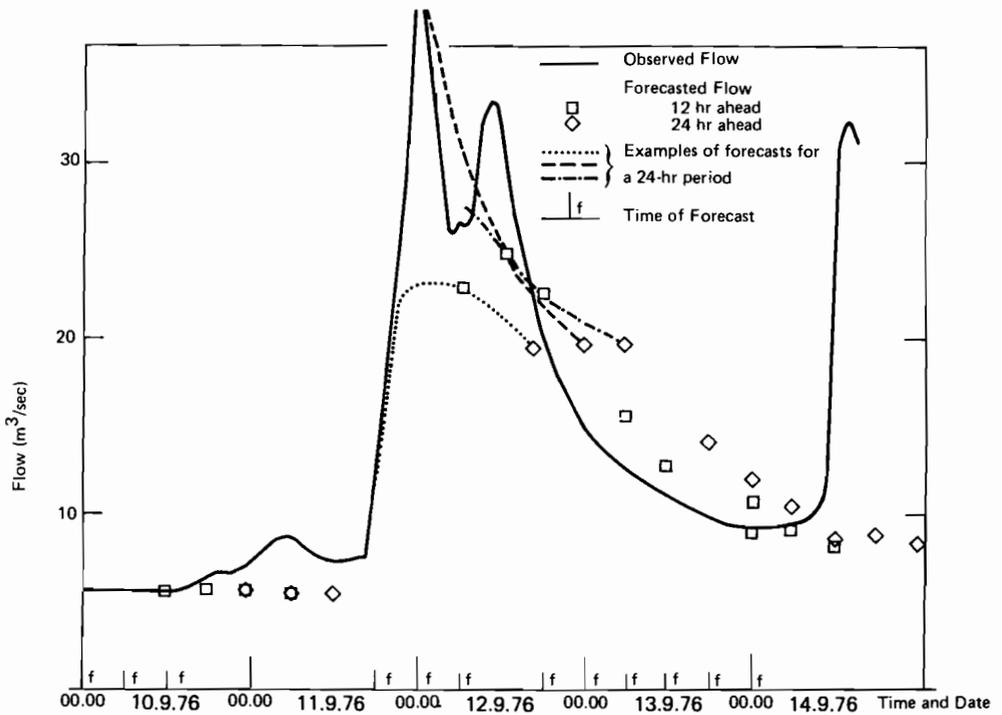
Fig. 16.8 Specimen of hydrograph and forecasts of the Dee at Corwen for September 10 to 13, 1976 (from the Dee Weather Radar and Real-Time Hydrological Forecasting Project Report 1977).
