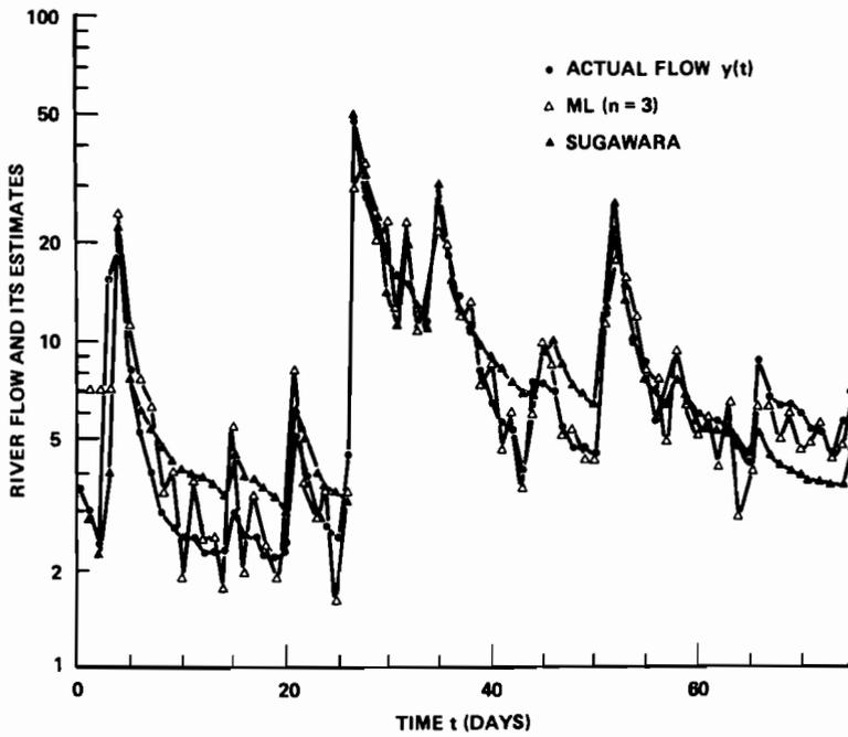
Fig. 4.6 Actual river flow and estimates with the linear and tank models.
