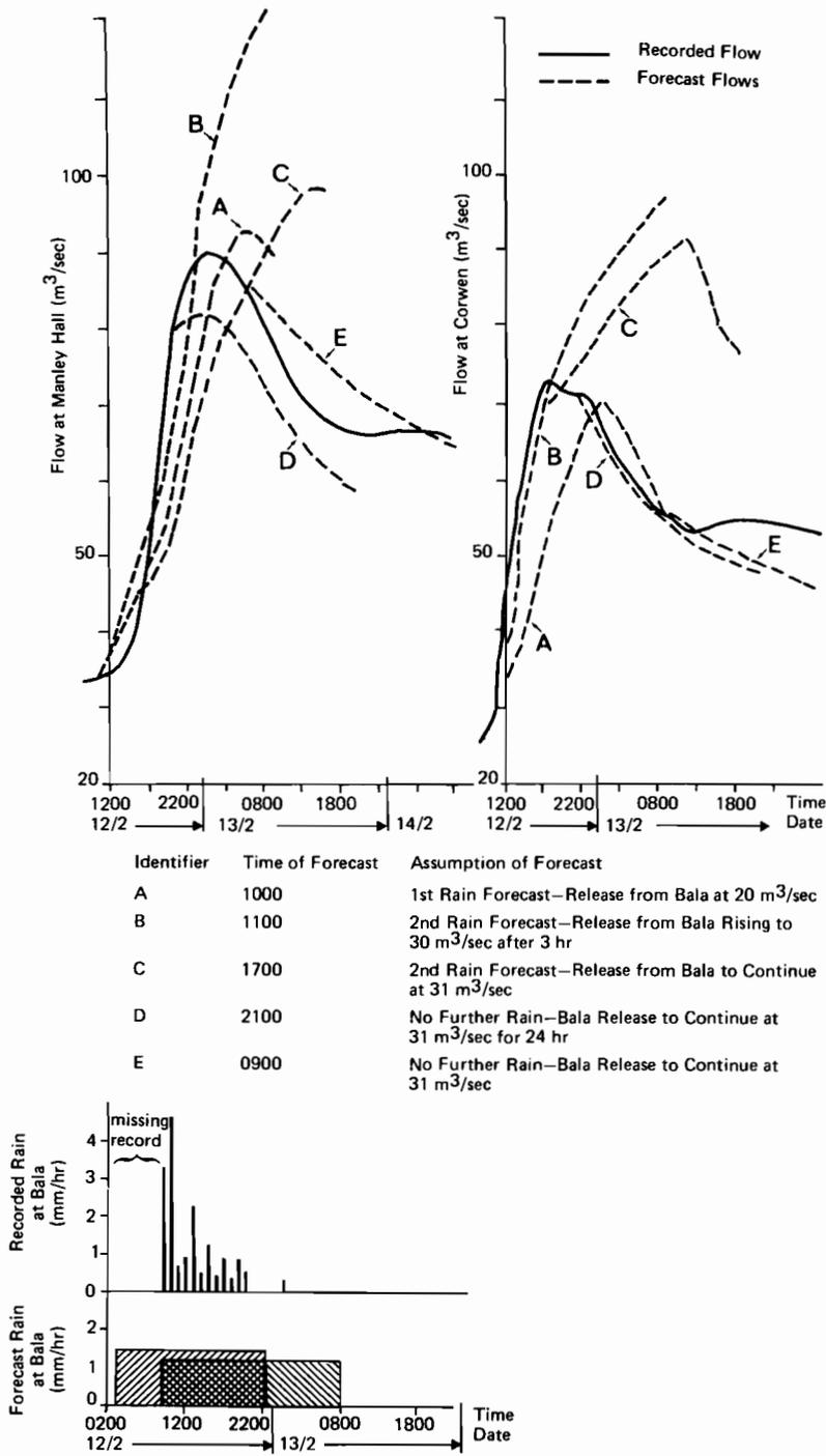
Fig. 16.6 Comparison of forecast hydrographs on basis of different rain forecasts (from Water Research Centre, Medmenham, England).
