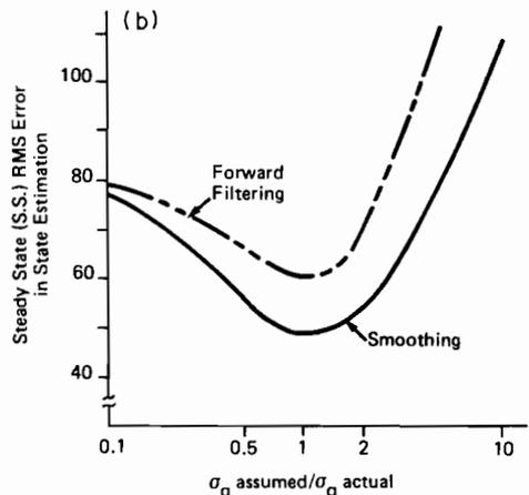
Fig. 2.4b Effect of errors in process noise variance on steady-state RMS error in state estimation.  $\sigma_q$  = process noise standard deviation. (from Mehra 1968).
