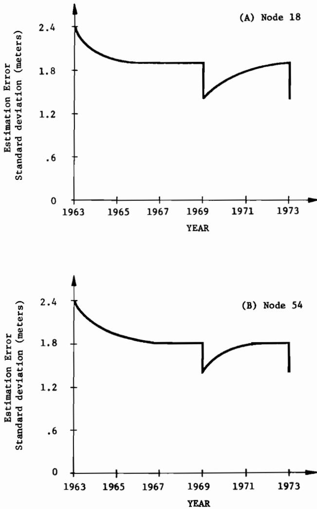
Fig. 7.4 Standard deviations of filtered water table elevation error.
