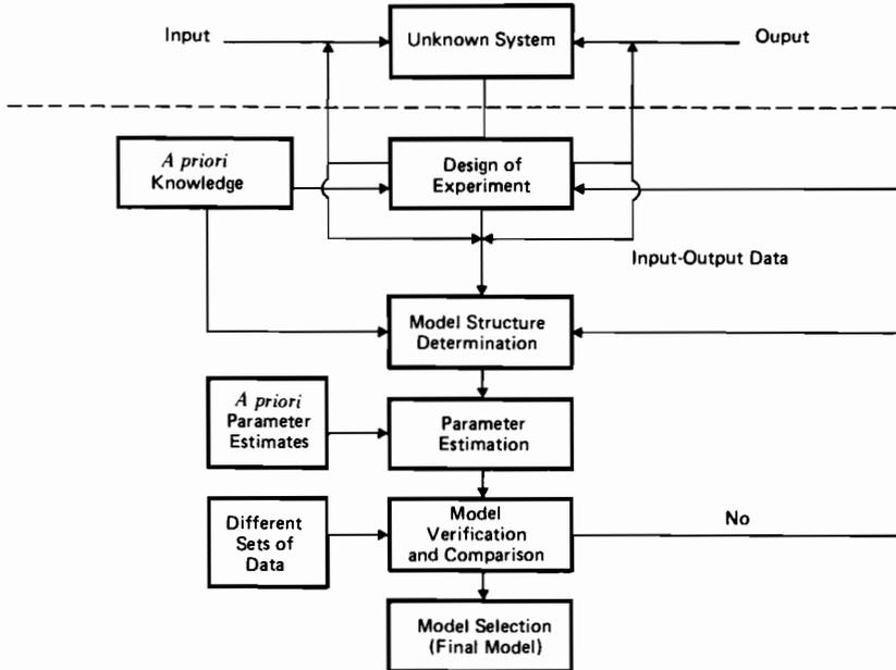
Fig. 2.1 Steps in system modeling and identification (from Mehra and Lainiotis, 1976).
