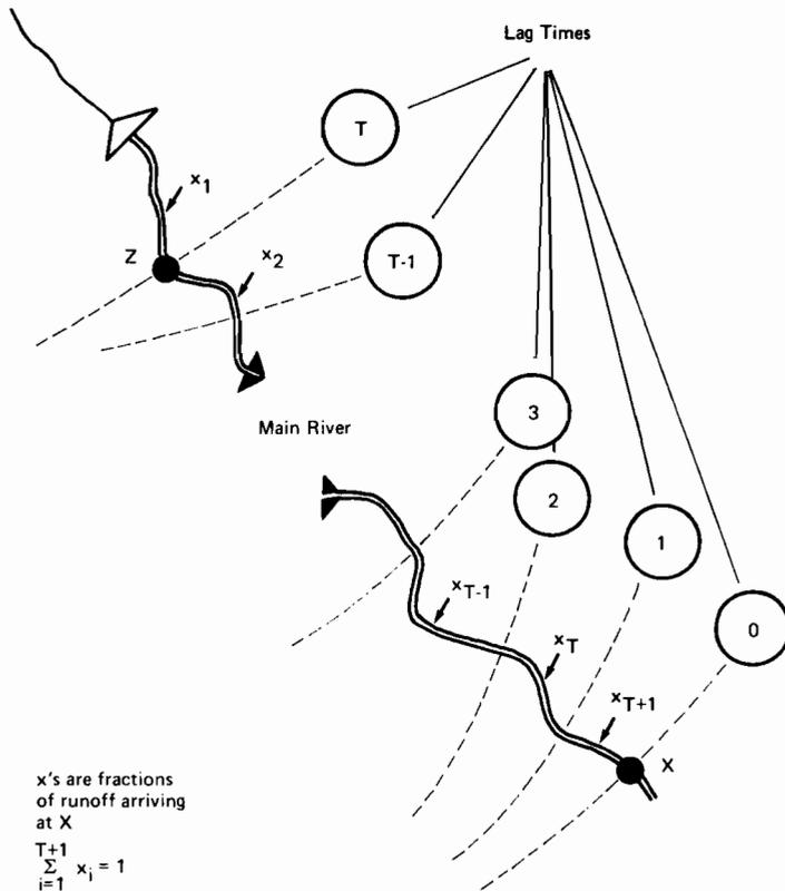
Fig. 16.4 Sketch of river receiving regulated releases at Z with time segments of travel to control point X (from Water Research Centre, Medmenham, England).
