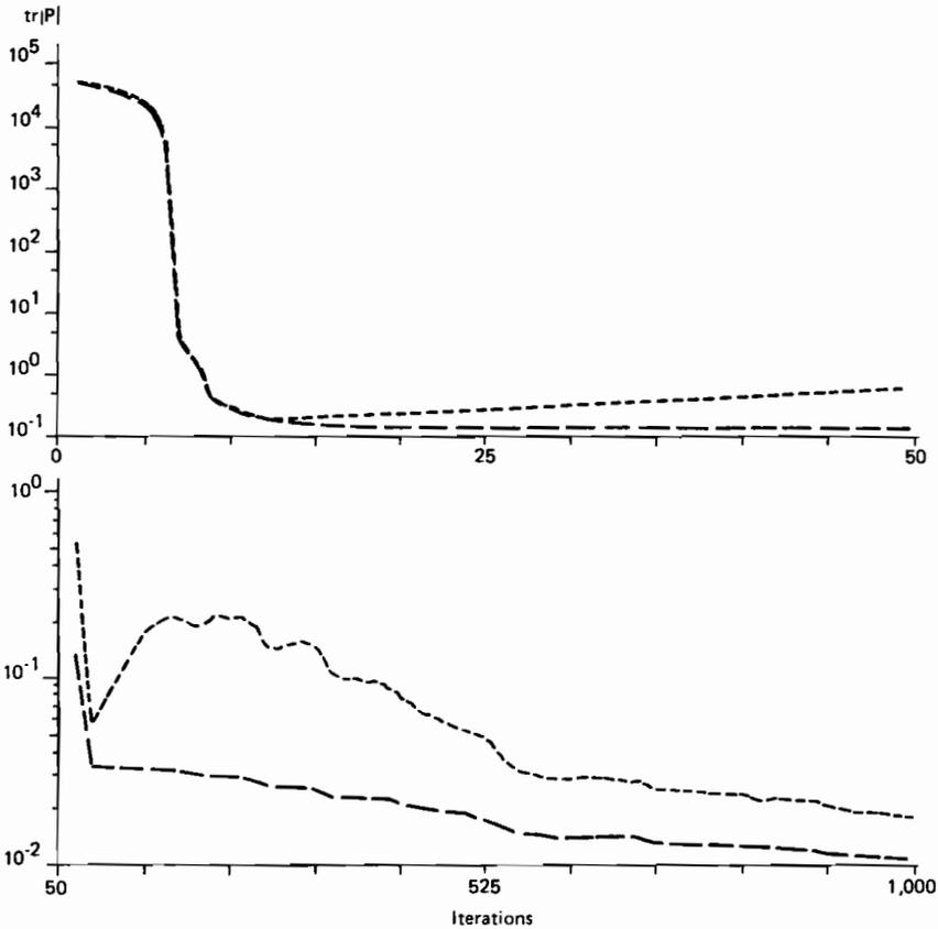
Fig. 9.2 Variation of  $\text{tr}|P|$  over 1,000 iterations with  $P(0) = I \times 10^4$ . - - - -  $\alpha_0 = 0.99, \alpha(0) = 0.95$ ;
