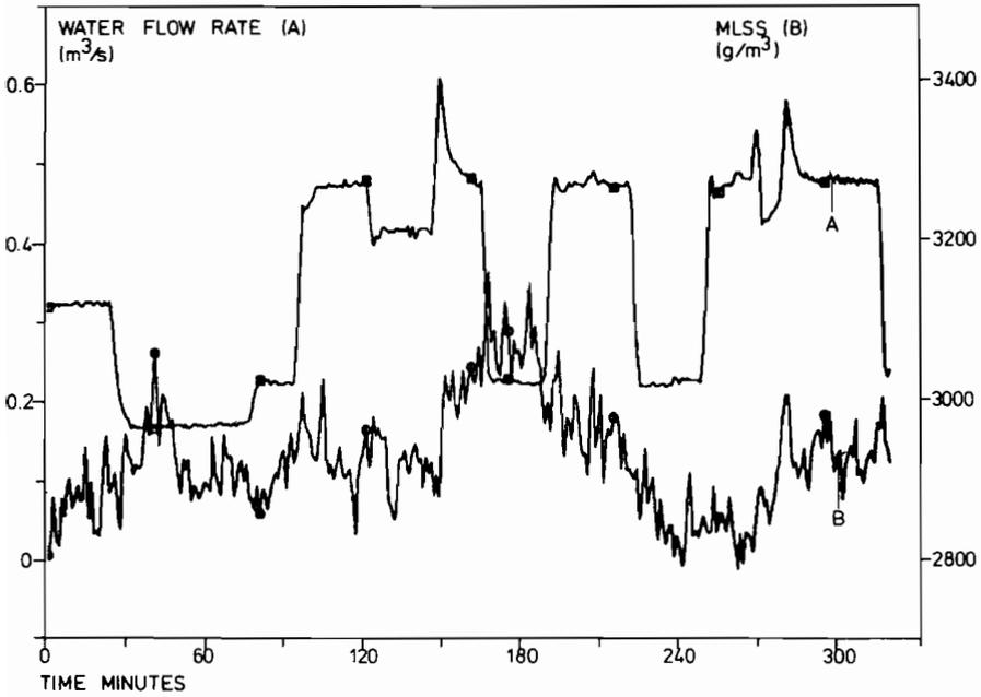
Fig. 6.4 Disturbance signals of a hydraulic experiment in the Käppala wastewater treatment plant. The water flow rate has been manipulated, causing the mixed liquor suspended solids concentration (MLSS) to vary.
