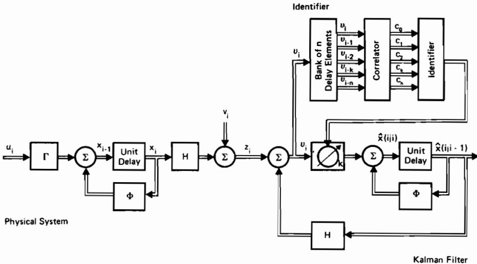
Fig. 2.3 An adaptive Kalman filter (from Mehra 1970).
