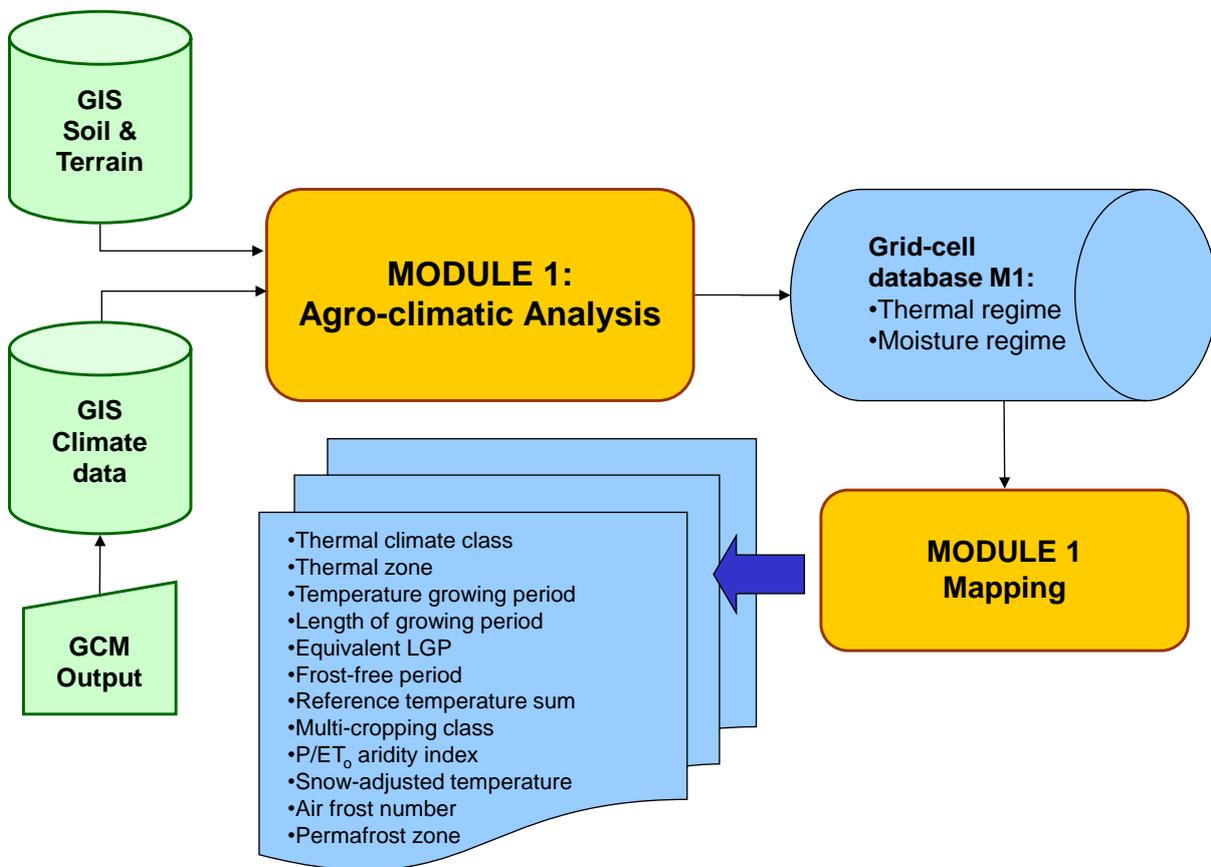
Figure 3-1. Information flow in Module 1 of the AEZ model framework
