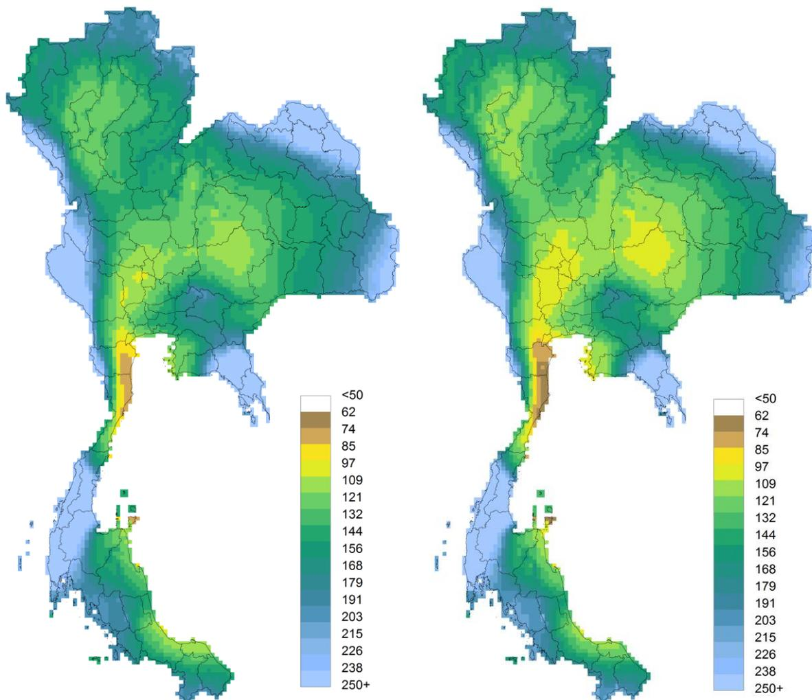
**Figure 9-1. Apr-Sep  $P/ET_0$  ratio for period 1981-2010 and ensemble mean of RCP6.0 in 2041-2070**
