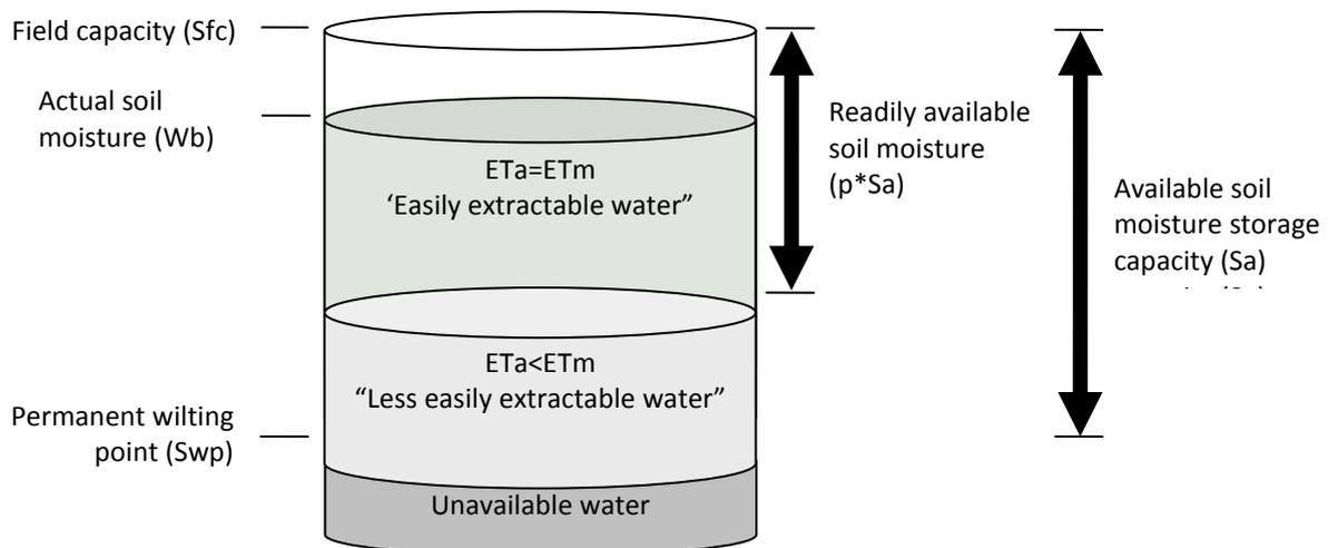
Figure 3-2. Schematic representation of water balance calculations
