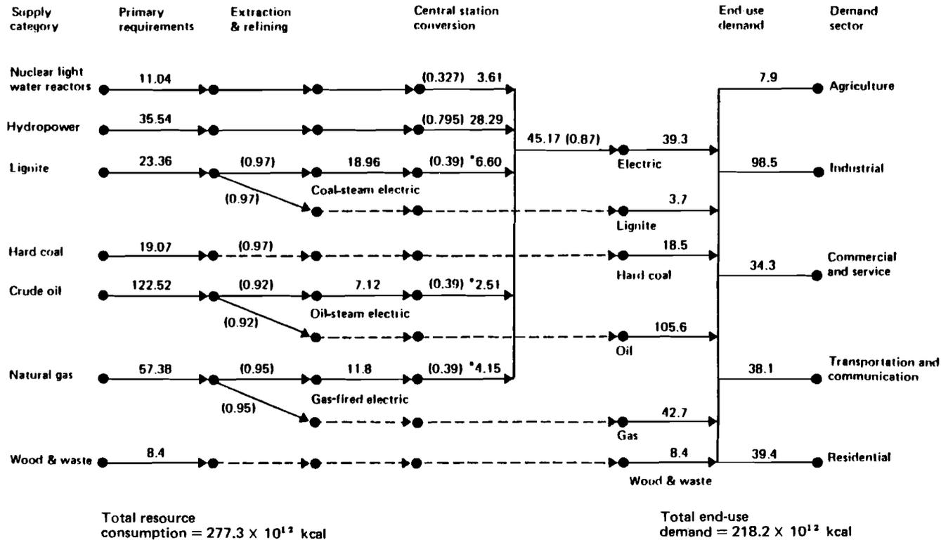
FIGURE 37 A simplified flow diagram of the Austrian reference energy system: Scenario S1, 1990. Energy flows are indicated in  $10^{12}$  kcal. Conversion efficiencies are in parentheses. The 0.39 efficiency for central station conversion of lignite, crude oil, and natural gas refers only to power plants and to combined cycle plants.
