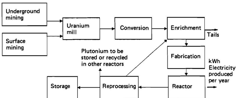
FIGURE 34 The reference system for nuclear power.
