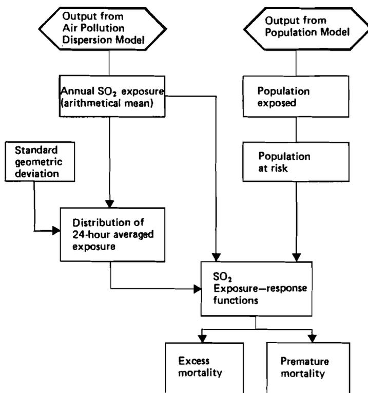
FIGURE 46 Flow of calculations in the SO<sub>2</sub> Health Impact Model.
