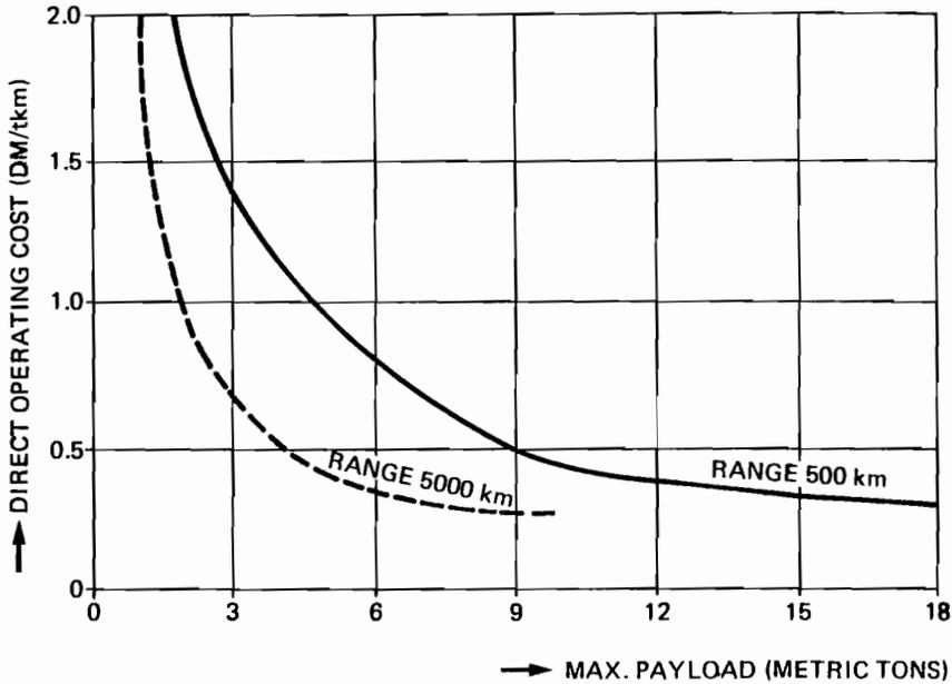
FIGURE 3.2 Direct operating cost as a function of the design payload of transport aircraft.
