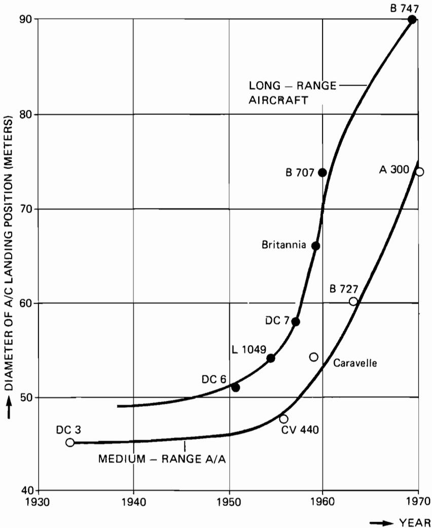
FIGURE 3.6 Area needed for aircraft in landing position on the airfield (safety distance included).
