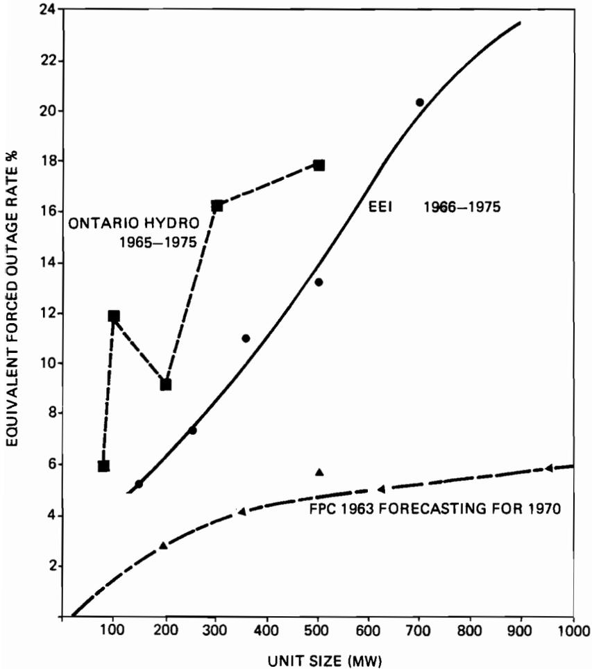
FIGURE 7.1 Equivalent forced outage rate versus unit size for fossil units.
