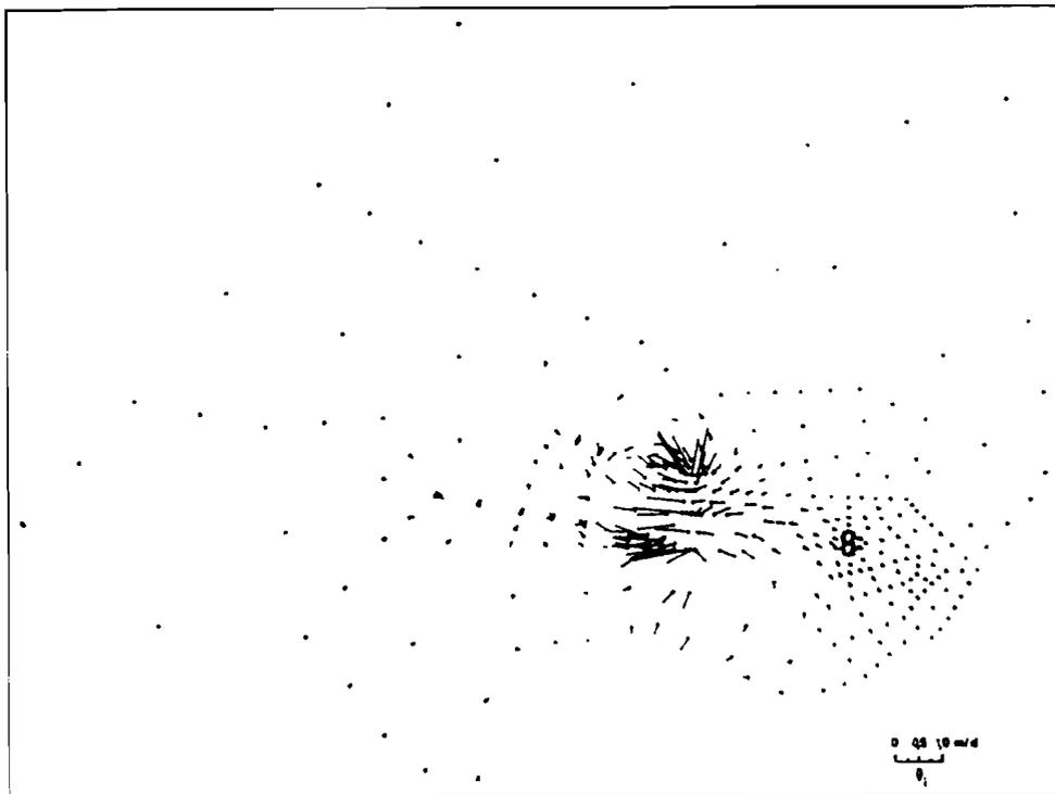
Figure 11. Computed velocity field for  $t \geq 1983$  ( $\hat{v}_i = \bar{q}_i / Mn$ ).
