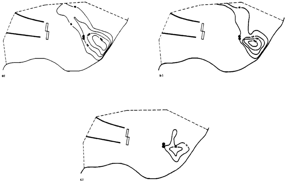
Figure 17. Predicted degradation of contaminant plume by applying two wells (total  $2000\text{m}^3/\text{day}$ ) starting 1984, under unceasing operating the hydraulic barrier, and with uncontaminated infiltrate ( $C_1^R = 0$  along  $efghi$ ); a) 1985, b) 1995, c) 2015
