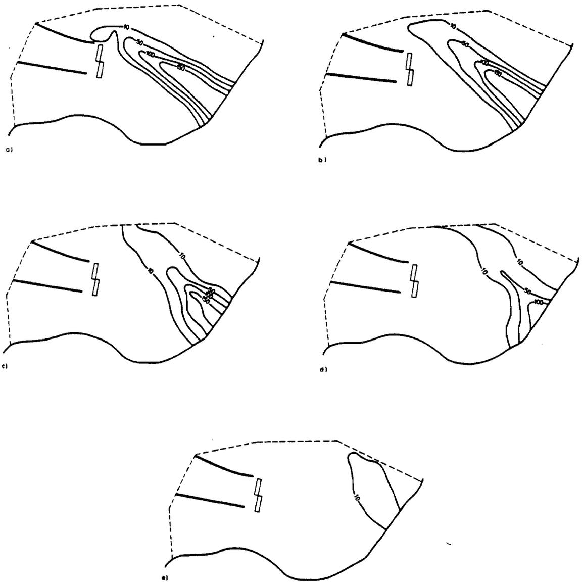
Figure 12. Computed contaminant distribution (cut-out of study area) under permanent operating of phenol barrier for prognosis period in a) 1978, b) 1980, c) 1986, d) 1993, e) 2010.
