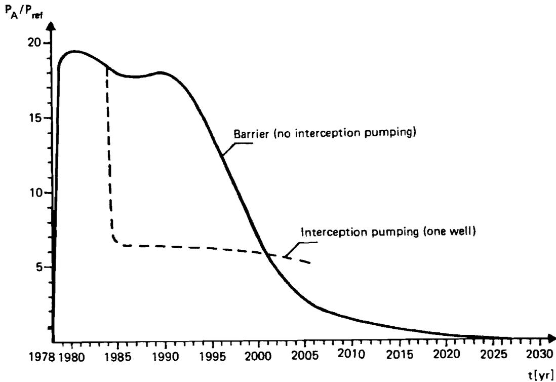
Figure 13. Computed history of normalized contaminant effluent  $P_A / P_{ref}$  entering the surface waters under permanent operating of hydraulic barrier.
