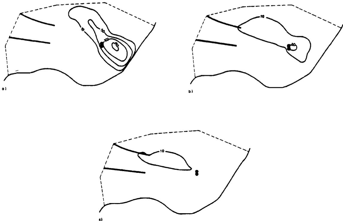
Figure 19. Predicted degradation of contaminant plume by applying two wells (total  $2000\text{m}^3/\text{day}$ ) with the beginning of the year 1984, under ceasing the hydraulic barrier, and with uncontaminated infiltrate ( $C_1^R = 0$  along  $efghi$ ); a) 1985, b) 1990, c) 1995.
