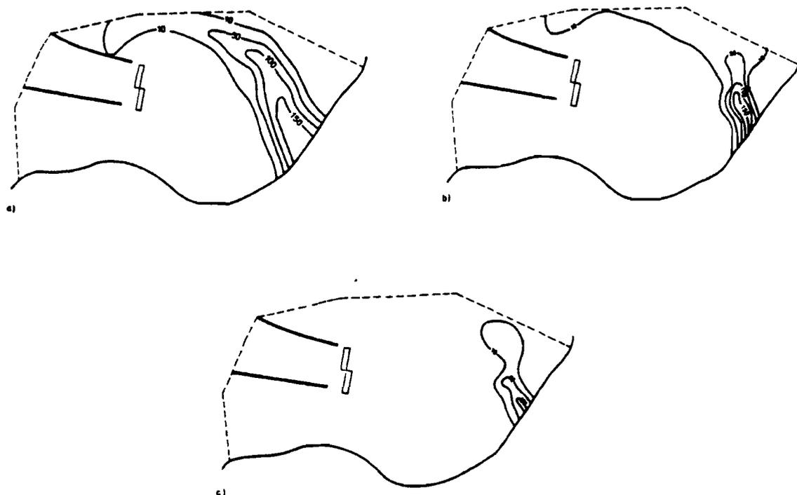
Figure 14. Hypothetical movement of contaminant plume at four-times higher water supply under barrier operating (cut-out of study area) for a) 1988, b) 2027, c) 2060.
