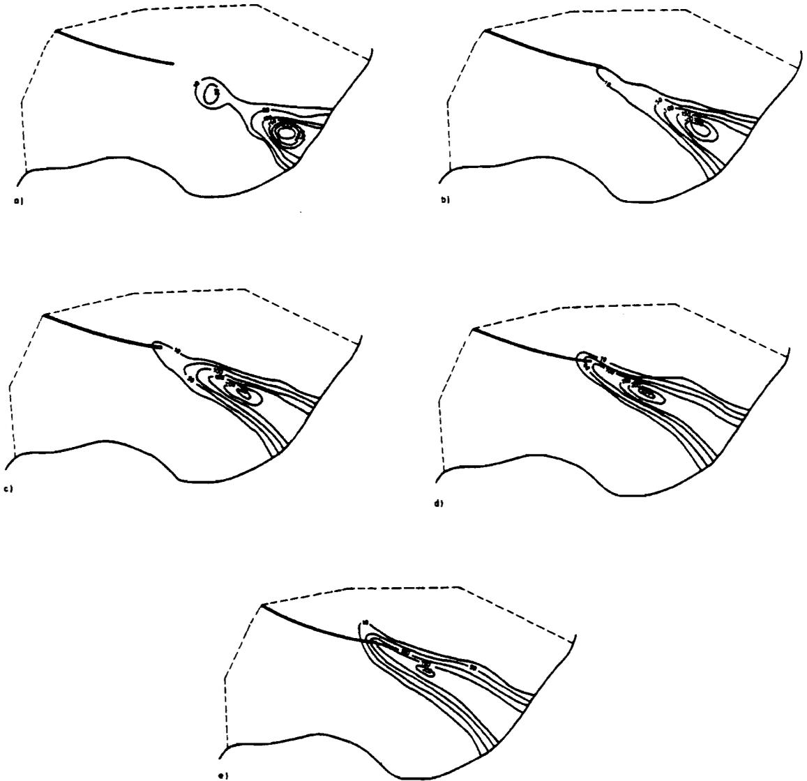
Figure 9. Computed contaminant distribution (cut-out of study area) at a) 1968 (initial field), b) 1970, c) 1972, d) 1974, e) 1977
