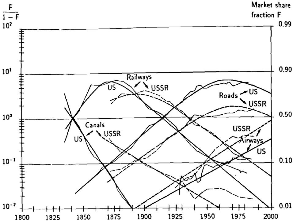
**Figure 7.** Infrastructure substitution in the USA and the USSR, shares in length, logit transformation.
