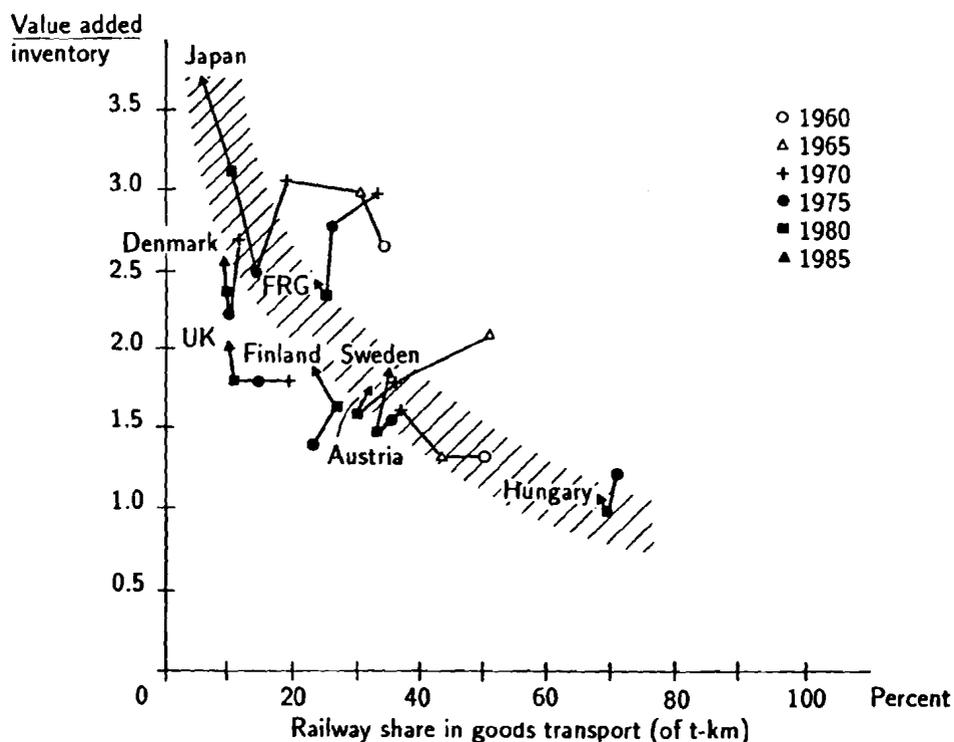
**Figure 21.** Ratio of value added over inventories in the manufacturing sector of selected countries versus railway share in goods transportation 1960–1985. Source: UN, Yearbook of Industrial Statistics, 1977 and 1987; IRF, World Road Statistics and National Transport Statistics, 1970 to 1987.
