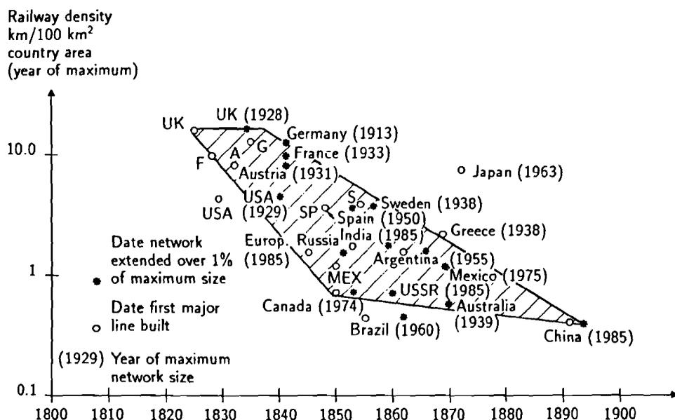
**Figure 27.** Spatial railway density envelope versus network construction start-up date, in km of railway network at peak year (1985, for networks still expanding) per 100 km<sup>2</sup> of the country. Source: Grübler (1990).
