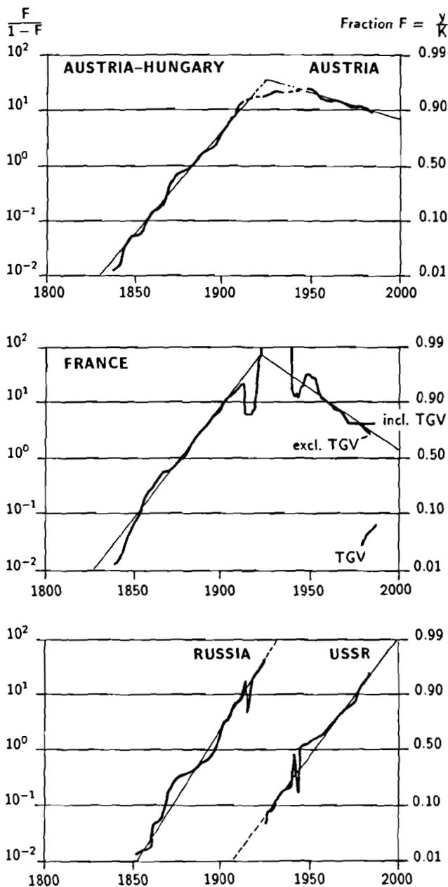
**Figure 25.** Rise and fall of railway networks in Austria-Hungary (Austria after 1919), France, and the first and second phase of railway construction in Russia and the USSR, in fractional share of estimated saturation level, logit transformation. For model parameters see *Table 1*. Source: Adapted from Grübler (1990).
