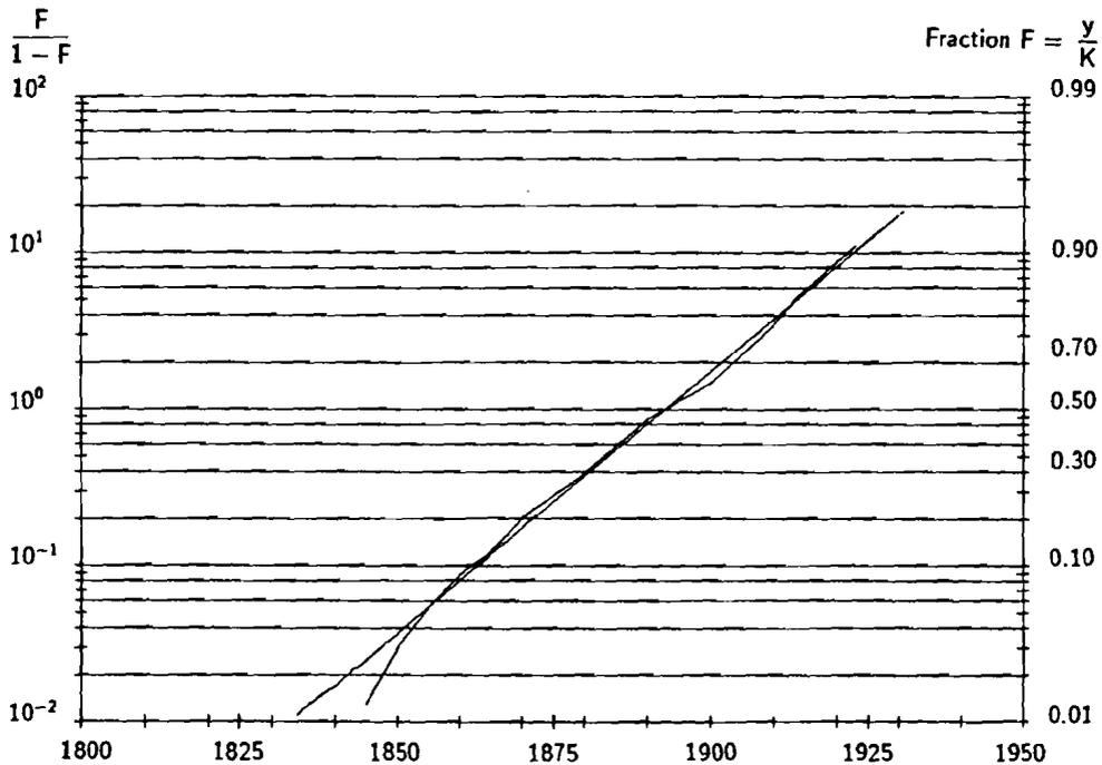
**Figure 23.** Growth of the world's railway network ( $K$  1.323  $10^6$  km,  $t_0$  1983,  $\Delta t$  57 years). The length of the network has remained constant at a level of 1.3 million km since the 1930s. Source: Grübler (1990).
