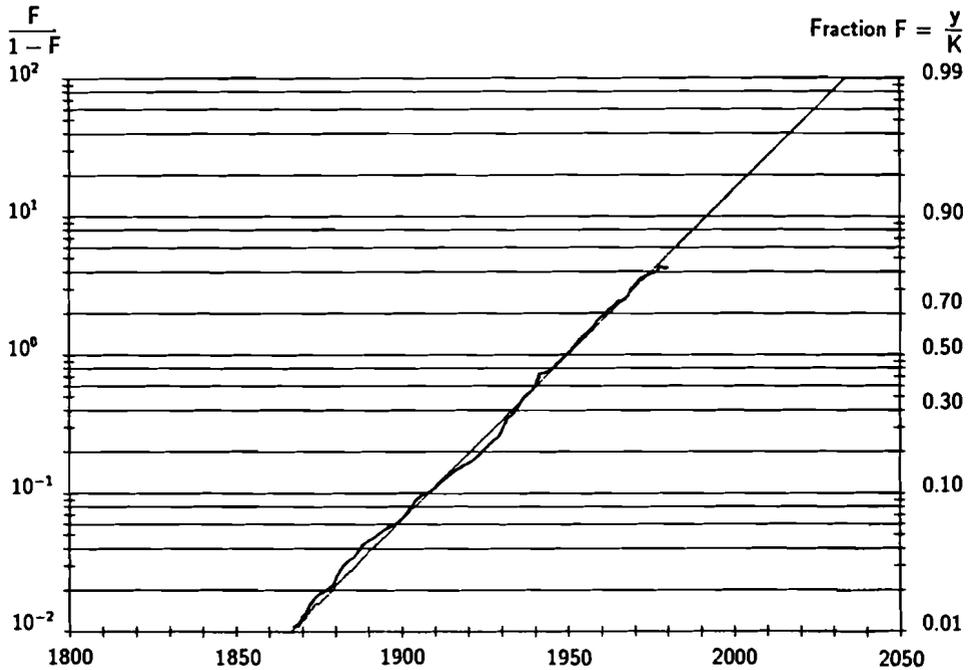
**Figure 3.** Growth in length of all transport infrastructures in the USA, in fractional share of ultimate saturation level (4.7 million miles or 7.6 million km), logit transformation. Source: Grübler (1990).
