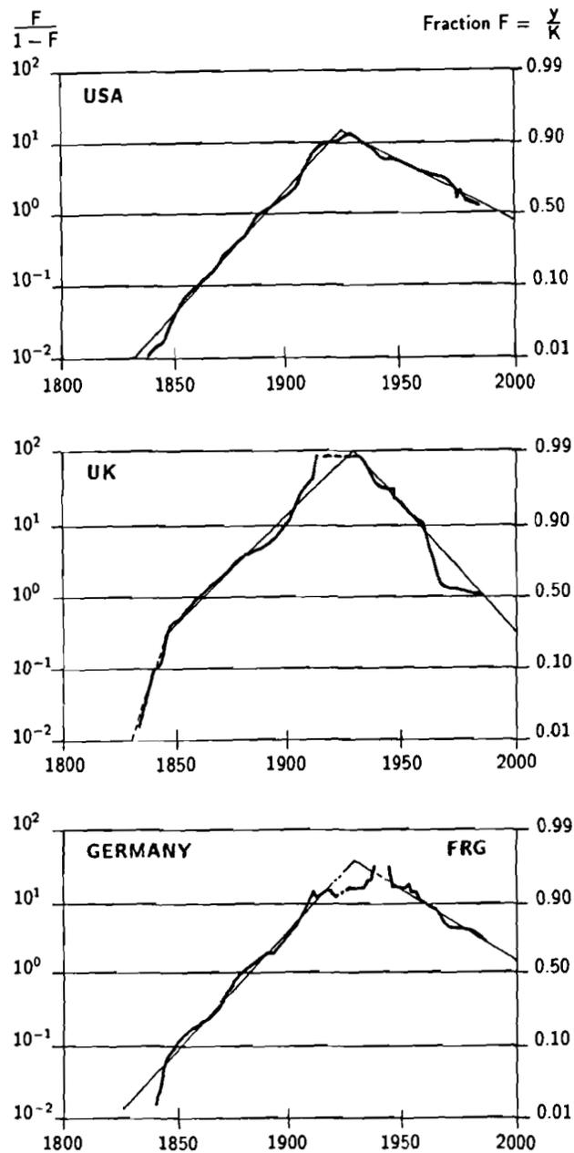
**Figure 24.** Rise and fall of railway networks in the USA, the UK, and Germany (FRG after 1945), in fractional share of estimated saturation level, logit transformation. For model parameters see *Table 1*. Source: Adapted from Grübler (1990).
