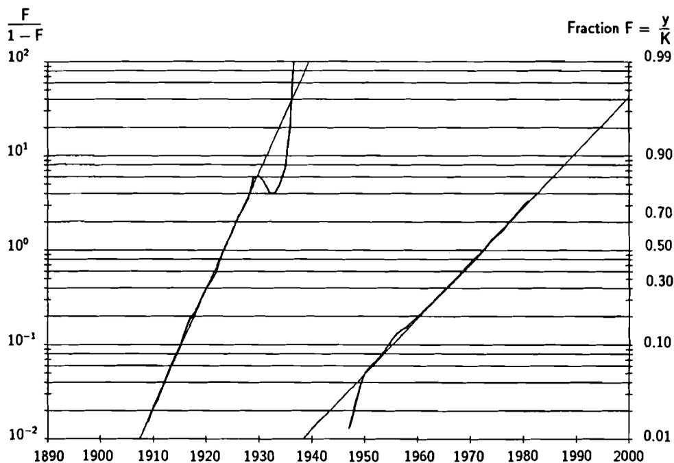
**Figure 29.** Two diffusion pulses in the expansion of the number of passenger cars registered worldwide. [First pulse:  $K$  35 million cars,  $t_0$  1923,  $\Delta t$  15 years; second pulse  $K$  464 million cars (including intercept),  $t_0$  1974,  $\Delta t$  36 years.] Source: MVMA (1987), for period prior to 1930 own estimates.
