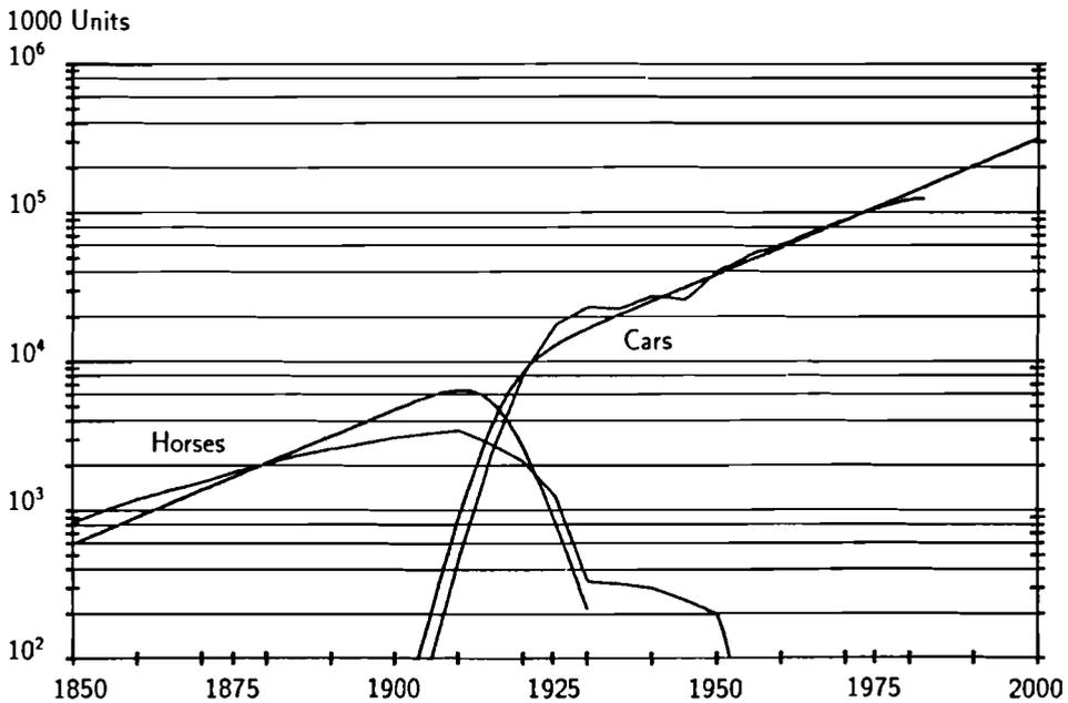
**Figure 30.** Number of draught animals (horses and mules) used for transport and number of cars in the USA, empirical data and model estimates resulting from logistic substitution model, in thousands. Source: Nakićenović (1986 and 1988).
