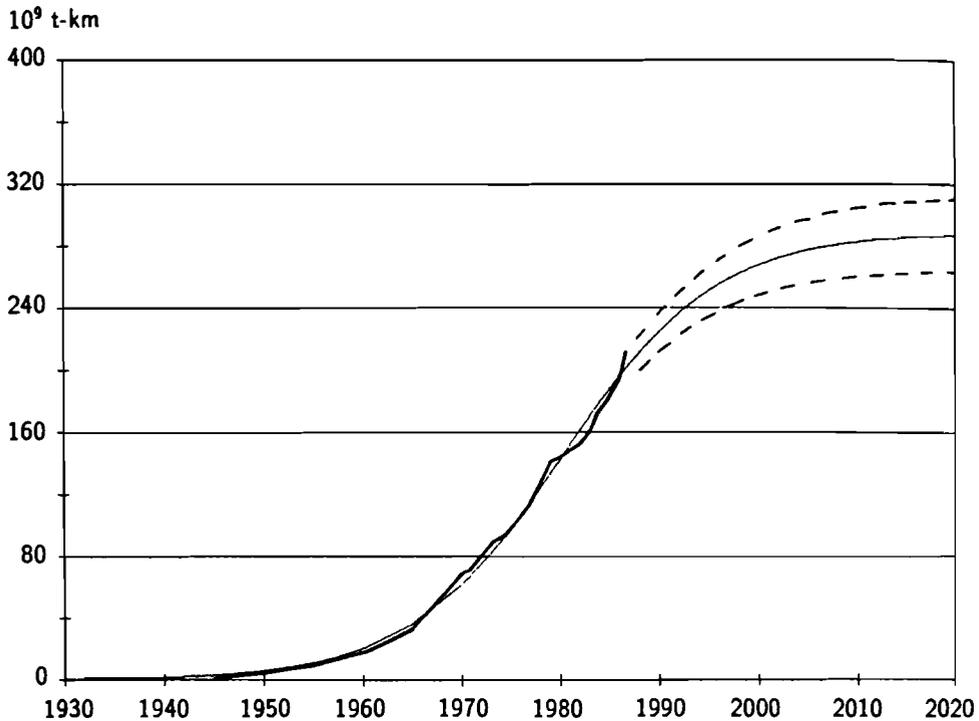
**Figure 33.** Volume of air transport worldwide (including centrally planned economies) passenger, cargo, and mail, in billion ton-km transported, linear scale. Diffusion model parameters:  $K$  289.2  $10^9$  t-km,  $t_0$  1980,  $\Delta t$  34.5 years, and uncertainty bands.
