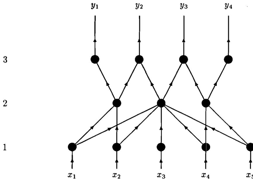
Figure 1: A multi-layered perceptron with 3 layers of nodes; the  $x_i$  are the inputs of the perceptron and the  $y_j$  the outputs.
