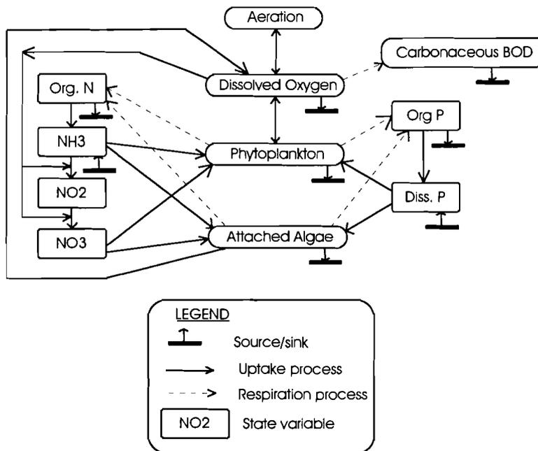
Figure 3: Water quality interactions accounted for in RMA4q v2.
