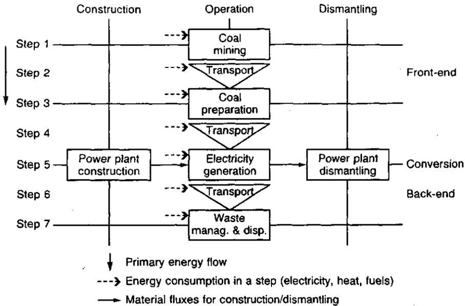
FIG. 3. Schematic representation of a coal fuel chain [3].
