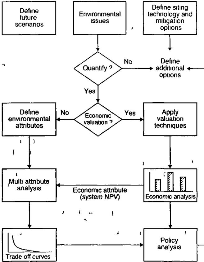
FIG 4 General methodology for environmental analysis of power systems
