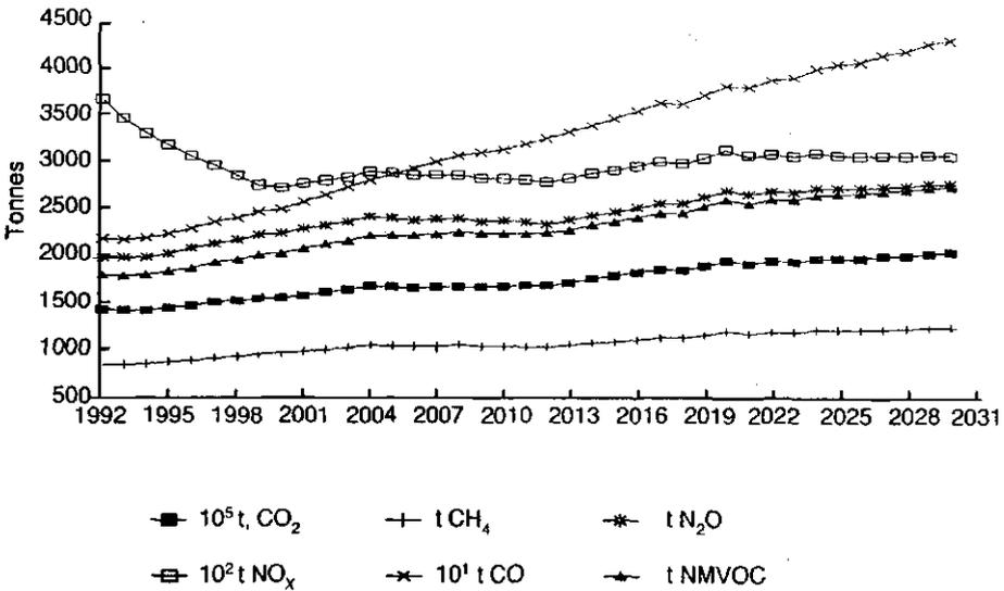
FIG. 7. Greenhouse gas emissions from electricity generation — nuclear case.
