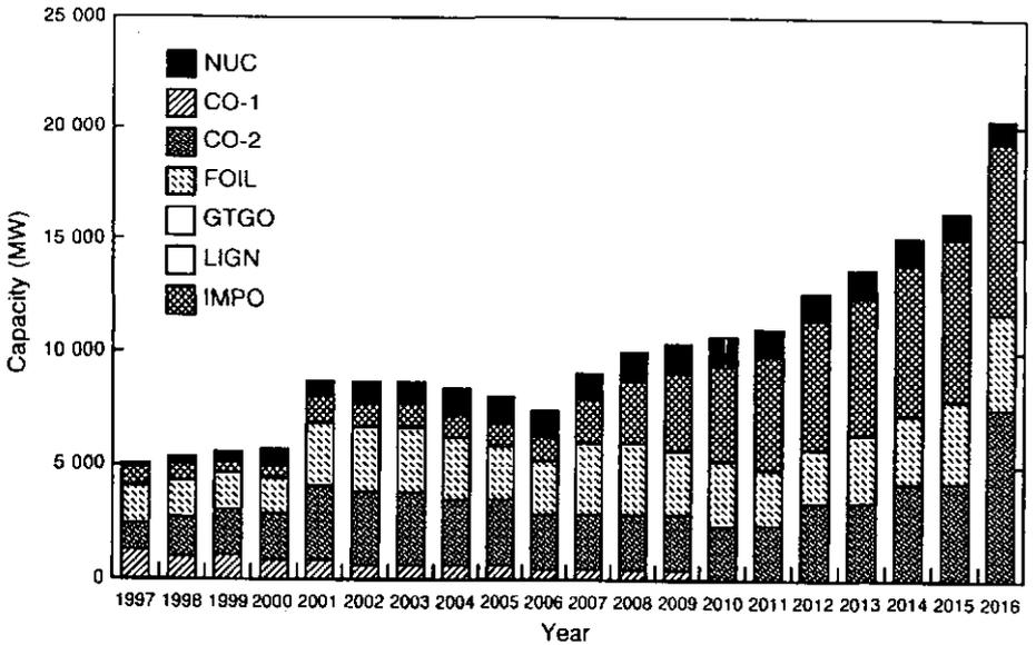
FIG. 22. Total installed capacity in a thermal system — screening mode.
