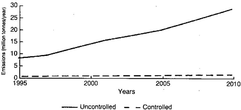
FIG. 5. Results for particulate emissions for the reference case.
