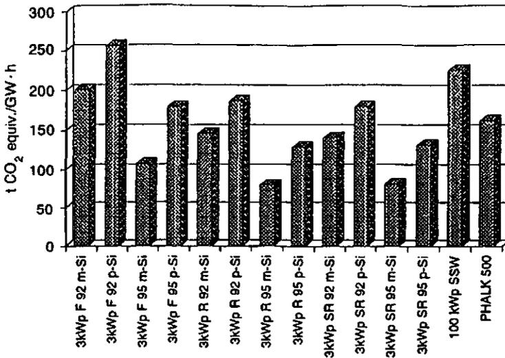
FIG. 2. LCA based GHG emissions from present photovoltaic systems [9] (warming potentials according to IPCC 1992).
