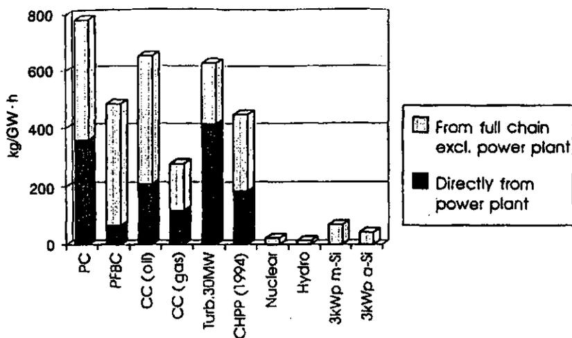
FIG. 4. LCA based NO<sub>x</sub> emissions from advanced systems [7] (see Fig. 3).
