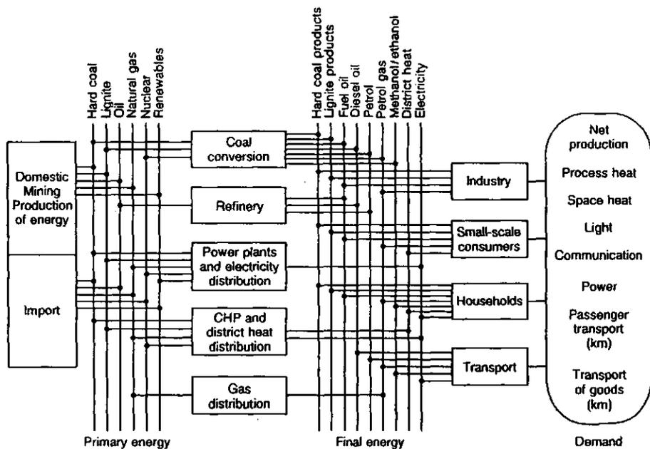
FIG. 1. Structure of the energy system model.
