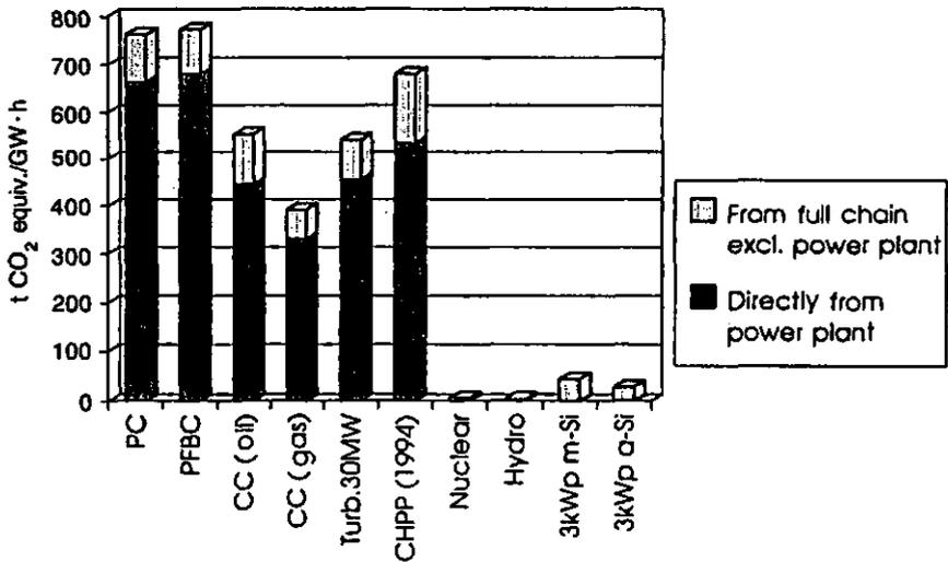
FIG. 3. LCA based GHG emissions from advanced systems [7] (warming potentials according to IPCC 1994).
