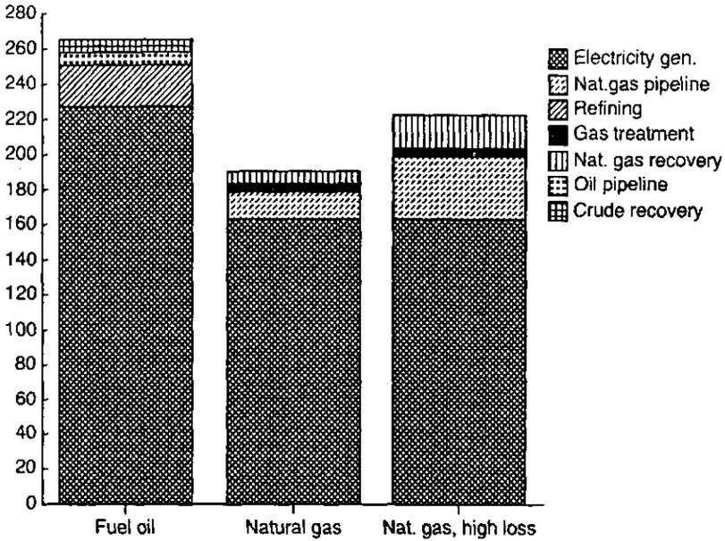
FIG. 3. Venezuela electricity fuel chains: greenhouse gas emissions by stage (kg CO<sub>2</sub> equivalent per gigajoule final energy; IPCC 100 year integration, see Ref. [15]).
