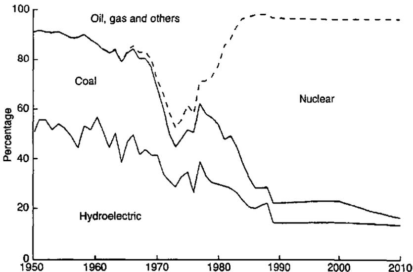
FIG. 1. Structure of electricity production in France with nuclear power.
