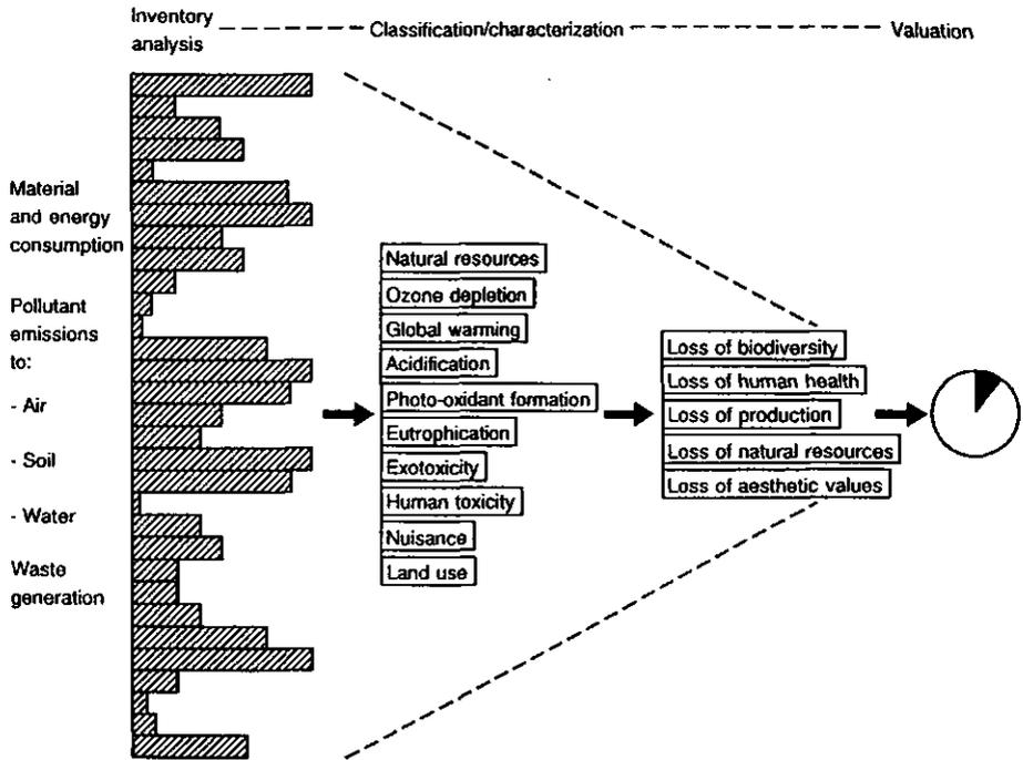
FIG. 12. Relationship between inventory analysis and components of impact assessment.
