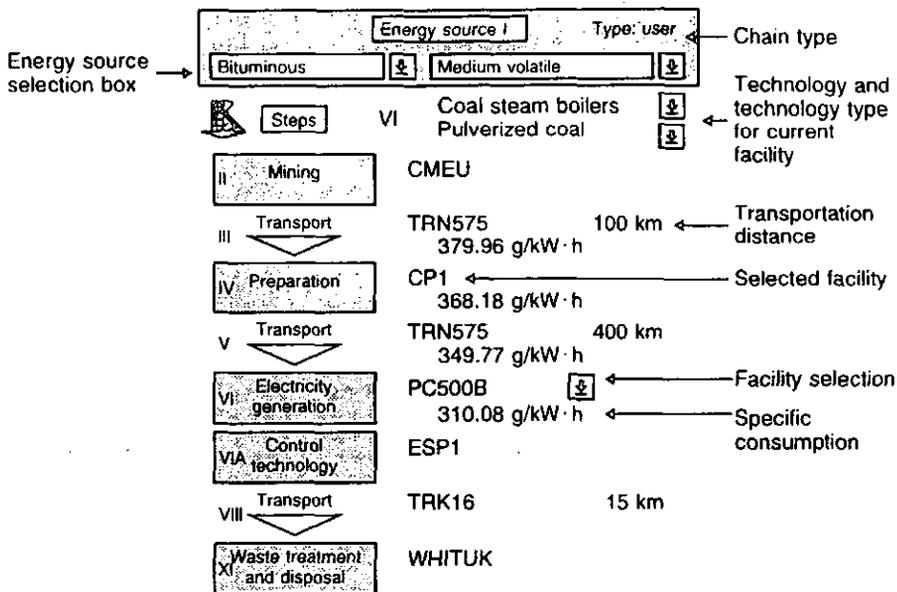
FIG. 13. Modular representation of the coal chain.
