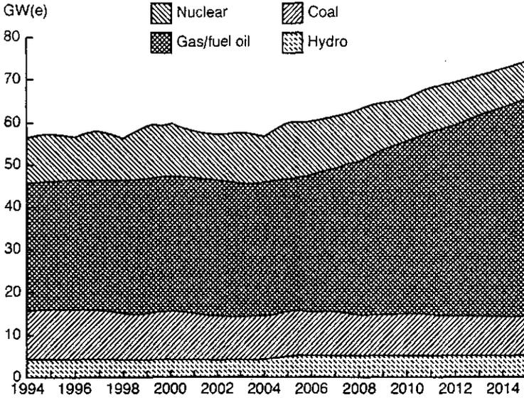
FIG. 5. Structure of the optimal capacity expansion plan.
