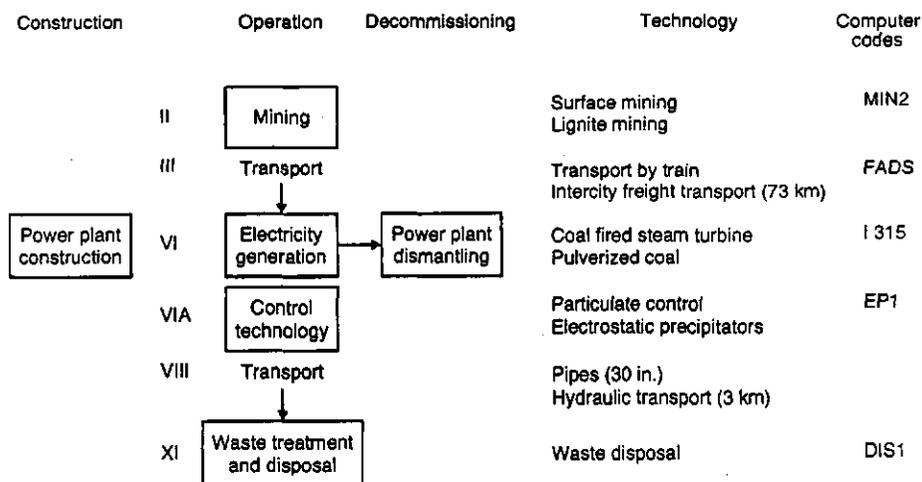
FIG. 1. Solid fuel: lignite chain.
