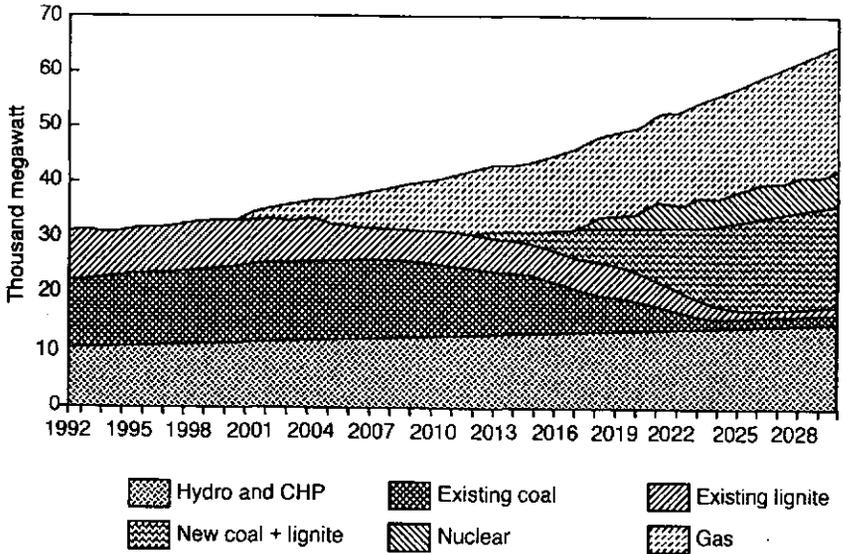
FIG. 5. Power system capacity mix — nuclear case.
