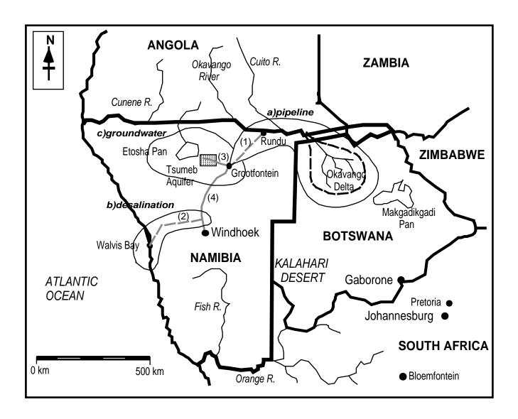
Figure 1. Map showing the 3 water supply alternatives for Windhoek that were evaluated with emergy analysis: (1) Kavango River pipeline; (2) pipe for transporting desalinated water; (3) groundwater pipeline; (4) existing canal; (——) approximate boundary of the Okavango Delta; (——) relative and approximate influence area for each water supply system.
