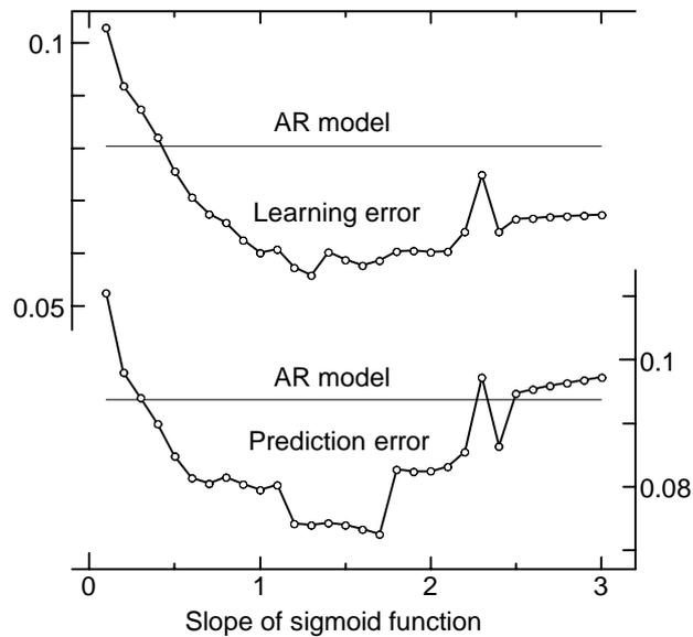
**Figure 10.5.** Learning results for the slope of the sigmoid function.
