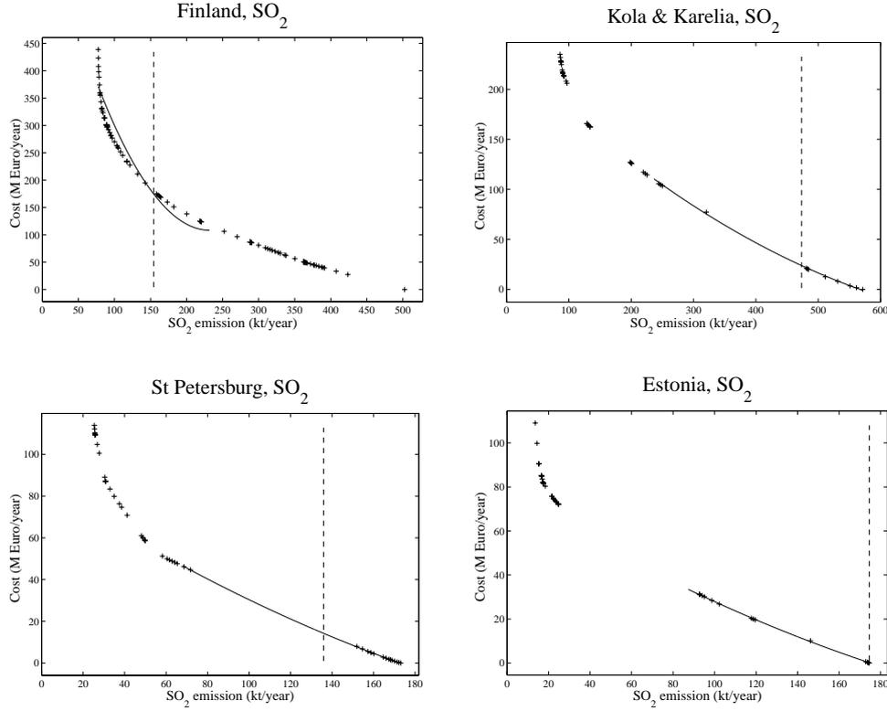
**Figure 5.1.** The original data (+) and the estimated yearly abatement costs (solid line) for SO<sub>2</sub> in different regions. The status-quo emission level is indicated by a dashed vertical line.
