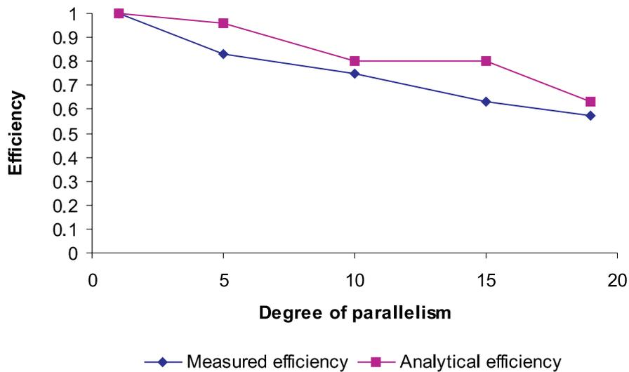
**Figure 17.4.** Efficiency of the distributed polytope optimization algorithm with an increasing degree of parallelism for the solution of the facility optimization problem.
