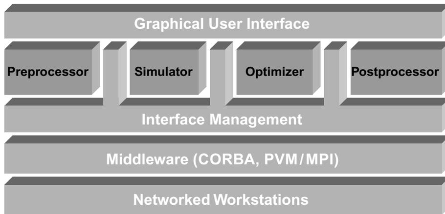
**Figure 17.1.** The software architecture for a distributed problem solving environment with coupled FEM simulation and optimization.
