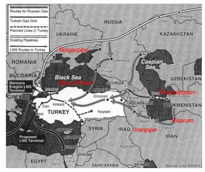
Figure 1. Gas pipeline routes to Turkey (Source: Gas Matters)
