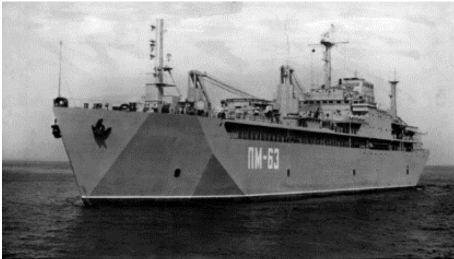
Figure 2-6: Project 2020 ("Malina") Class Floating Workshop (Bellona, 1996)
