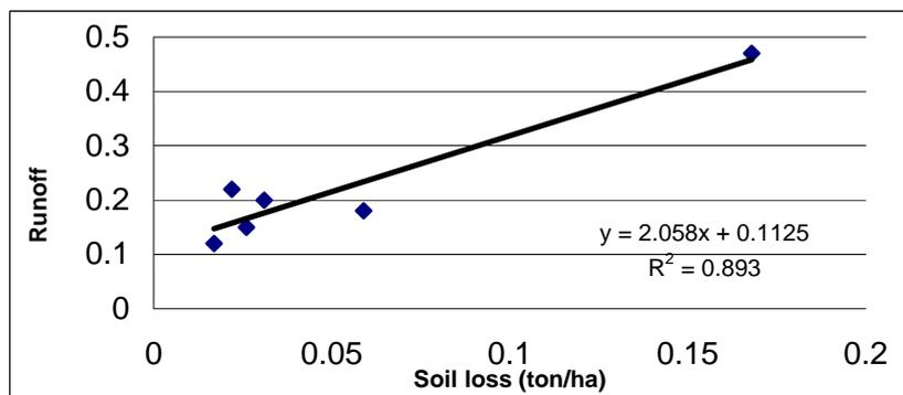
Fig. (9): Relationship between the runoff and soil loss under planting with mulch (1.0 ton/ ha)
