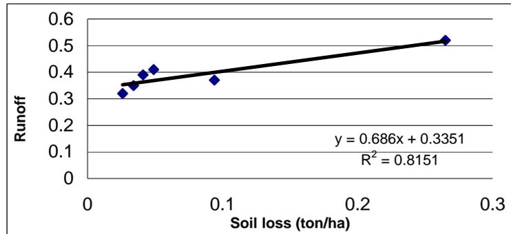
Fig. (8): Relationship between the runoff and soil loss under planting with mulch (0.5 ton/ ha)
