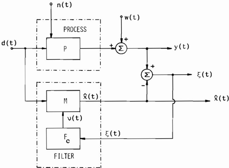
Fig. 11.11 The principal components of process state estimation and filtering;  $n(t)$  and  $w(t)$  are, respectively, system noise and random measurement errors.
