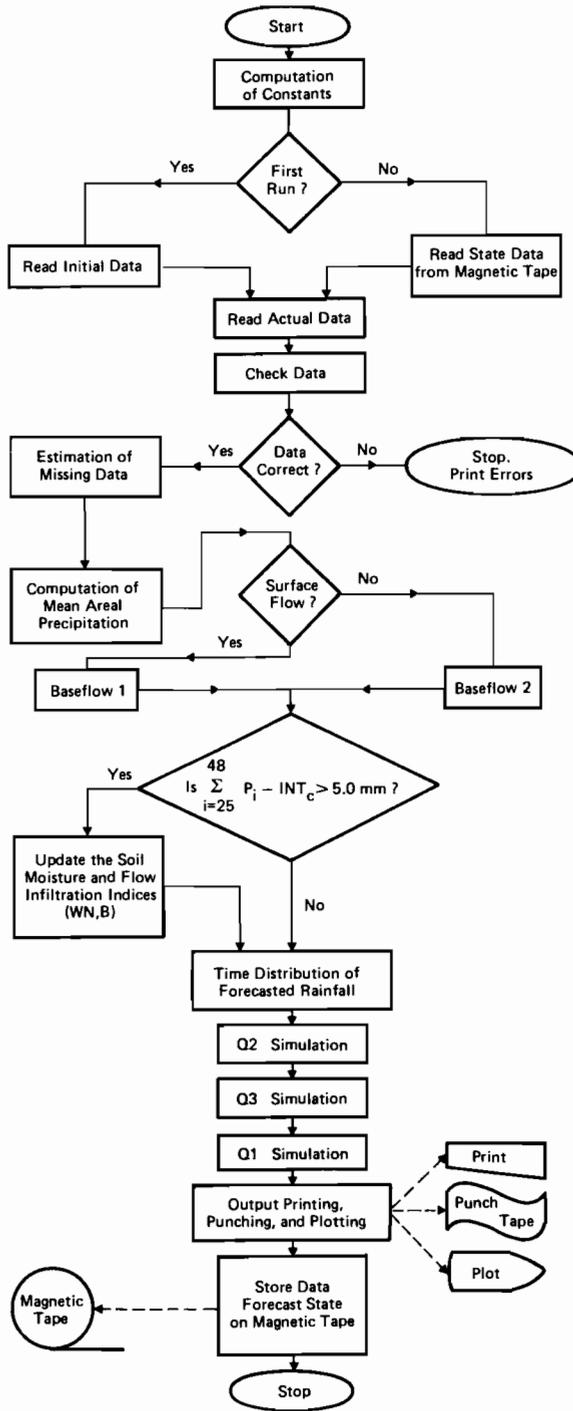
Fig. 17.1 A flow chart of the forecasting model for the Sola and Dunajec Rivers. See the text for explanations of  $P_i$  and  $INT_c$ .
