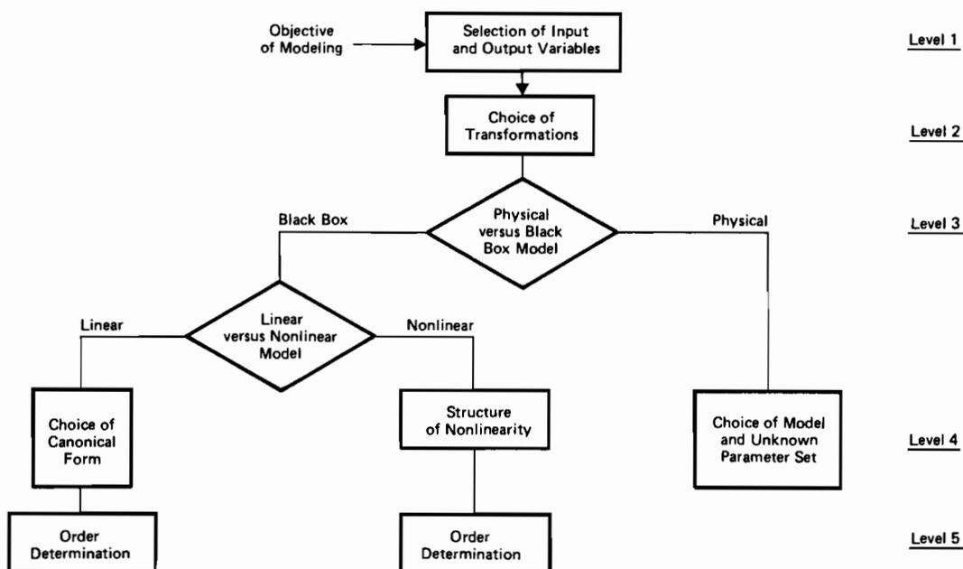
Fig. 2.5 Hierarchical levels in model structure determination.
