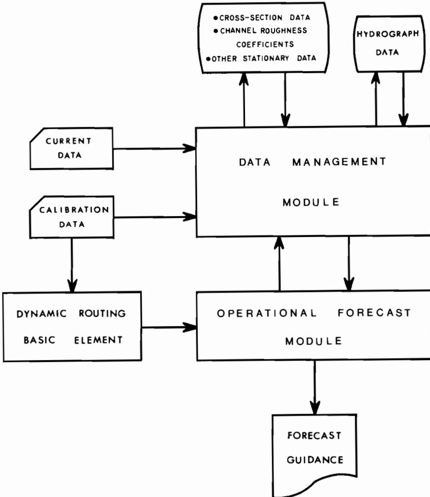
Fig. 18.7 Operational dynamic routing model.
