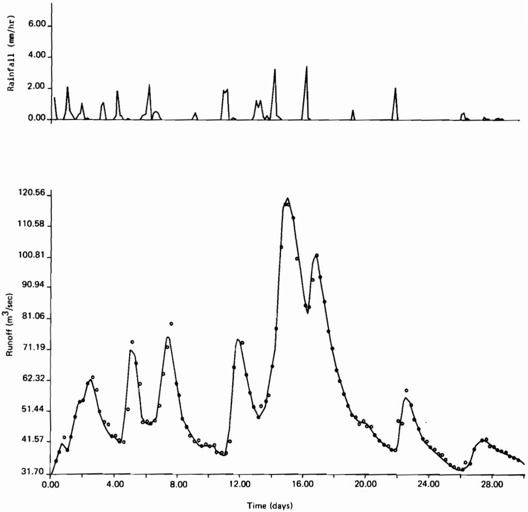
Fig. 9.6 Two-step-ahead self-tuning predictor for Brosna Catchment with  $m = 3$ ,  $n = 2$ ,  $l = 2$  and input delay = 1 (3 hr).
