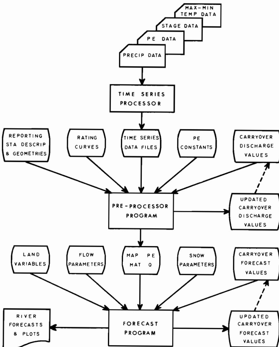
Fig. 18.6 Operational catchment response model. PE stands for potential evapotranspiration, STA for station, and Q for discharge.
