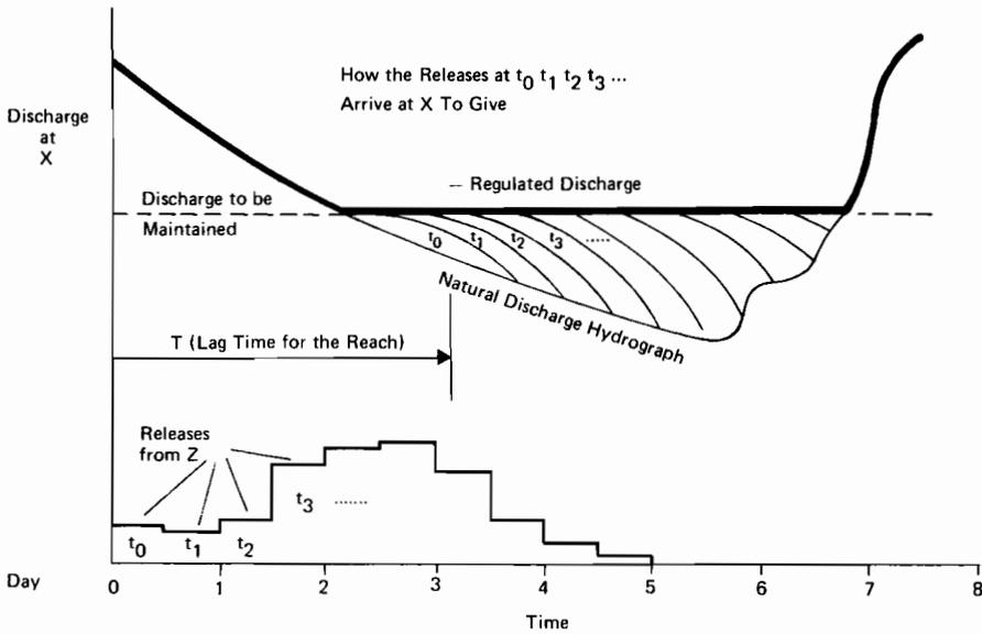
Fig. 16.5 How successive releases of water at Z arrive at X (from Water Research Centre, Medmenham, England).
