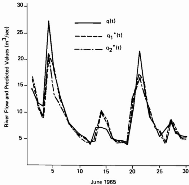
Fig. 10.9 Tracking behavior of predicted values  $q_1^*(t)$  and  $q_2^*(t)$  together with actual flow  $q(t)$ .
