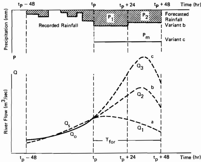
Fig. 17.2 The diagram of the forecasting model principles.  $t_p$  = the initial moment of the forecast period;  $t_p + 48$  = the end of the hydrograph forecast period;  $T_{for}$  = the forecast period;  $Q_s$  = simulated hydrograph;  $Q_o$  = recorded hydrograph; a, b, c, = three variations of the hydrograph forecast corresponding to three precipitation forecasts.
