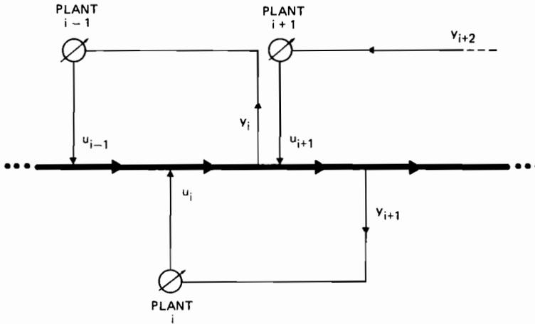
Fig. 14.3 Overlapping control structure along a river (from Rinaldi et al. 1978).
