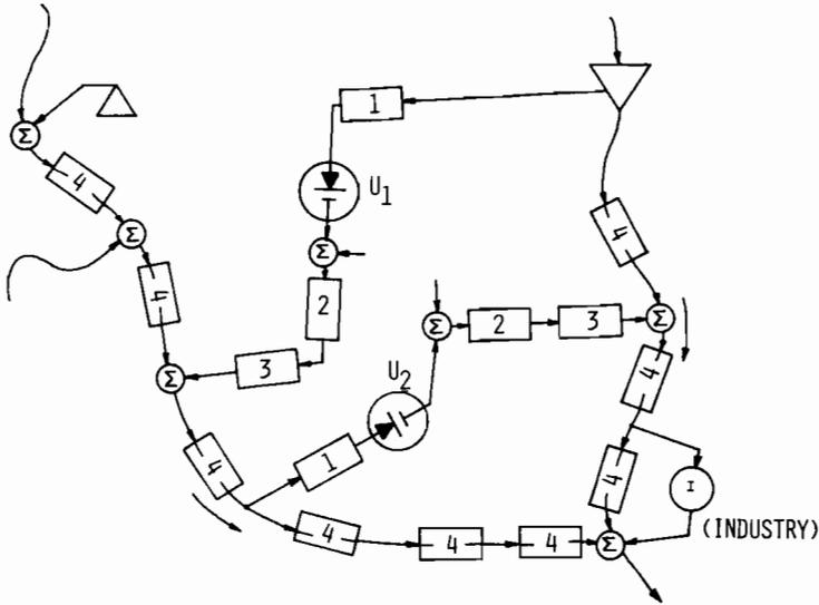
Fig. 11.3 Analytical picture of a hypothetical water resource system.  $U_1$  and  $U_2$  represent urban/industrial centers; the block numbers refer to the subsystems defined in Fig. 11.2.
