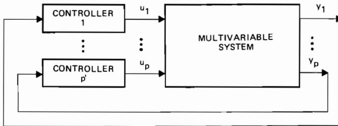
Fig. 14.2 The classical multivariable control system (from Rinaldi et al. 1978).
