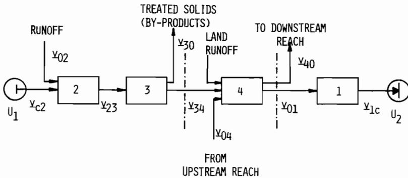
Fig. 11.4 Basic input/output flowchart for  $U_1$  and  $U_2$  in Fig. 11.3. The dashed lines indicate the division of the flowchart for consideration of the control problems in Fig. 11.5.
