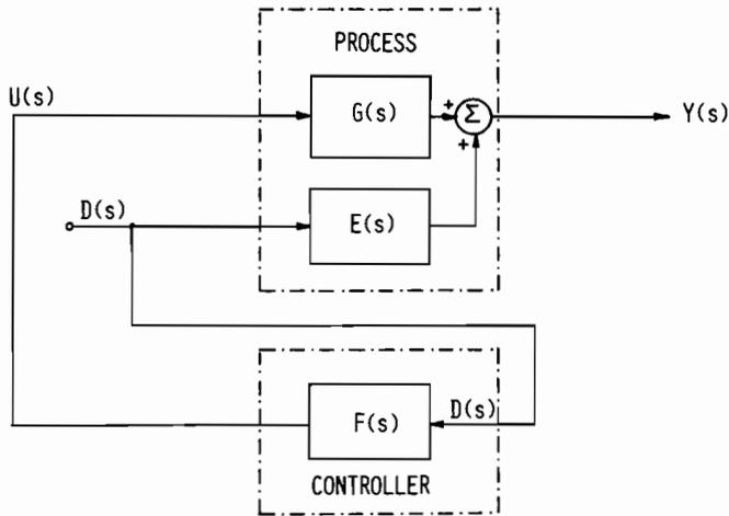
Fig. 11.7 The feedforward controller principle.
