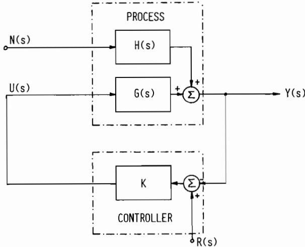
Fig. 11.8 The feedback controller principle.
