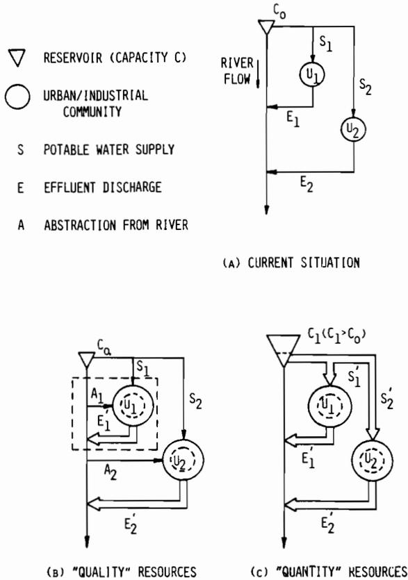
Fig. 11.1 Qualitative and quantitative alternatives for water resources management: (A) current situation; (B) future policy alternative exploiting use and reuse of river water by management of river water quality; (C) future policy alternative based on increased exploitation of clean water sources. Notational relationships:  $S_1' > S_1$ ;  $S_2' > S_2$ ;  $E_1' > E_1$ ;  $E_2' > E_2$ .
