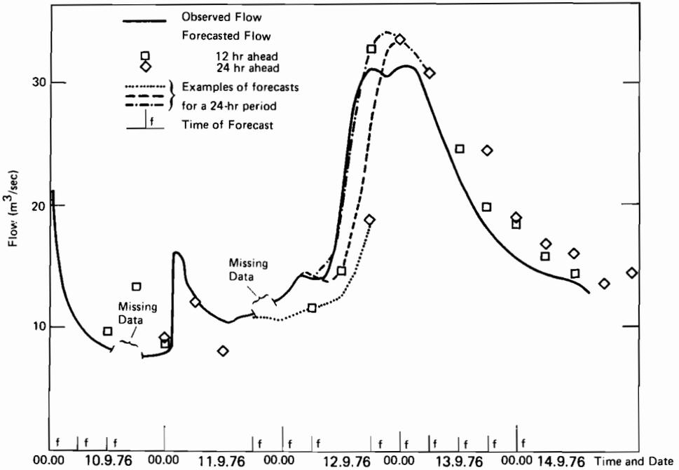
Fig. 16.10 Specimen hydrograph and forecasts of the Dee at Farndon for September 10 to 13, 1976 (from the Dee Weather Radar and Real-Time Hydrological Forecasting Project Report 1977).
