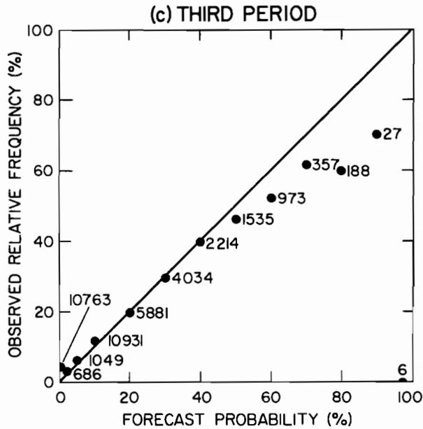
Fig. 15.1 The forecast probabilities versus the observed relative frequencies for the precipitation probability forecasts issued by NWS forecasters in the Southern Region during the period from April 1973 through March 1974 (see Cummings 1974). (a) First-period (0-12 hr) forecasts. (b) Second-period (12-24 hr) forecasts. (c) Third-period (24-36 hr) forecasts.
