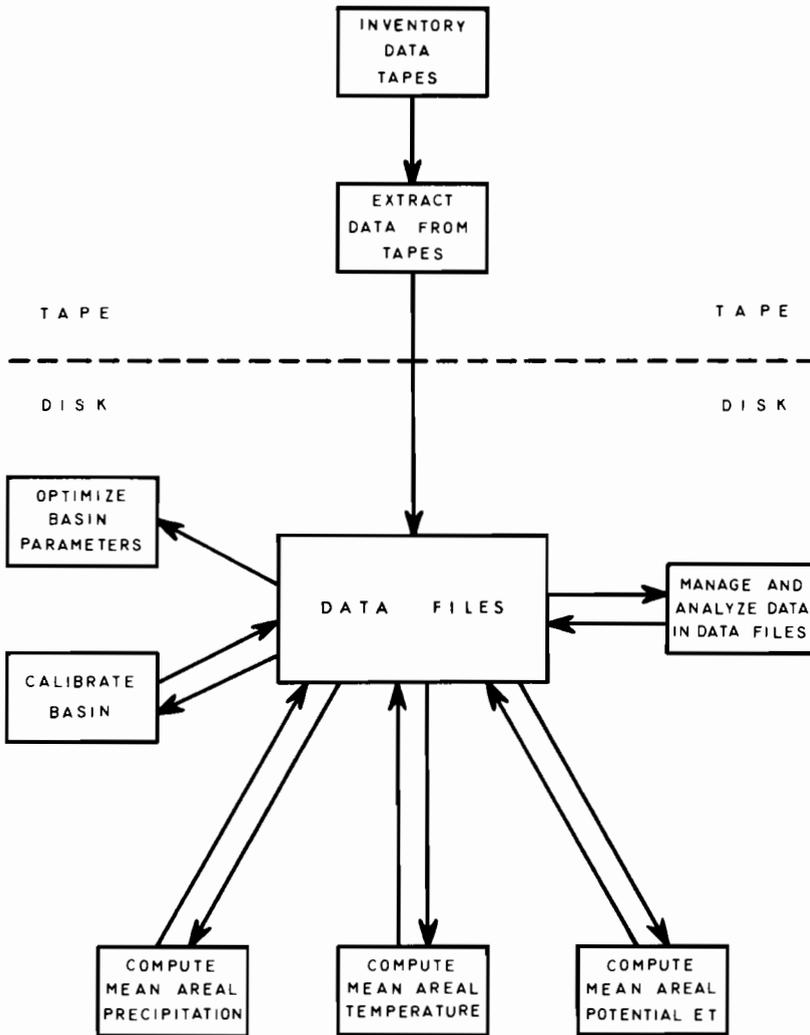
Fig. 18.3 Calibration data management system. ET stands for evapotranspiration.
