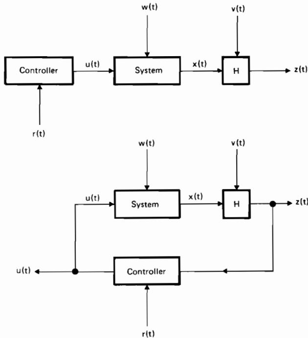
Fig. 1 (top) The open-loop control system. (bottom) The closed-loop control system.
