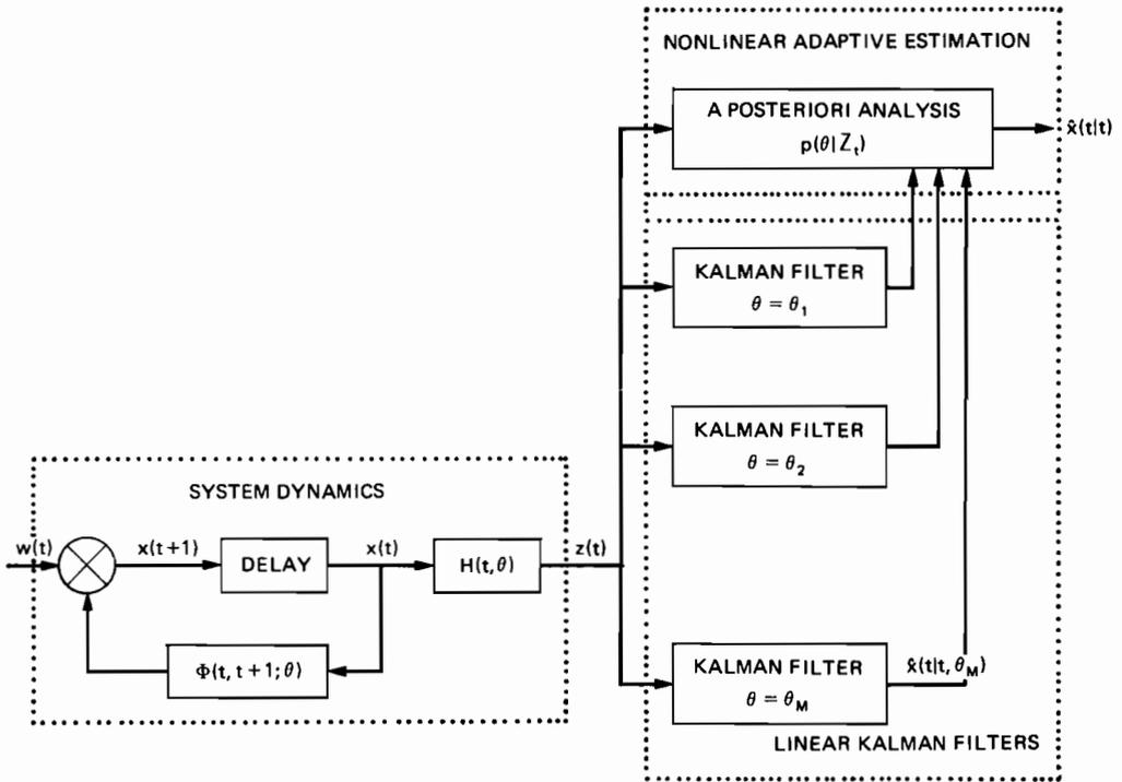
Fig. 12.2 Block diagram of the nonlinear adaptive sequential estimation algorithm for a discrete linear stochastic system with discrete parameters.
