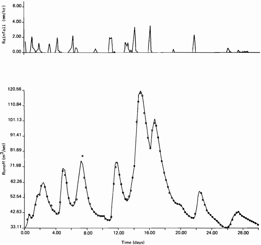
Fig. 9.5 One-step-ahead self-tuning predictor for the Brosna Catchment with  $m = 2$ ,  $n = 2$ , and  $l = 2$ .
