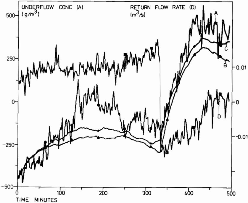
Fig. 6.6 Input and output signals of a hydraulic experiment for the thickener identification. The return sludge flow rate (D) has been manipulated. The underflow concentration level (A) is compared with two model outputs: (B) flow rate used as input; (C) flow rate and mixed liquor suspended solids concentration as input.
