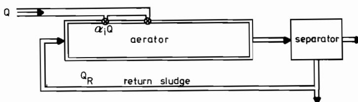
Fig. 6.2 The activated sludge process.
