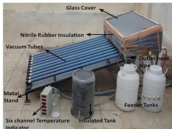
Figure 2: Photograph of experimental set-up with various instruments
