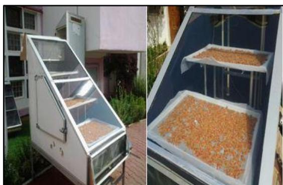
Figure 2: The solar dryer with a deposited waste product on the three trays
