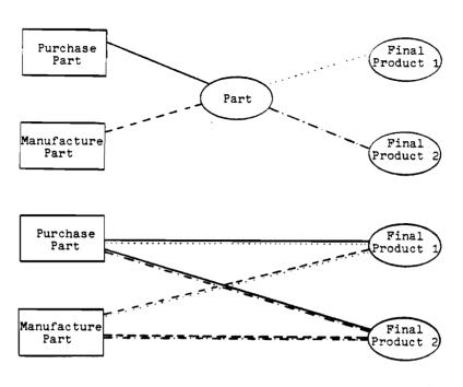
Fig.5: Elimination of a balance equation as general series transformation
