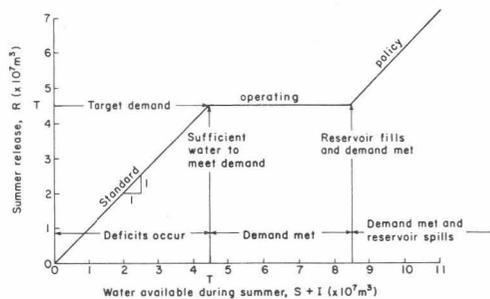
Fig. 3. Standard operating policy for initial storage  $S$  and inflow  $I$  obtained by minimizing the expected loss  $E[l_{\beta}(R)]$  for  $\beta = 1$ .
