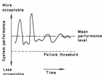
Fig. 2. Variable system performance without failures.
