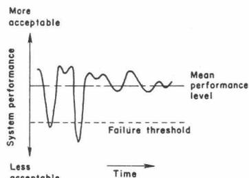
Fig. 1. Variable system performance with infrequent failures.
