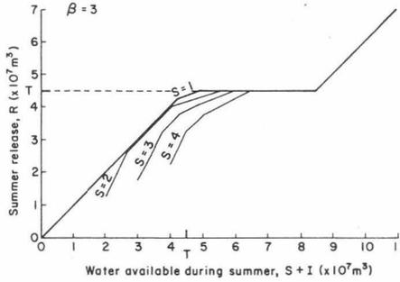
Fig. 4. Optimal summer release policy for  $\beta = 3$ . The lines show best value of release  $R$  as a function of initial storage  $S$  plus inflow  $I$  for specified value of  $S$  and release target  $T$ .
