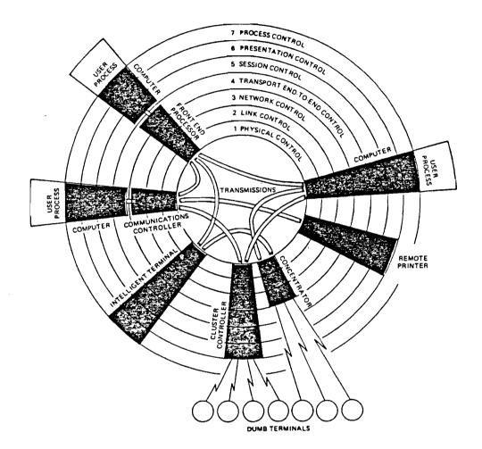
Figure 8. The layers of control are allocated between machines in different ways
