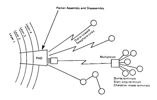
Figure 14. Dumb terminals connected to the network via a PAD (Packet Assembly and Disassembly) interface
