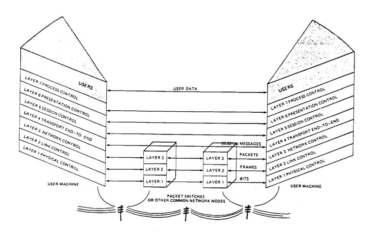
Figure 12. Layers 4 to 7 provide end-to-end communication between session software. Layers 1 to 3 provide an interface to a shared network
