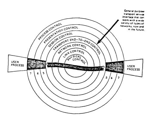
Figure 16. A system which uses the session services layers but not the transmission subsystem layers. It employs the standard interface to Layer 4, but transmission does not use CCITT X.25 mechanisms or similar. It may be a wideband point-to-point channel, CATV, communication satellite network, office network, or merely a computer channel connecting machines in a building
