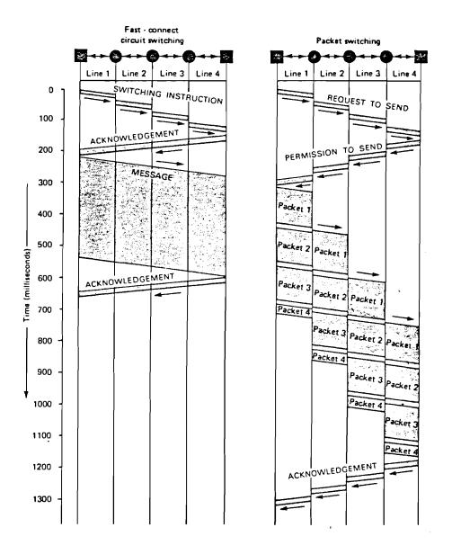
Figure 19. A comparison of the timing on packet switching and fastconnect circuit switching. In this illustration a 400-byte (3200-bit) message is sent on 9600 bps lines. The packet size is 1008 bits. No queuing delays are shown. If the lines were moderately highly utilized queuing delays would lengthen the end-to-end delay with packet switching more than with circuit switching.
