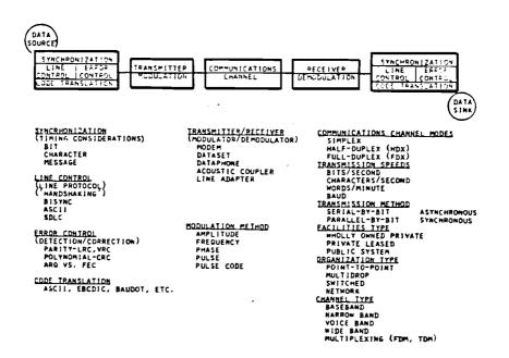
Figure 3. The data communications subsystem with its components as discussed in this chapter [1]
