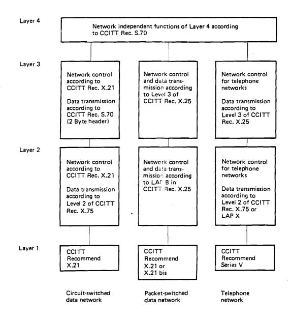
Figure 9. Protocol functions/interface definitons for teletext services over different types of networks (according to CCITT Rec. S.70) described in terms of teletext and videotex services:
