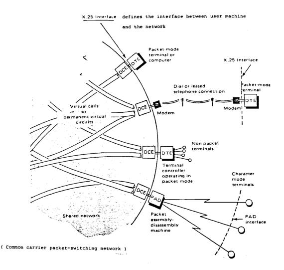
Figure 17. The user machine, DTE, can be computer, terminal, terminal controller, or interface to another form of teleprocessing. The PAD, packet assembly/disassembly machine, buffers characters to and from character-mode terminal (e.g., start-stop machines) and forms the requisite packets.
