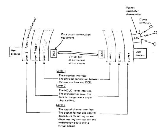
Figure 18. The CCITT X.25 user/network interface is subdivided into three level of interface
