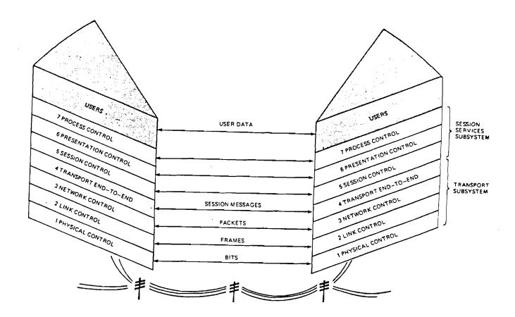
Figure 11. Each layer contains different functions. Each layer communicates with its peer in another machine
