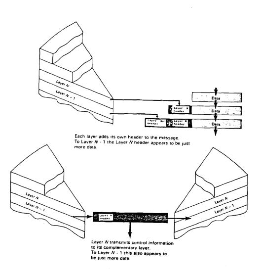
Figure 13. There are two firms of communication between equivalent layers: message headers for that layer, and control messages passed between the layers. These are, or will become, the basis of international standards
