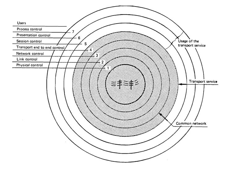
Figure 6. The International Standards Organization's seven layers of control for distributed processing.
