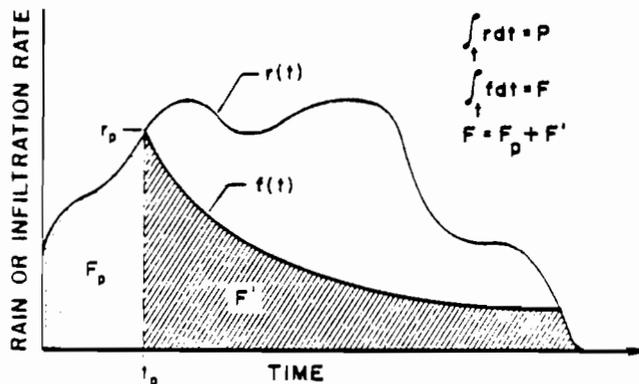
Figure 2. Schematic representation of runoff model using infiltration approach (Smith and Parlange, 1978).
