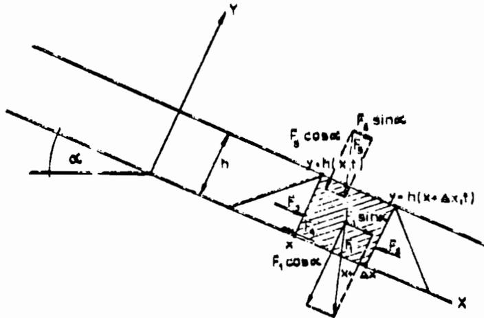
Fig. 2. Scheme for determination of equation of movement.
