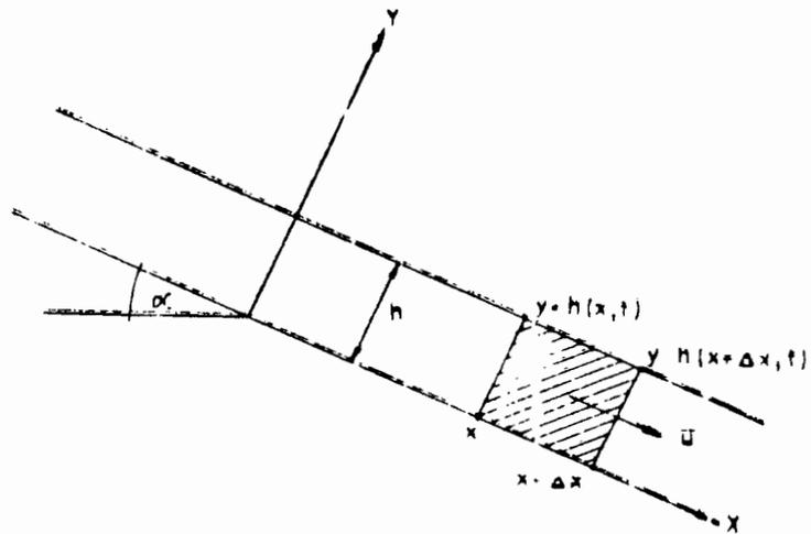
Fig. 1 Scheme for determination of equation of continuity
