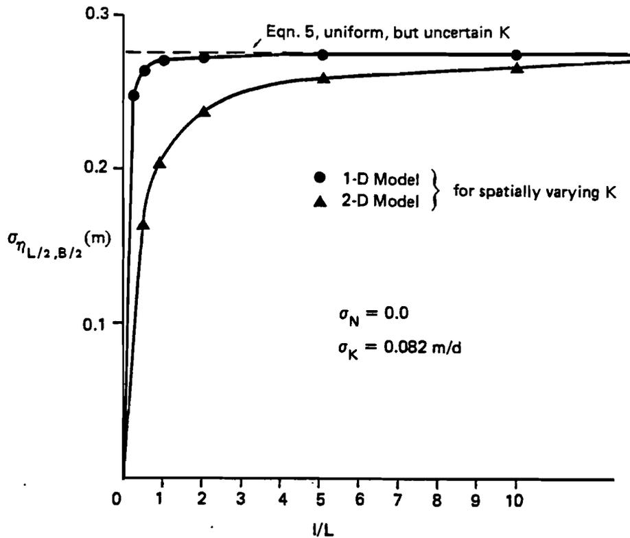
Figure 8.  $\sigma_{h_{L/2}}$  versus Correlation length  $K$  in 2-D for  $l/L > 5$ , once again demonstrating that for sufficiently large correlation length the simple uniform model can be reasonably employed.
