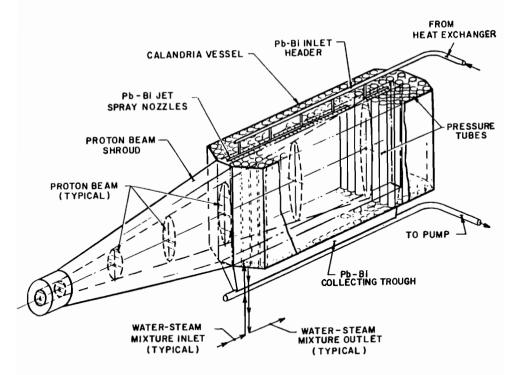
FIGURE 3 A PWR target assembly.
