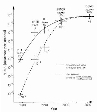
FIGURE 2 Expected neutron yield of future tokamaks (3000 MW  $\simeq 10^{21}$  neutrons per second). (The values for PLT were obtained with deuterium only, but are scaled towards D-T reactions.)
