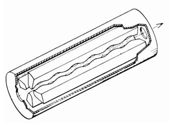
FIGURE 3 A cutaway view of an RFQ accelerating structure (reprinted with permission from Crandall et al., 1979). The RFQ would be the low-energy accelerating structure in an accelerator breeder.
