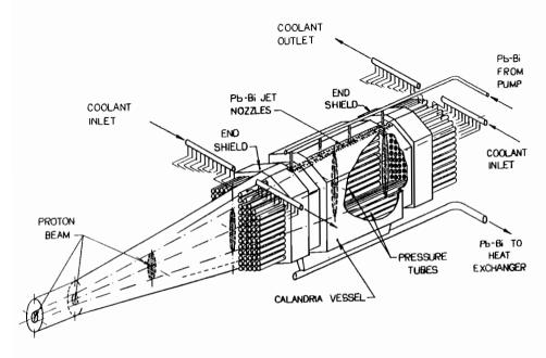
FIGURE 4 An HWR-type target assembly.
