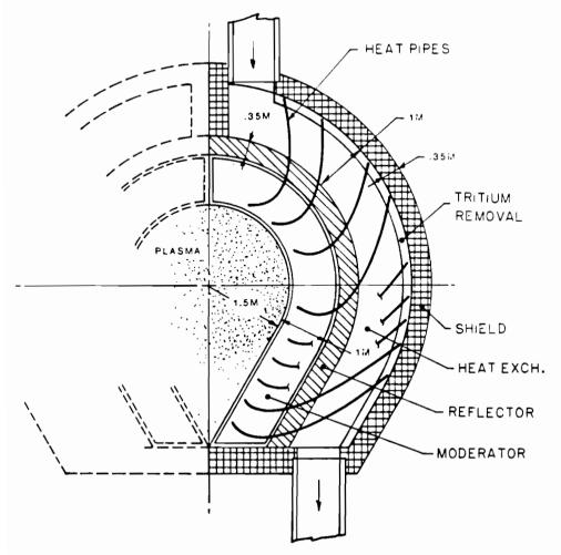
FIGURE 11 A heat-pipe blanket module.
