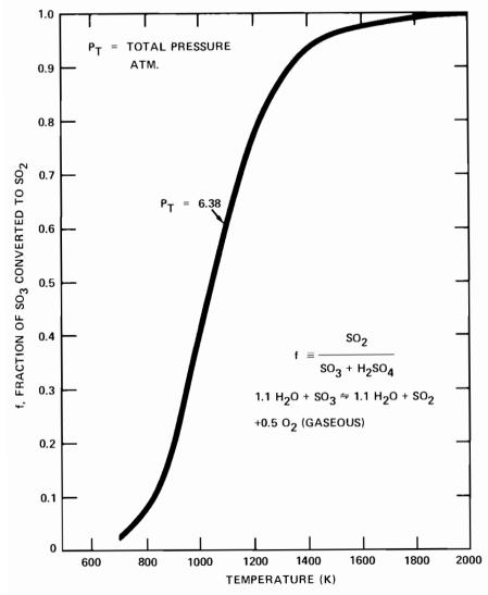
FIGURE 3 The SO<sub>3</sub>-SO<sub>2</sub> equilibrium curve.
