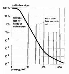
FIGURE 10 Beam loss versus proton energy. The upper limit of beam loss (fractions of total beam per meter of length) permissible for hands-on maintenance of the accelerator decreases steeply with proton energy (curve). The shaded bars show sources of point losses assumed as worst cases for the design of buildings, accelerator components, and handling systems.
