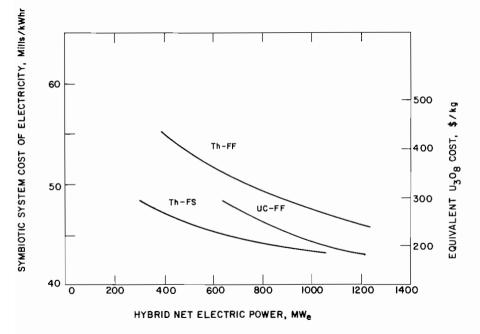
FIGURE 4 System power cost versus fusion breeder net power for three blanket designs.
