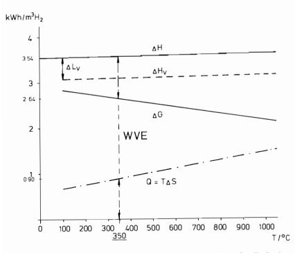
FIGURE 3 Thermodynamic functions of water electrolysis.  $\Delta H = \Delta G + T \Delta S$ , where  $\Delta H$  is the thermoneutral enthalpy,  $\Delta G$  is the free enthalpy supplied as electricity (in the absence of overvoltages and ohmic losses), and  $Q = T \Delta S$  is the enthalpy increment contributed as heat. The position (corresponding to case III in Table 2) for the WVE operated at 350° C is indicated.
