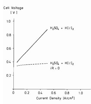
FIGURE 5 The current density versus cell voltage characteristics of the electrolytic step of the advanced sulfuric acid hybrid cycle. The broken curve corresponds to the measured performance without diaphragm (iR = 0).
