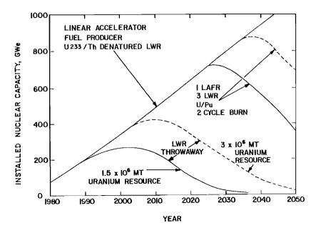
FIGURE 13 Nuclear power growth patterns: the effect of LAFER systems (small  $U_3O_8$  supply) for a capacity growth rate of 15 GWe year<sup>-1</sup>.
