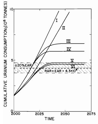
FIGURE 6 Cumulative uranium consumption for the different scenarios shown in Figure 2 for the traditional market-penetration constraint B with an introduction date of 2000.
