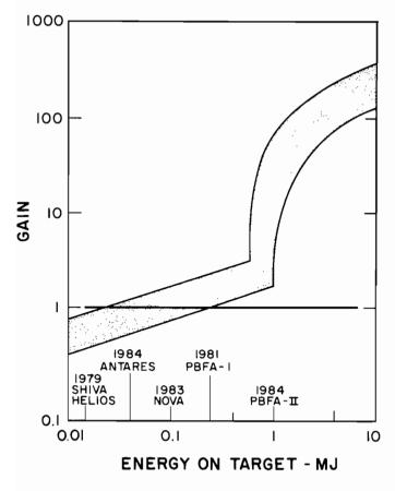
FIGURE 10 Energy-gain predictions for inertial confinement.
