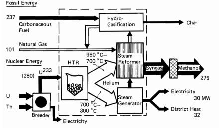
FIGURE 13 A zero-emission energy system for the conversion of dirt into secondary energy.
