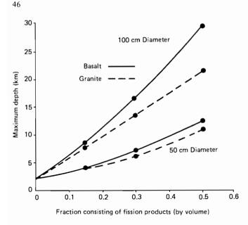
FIGURE 11 Capsules of various diameters, containing fission products of initial age six months, melt the surrounding rock by nuclear decay heat and thus sink. The final depth of penetration is shown as a function of the fraction by volume of fission products, for each combination of capsule diameter and surrounding rock.
