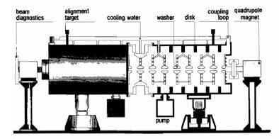
FIGURE 14 A twin tank of the DAW accelerator. Accelerating cells are formed by pairs of washers, while the ring-shaped slit between disks and washers provides a high flow of energy.
