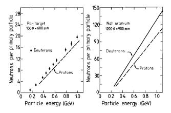
FIGURE 5 Neutron yield per primary particle for protons and deuterons on lead  $(100\phi \times 600 \text{ mm})$ and natural uranium  $(1200\phi \times 900 \text{ mm})$  targets (after Barashenkow et al., 1974);  $\phi$  denotes diameter (mm).
