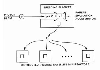
FIGURE 1 A schematic representation of an accelerator-supported system of fission minireactors.
