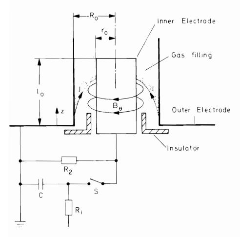
FIGURE 1 The start-up of a plasma focus discharge (schematic).
