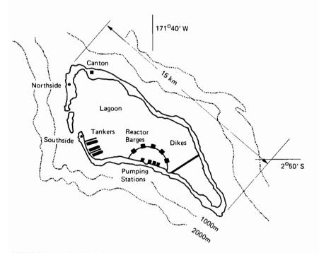
FIGURE 6 A plan view of Canton Island, with the installation drawn to scale. Each barge represents 200 GWth of primary energy. The island is located in the central equatorial Pacific  $(171^{\circ} 40'W, 2^{\circ} 50'S)$ .
