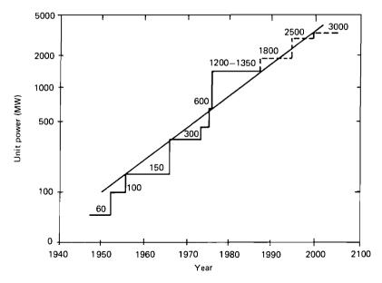
FIGURE 2 The relation between the size of electric generators and electrical energy consumption in the Federal Republic of Germany. For relatively short intervals, the size of generators is always proportional to consumption.
