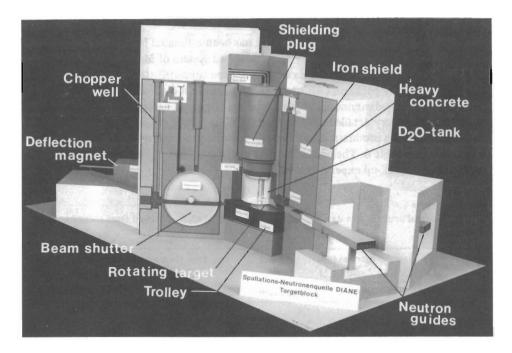
FIGURE 18 A cutaway model view of the target block of the target station DIANE
