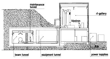
FIGURE 11 A cross section of the DAW accelerator. Zones of different accessibility are delimitated from each other; the building of the RF gallery is freely accessible during machine operation.
