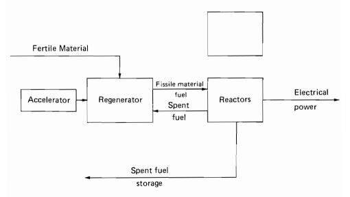
FIGURE 6 The scheme of the LAFER.
