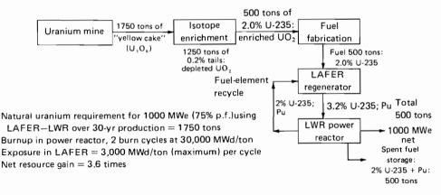
FIGURE 9 A LAFER fuel cycle with no reprocessing.
