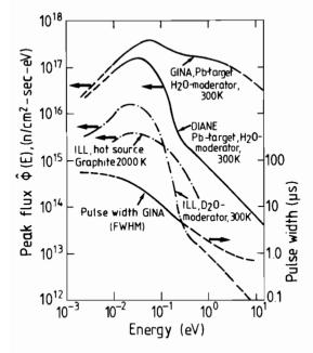
FIGURE 20 Peak neutron flux at DIANE as a function of energy in comparison to the steady-state flux at the HFR, Grenoble. The pulse width at DIANE is about  $500 \,\mu$ s for all energies and the time-average flux is a factor of 18–20 below the peak flux. The curve labeled GINA is for the option of a pulsed source as outlined in the text.
