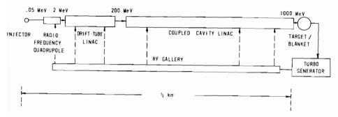
FIGURE 1 A schematic diagram of the main components of an accelerator breeder.
