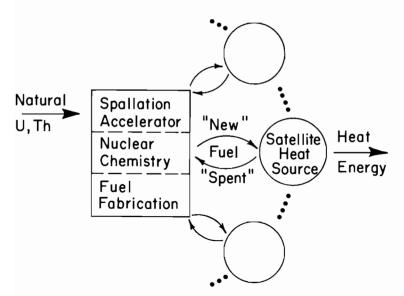
FIGURE 1 A graphical depiction of a central facility supplying a number of small heat sources with rejuvenated fuel. The power requirements for the central facility – which form part of the overall power balance – are not shown.
