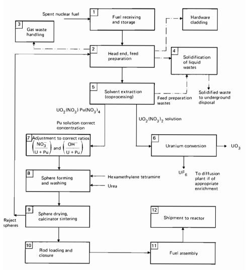
FIGURE 1 Generalized fuel-cycle flow sheet.
