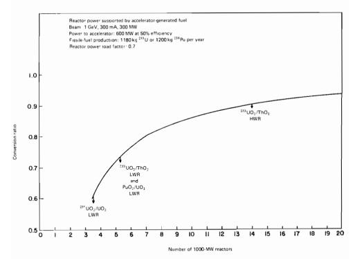
FIGURE 12 The reactor power supported by accelerator-generated fuel.
