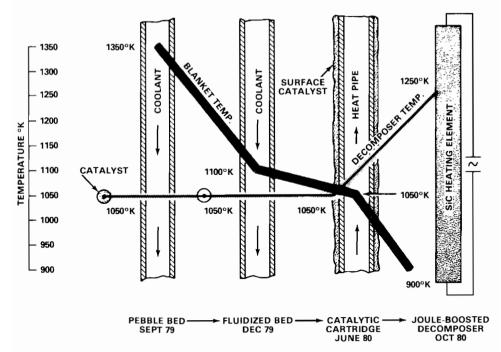
FIGURE 10 Progress in lowering the blanket temperature and raising the decomposer temperature for synfuel applications.
