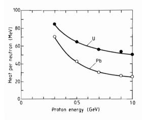
FIGURE 7 Heat release per neutron for lead and uranium as a function of proton energy (from Bartholomew and Tunnicliffe, 1966).
