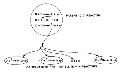
FIGURE 2 A depiction of a set of  $D^{-3}$ He fusion minireactors supported by a <sup>3</sup>He-breeding fusion reactor.
