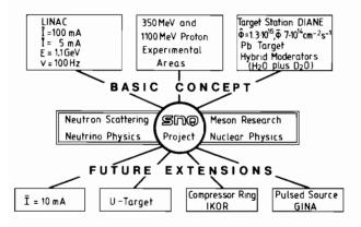
FIGURE 3 The basic concept, fields of research, and optional future extensions of the SNQ project.
