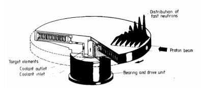
FIGURE 16 A schematic representation of the rotating target arrangement with individually canned target pins cooled by water which flows in and out through the hub of the wheel. The diameter of the wheel is 2.5 m and the height of the target material is 10 cm. The distribution of fast neutron leakage as calculated with the HFT code is indicated for the upper surface.
