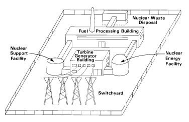
FIGURE 7 A schematic representation of a synergetic nuclear energy system. As indicated, one facility is optimized for energy production while another provides a support capacity. As suggested here, intrinsically safe fertile materials only would be transported into this energy park and energy is supplied to a power grid.
