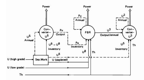
FIGURE 9 A converter-breeder system.
