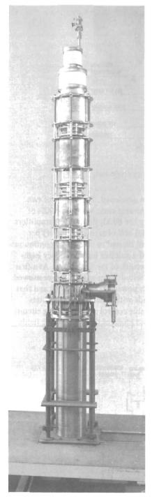
FIGURI-15 The test klystron VE07SK. With a power capability of 1.5 MW and an efficiency of 70% the klystron is a development step towards the SNQ series production klystron.
