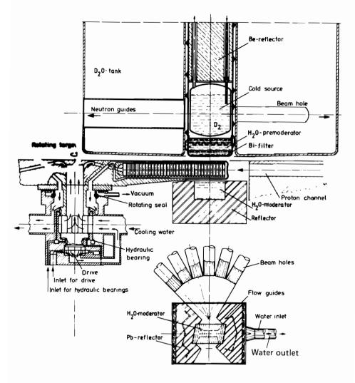
FIGURE 17 The hybrid moderator concept proposed for the target station DIANE. A large volume of high neutron flux, housing the cold neutron source and irradiation facilities (not shown), is arranged above the target to facilitate access from above. The  $H_2O$  moderator below the target is surrounded by a lead reflector on three sides and is viewed by 12 beam tubes.
