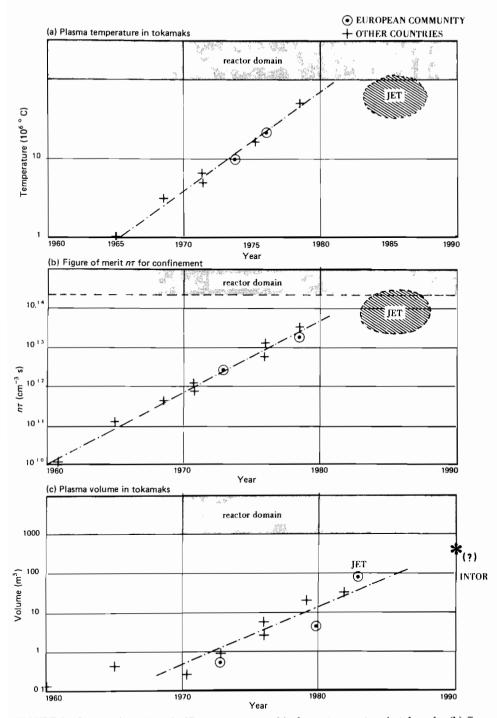
FIGURE 3 Progress in various significant parameters: (a) plasma temperature in tokamaks, (b) figure of merit  $n\tau$  for confinement, (c) plasma volume in tokamaks. (By courtesy of the European Community Fusion Programme.)
