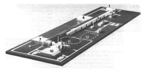
FIGURE 4 A model view of the SNQ facility The buildings of the basic concept are shown together with the locations foreseen for the compressor ring and a future pulsed neutron source: 1, injector building; 2, test building; 3, RF gallery; 4, 350-MeV experimental area; 5, operations building; 6, accelerator tunnel; 7, 1100-MeV experimental area; 8, maintenance building; 9, target building; 10, neutron-guide hall; 11, future compressor ring; 12, future pulsed source.
