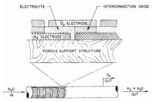
FIGURE 6 HTE cell design (the Westinghouse fuel cell).
