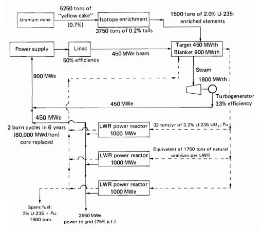
FIGURE 11 A system of three LWRs supplied by one LAFER.
