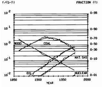
FIGURE 2 Global primary-energy substitution: a logarithmic plot of the transformation f/(1-f) where f is the fractional market share. The smooth curves are model estimates of historical data; the zigzag lines are historical data; the straight lines show the logistic model substitution paths.
