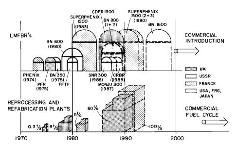
FIGURE 8 The current status and planned facilities for LMFBRs and associated fuel-cycle plants.
