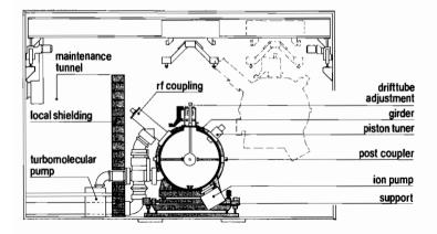
FIGURE 13 A cross section of the beam tunnel in the Alvarez accelerator.
