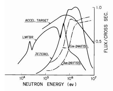
FIGURE 2 Neutron spectra and fission cross-sections.
