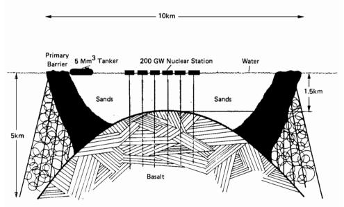
FIGURE 7 A scale cross section of Canton "Energy Island" with its presumed geological structure. The full lines under the power station barges represent permanent radioactive-waste sink holes and the broken extensions represent the free trajectories of the sinking capsules.
