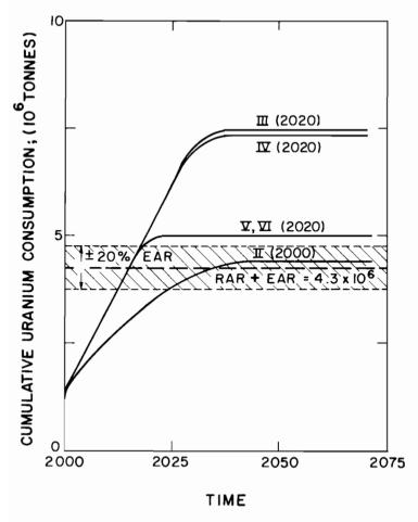
FIGURE 5 A comparison between breeder scenario II and hybrid scenarios III–VI for the marketpenetration constraint  $\Lambda$  with introduction dates of 2000 and 2020, respectively.
