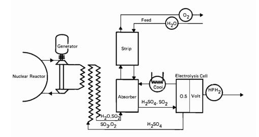
FIGURE 8 A possible block flow sheet for the realization of the Westinghouse sulfur cycle (Farbman, 1976). Sulfuric acid is decomposed thermally and  $SO_2 + SO_3$  are stripped in an absorption column where the electrolyte of a cell is circulated.  $SO_2$  is transformed into  $SO_3$  electrolytically.
