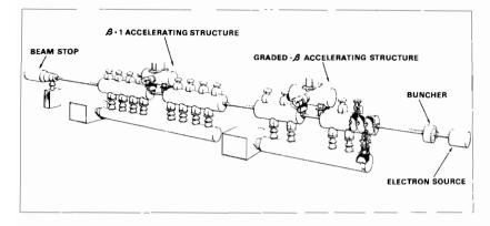
FIGURE 5 The Chalk River Nuclear Laboratories electron test accelerator for experiments on the acceleration of intense beams with a large accelerating gradient at 100% duty factor in a coupled-cavity linac typical of the high-energy section of an accelerator breeder.
