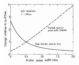
FIGURE 8 The change in peak thermal neutron flux and thermal neutron pulse width with proton pulse duration at constant source strength and repetition rate (H<sub>2</sub>O moderator, with a decay time  $\tau$  of the thermal neutron field of 200  $\mu$ s). The FWHM at  $t_p = 0.5$  ms is 0.516 ms.
