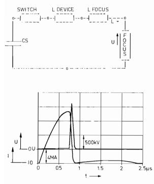
FIGURE 5 (Top) Auxiliary circuit of a plasma focus device. (Bottom) Voltage across and corresponding current in the power-amplifier compressor: W = 1 MJ;  $C = 32 \mu$ F;  $L_{tot} = 7$  nH; U = 250 kV.
