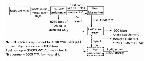
FIGURE 8 The conventional LWR nuclear fuel cycle.
