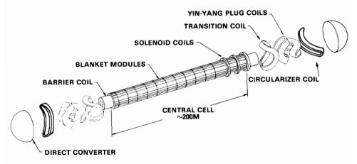
FIGURE 8 The tandem-mirror reactor.
