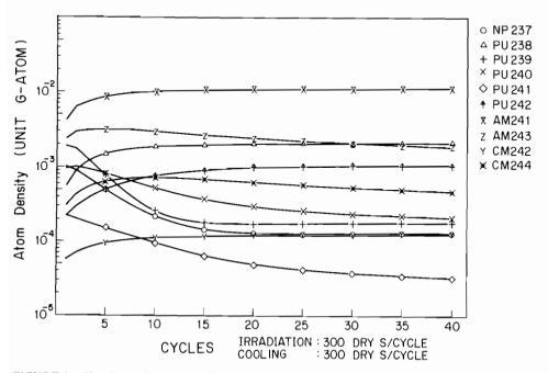
FIGURE 4 The change in atom density at each cycle in the ABFR.
