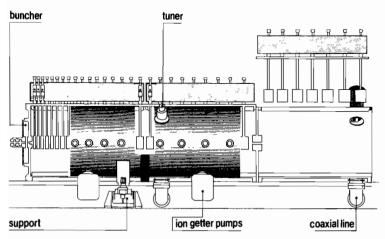
FIGURE 12 The first tank of the Alvarez accelerator. The buncher is directly flanged to the front end plate. Sets of drift tubes are suspended from girders.
