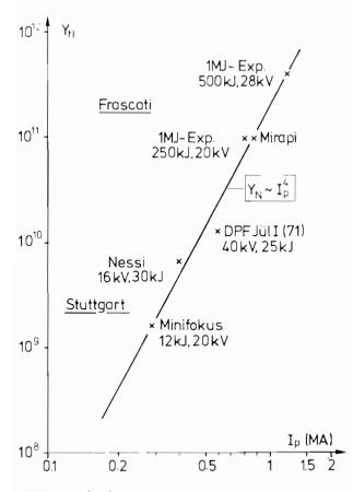
FIGURE 4 <sup>2</sup>H-<sup>2</sup>H neutron yield as a function of plasma current.
