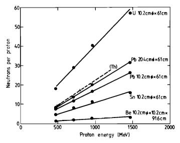
FIGURE 6 Neutron yield per incident proton as a function of proton energy for various target materials (from Bartholomew and Tunnicliffe, 1966; the data for thorium are taken from Garvey, 1980, and Russell et al., 1981).
