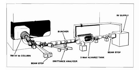
FIGURE 4 The Chalk River Nuclear Laboratories high-current test facility for experiments on the acceleration of intense proton beams at 100% duty factor in a drift-tube linac typical of the intermediate-energy section of an accelerator breeder.
