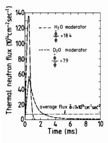
FIGURE 19 The time structure of the thermal neutron flux in the moderators of DIANE as derived from measured data.
