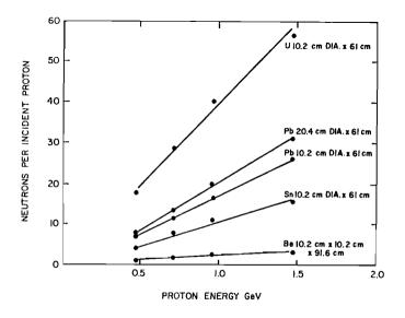
FIGURE 1 The experimental yield of neutrons obtained by bombardment of a heavy-metal target with high-energy protons.
