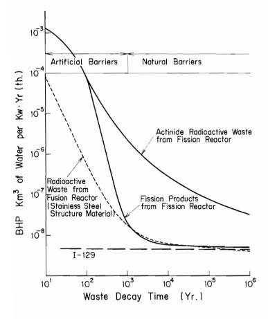
FIGURE 1 Decay and hazard characteristics of radioactive waste from fusion and fission reactors.
