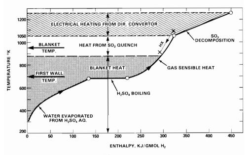
FIGURE 9 The heating curve for the H<sub>2</sub>SO<sub>4</sub> process step.
