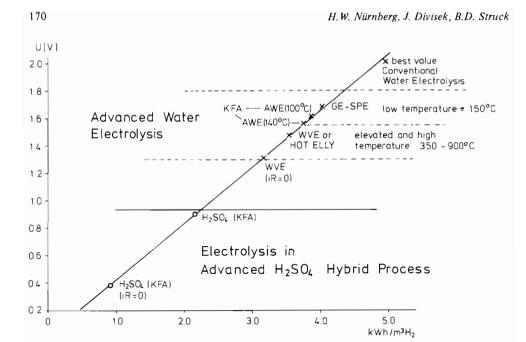
FIGURE 6 Relationship between required electricity in kilowatt-hours per cubic meter of  $H_2$  and cell voltage U. The points inserted for various electrolytic procedures refer to a current density of 0.53 A cm<sup>-2</sup>.
