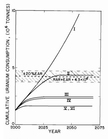
FIGURE 4 The variation of cumulative uranium consumption with time for the different scenarios shown in Figure 2 (these represent the lowest possible values since constraint A is used with an introduction date of 2000).
