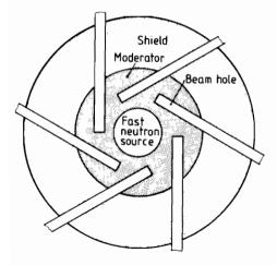
FIGURE 1 A schematic representation of a neutron source for beam-hole research.
