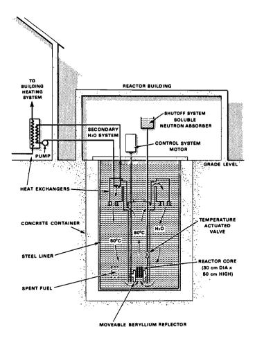
FIGURE 2 A 2-MW SLOWPOKE heating reactor.
