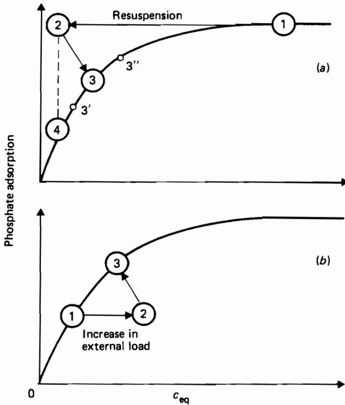
**Figure 7.8.** (a) Desorption and (b) adsorption related to sorption isotherms.
