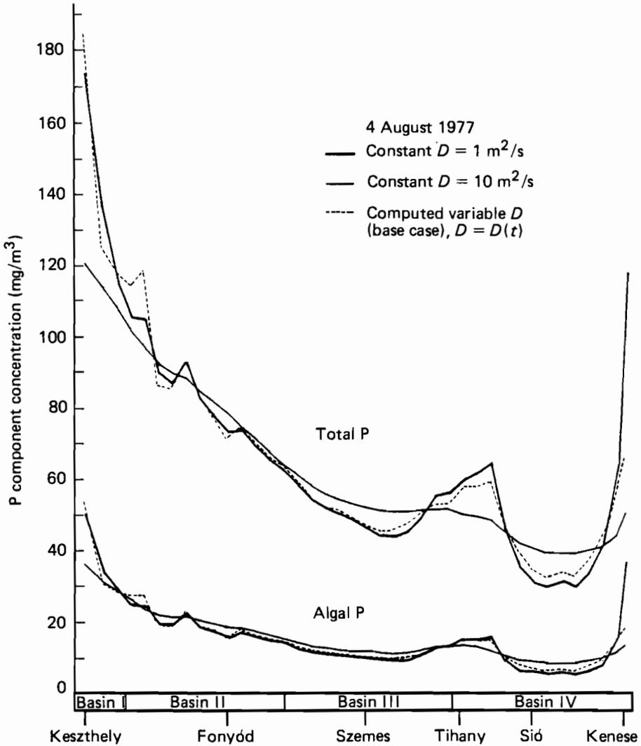
**Figure 10.7.** (b) Effect of model dispersion on predicted P distribution: comparison with constant dispersion.
