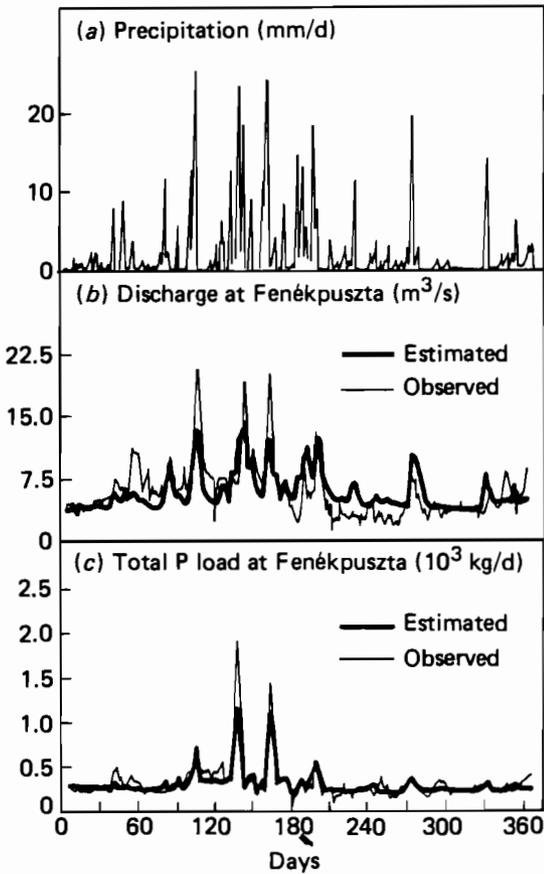
**Figure 6.3.** Calibration of the time-series model: (a) observed precipitation sequence for 1978; (b) observed and estimated stream discharge; (c) total P load at Fenékpuszta.
