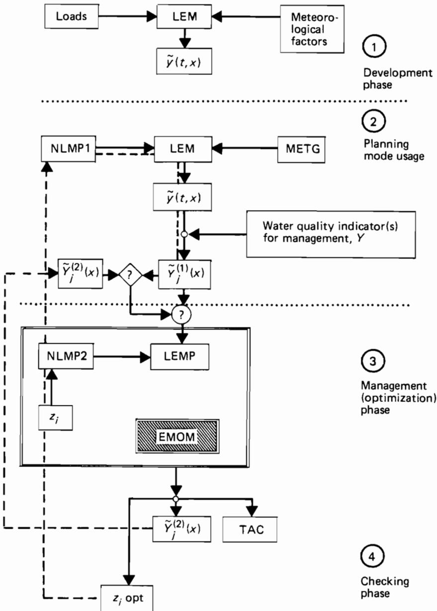
**Figure 4.1.** Structure of the analysis. LEM, lake eutrophication model; NLM, nutrient loading model; EMOM, eutrophication management optimization model; METG, meteorology generator;  $c_j$  state variables of LEM;  $Y_j$  water quality indicators;  $z_i$  control variables; TAC, total annual cost.
