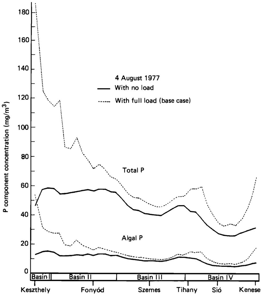
**Figure 10.9.** Effect of nutrient loading on predicted P dynamics in Keszthely Bay.
