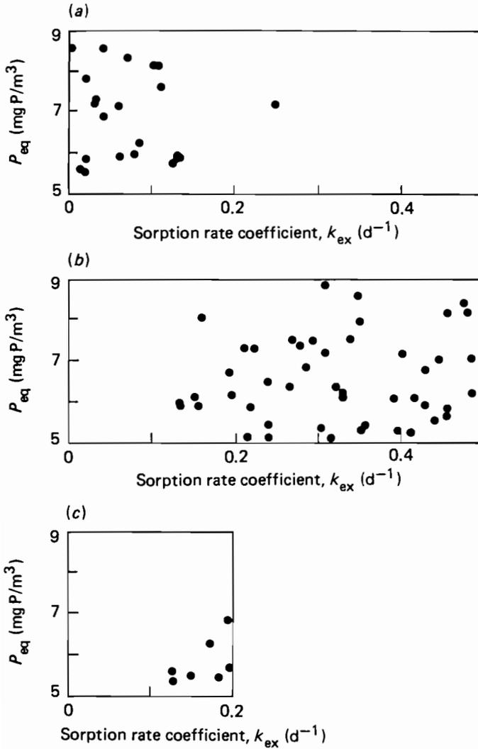
**Figure 11.9.** Monte Carlo simulation results for distribution of equilibrium concentration ( $P_{eq}$ ) and sorption rate coefficient ( $k_{ex}$ ). (a) Runs with total P behavior (series 1); (b) runs with total dissolved and dissolved inorganic P behavior (series 1); (c) full behavior runs (series 2).
