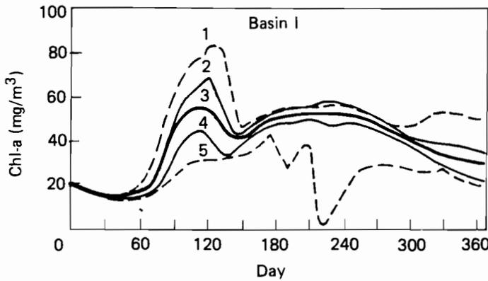
**Figure 4.4.** Influence of uncontrollable factors (e.g., climatic) on water quality. 3, mean; 2 and 4,  $\pm$  standard deviation; 1 and 5, extremes (from 200 Monte Carlo simulations).
