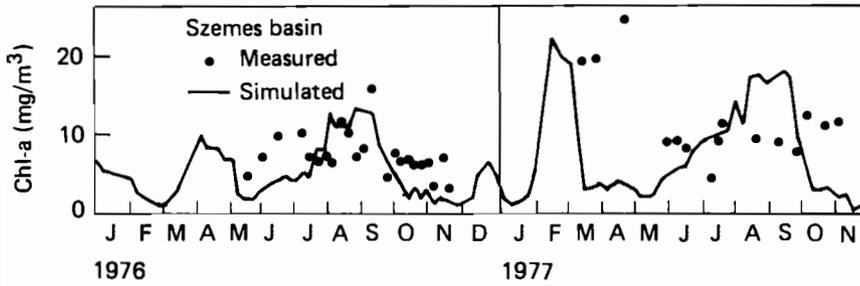
**Figure 12.4.** Measured and simulated Chl-a concentrations in Basin III (Szemes basin), 1976–77.
