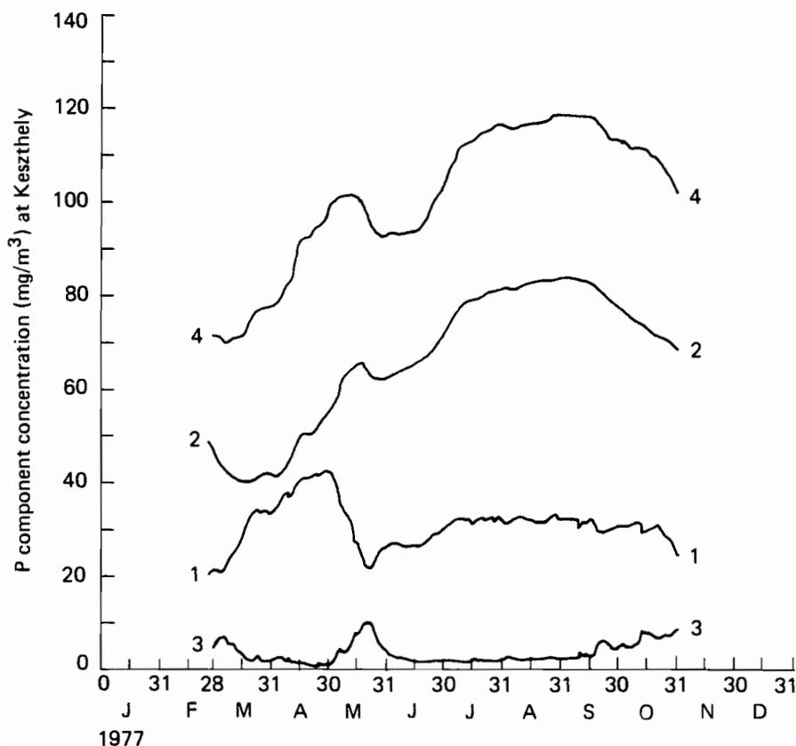
**Figure 10.8.** (a) Effect of model dispersion on predicted P dynamics in Keszthely Bay: with constant dispersion,  $D = 10 \text{ m}^2/\text{s}$ . 1 = total algal P; 2 = detrital P; 3 = dissolved inorganic P; 4 = total P.
