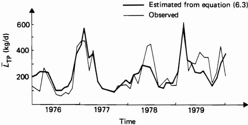
**Figure 6.5.** Calibration of the regression model for the Zala River.
