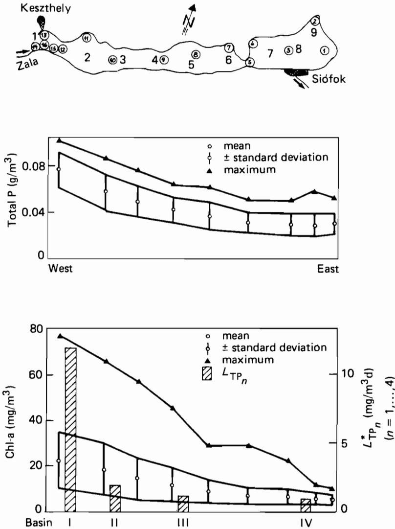
**Figure 1.2.** Longitudinal distribution of water quality and P loads, 1976-78. 1-9 and 1-16 (encircled; point 6 not included because not used after the initial investigations) are sampling locations of VITUKI and the Central Transdanubian District Water Authority, respectively.
