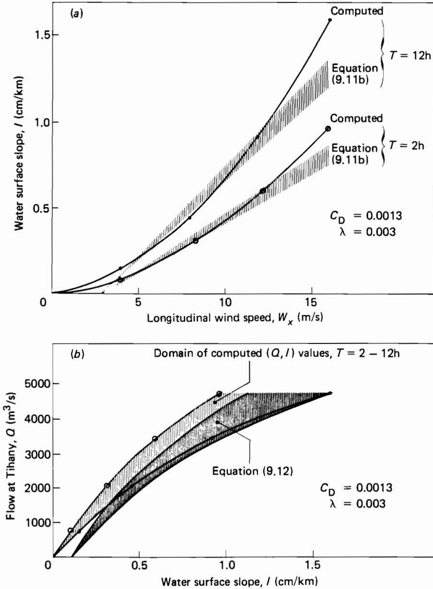
**Figure 9.10.** Comparison of model calibration with Muszkalay's empirical formulas. Comparison of computer predictions with (a) equation (9.11b), and (b) equation (9.12).
