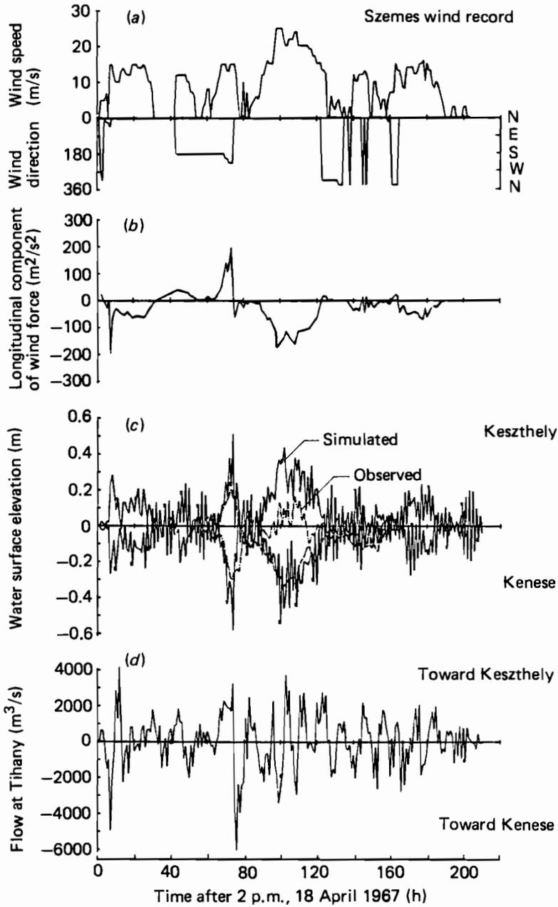
**Figure 9.13.** Comparison of simulation results with observations for the event of 18 April 1967. (a) Wind speed and direction at Szemes; (b) longitudinal component of wind force; (c) water surface elevation at Keszthely and Kenese; (d) flow at Tihany.
