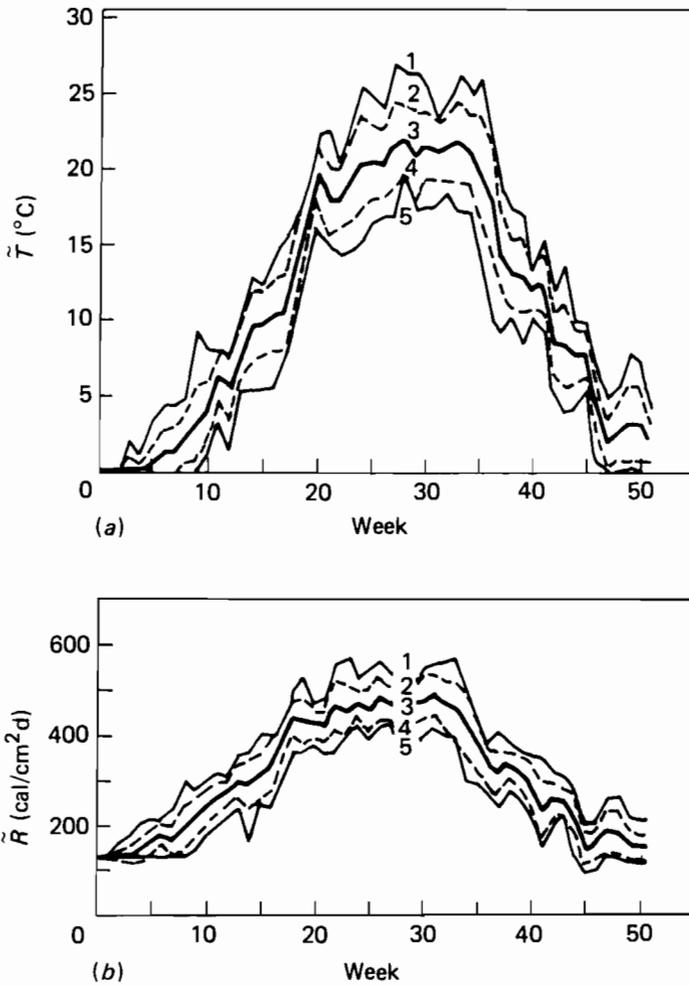
**Figure 4.3.** Generation of (a) water temperature,  $\tilde{T}$ , and (b) global radiation data,  $\tilde{R}$ . 3, mean; 2 and 4,  $\pm$  standard deviation; 1 and 5, extremes (all from 1000 Monte Carlo simulations).
