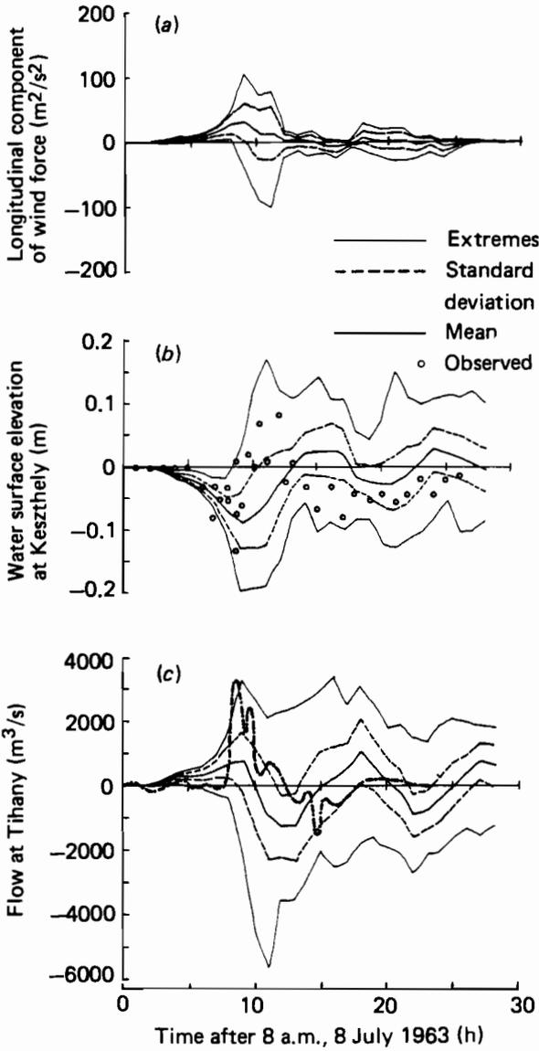
**Figure 9.16.** Monte Carlo simulation of the event of 8 July 1963. (a) Longitudinal component of wind force; (b) water surface elevation at Keszthely; (c) flow at Tihany.
