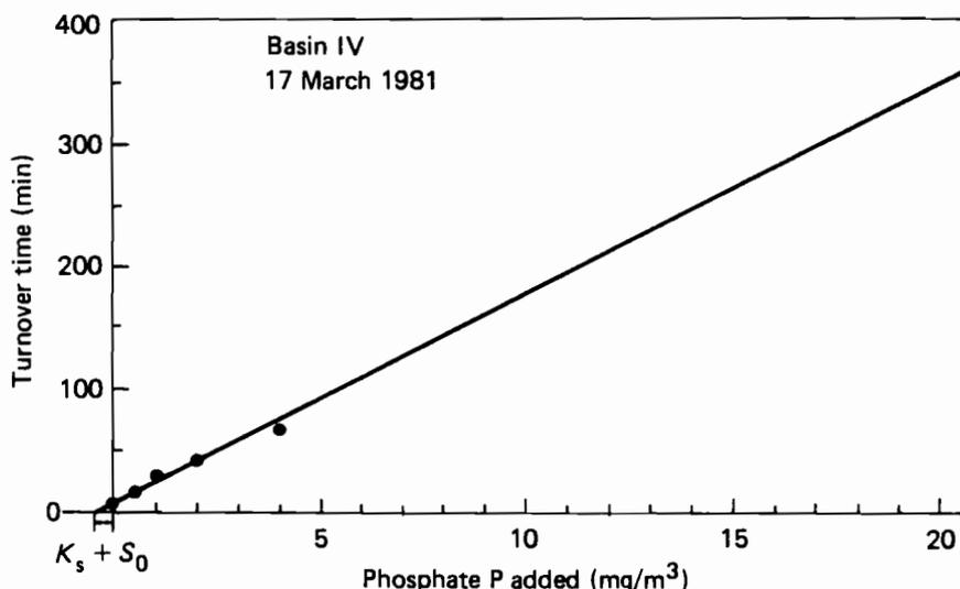
**Figure 8.10.** Turnover time of orthophosphate in lake water samples as a function of the added phosphate P.
