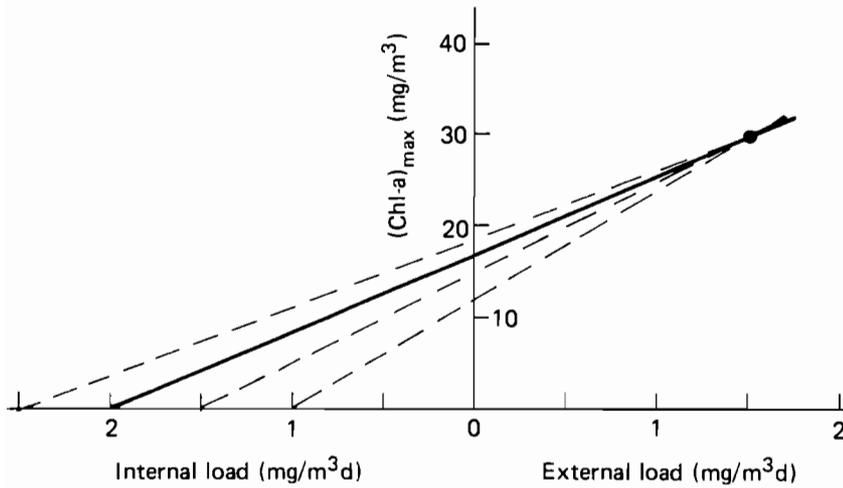
**Figure 3.8.** Estimation of internal load by in-lake parameter estimation and the effect of parameter uncertainty on load uncertainty.
