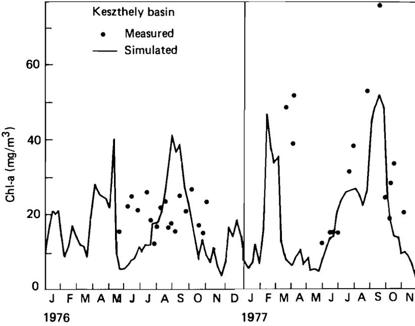
**Figure 12.2.** Measured and simulated Chl-a concentrations in Basin I (Keszthely basin), 1976–77.
