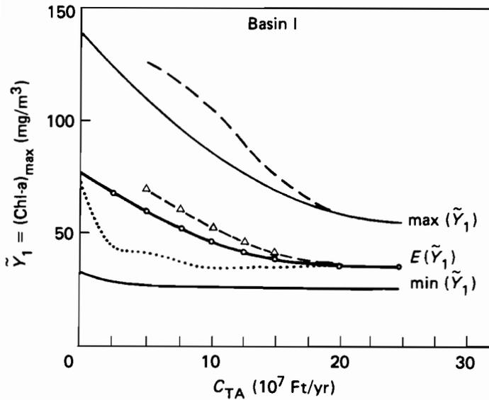
**Figure 4.14.** Sensitivity of the solution to P retention and prescribed effluent standards. —, basic case; ---,  $r_i = 1$ ; ....,  $r_i = 1$  with a prescribed effluent standard ( $2 \text{ g/m}^3$ ).
