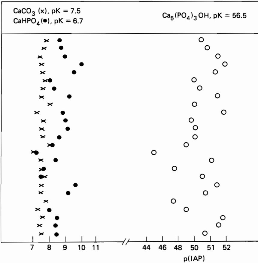
**Figure 7.4.** Ion activity products (IAP) of three minerals for lake water and pore water samples from Lake Balaton. Values expressed as a negative logarithm,  $p(\text{IAP})$ .
