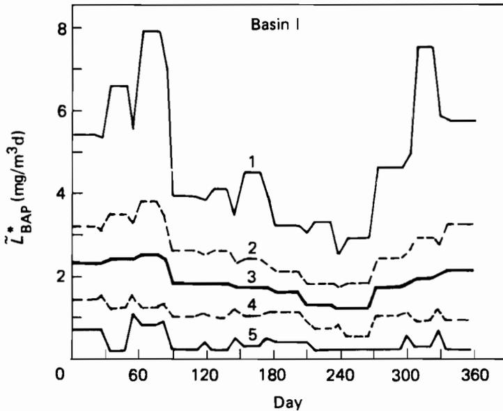
**Figure 4.2.** Generation of the volumetric biologically available P load. 3, mean; 2 and 4,  $\pm$  standard deviation; 1 and 5, extremes.
