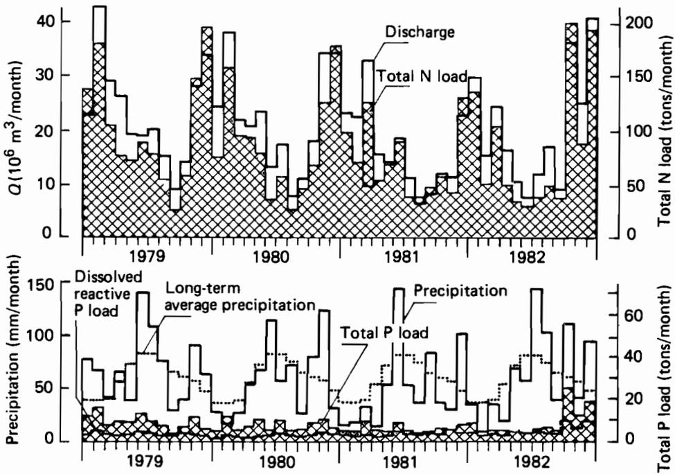
**Figure 14.4.** (b) Monthly average precipitation, discharge, and nutrient loads for the Zala River, Fenékpusztá, 1979–82.
