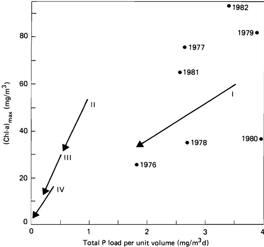
**Figure 3.3.** Trend in reaction of  $(\text{Chl-a})_{\text{max}}$  to P load reductions according to OECD empirical relations. Historical variability for Keszthely basin is also shown.
