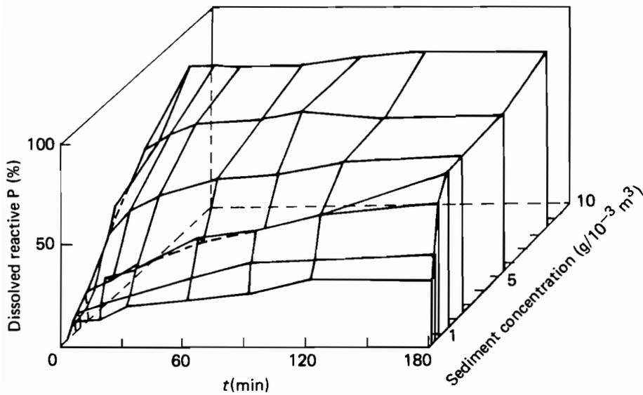
**Figure 7.6.** Phosphate adsorption as a function of time and suspended solids (Keszthely sediment).
