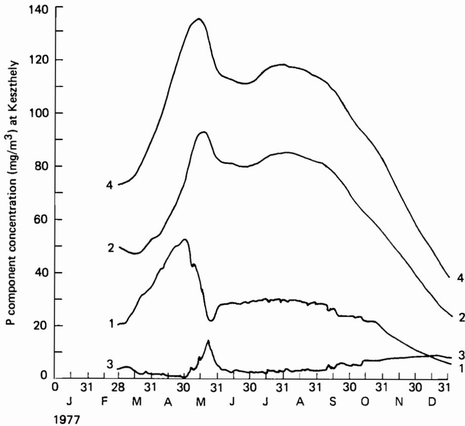
**Figure 10.8.** (a) Effect of model dispersion on predicted P dynamics in Keszthely Bay: with hydrologic flow only (no dispersion),  $D = 0$ . 1 = total algal P; 2 = detrital P; 3 = dissolved inorganic P; 4 = total P.
