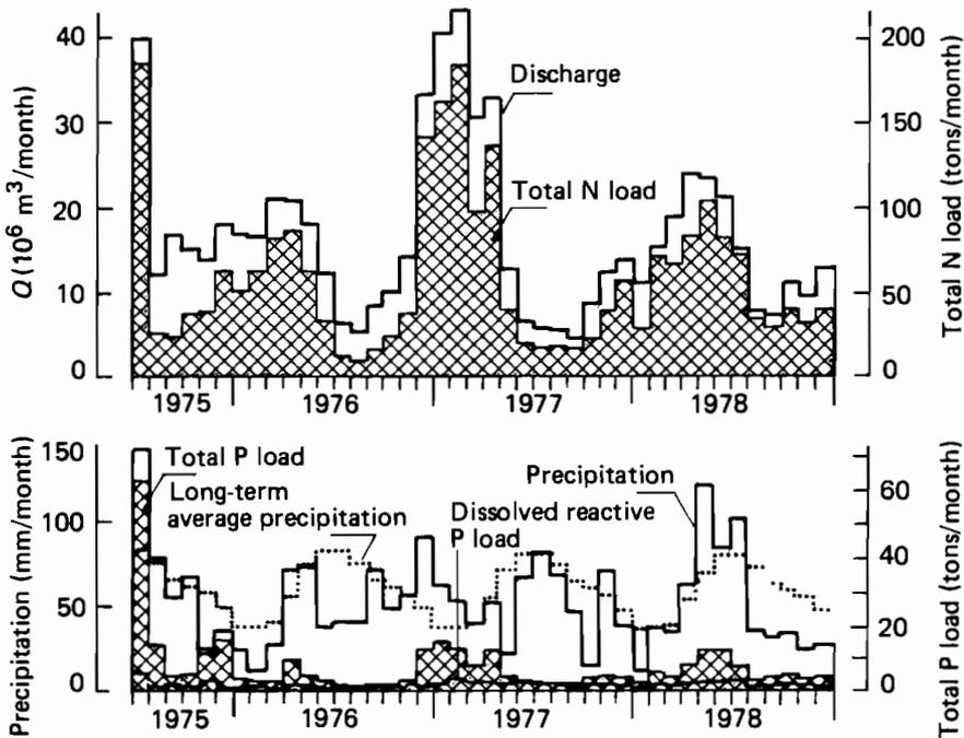
**Figure 14.4.** (a) Monthly average precipitation, discharge, and nutrient loads for the Zala River, Fenékpuszta, 1975–78.
