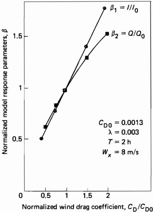
**Figure 9.9.** Summary of model sensitivity to the wind drag coefficient,  $C_D$ .
