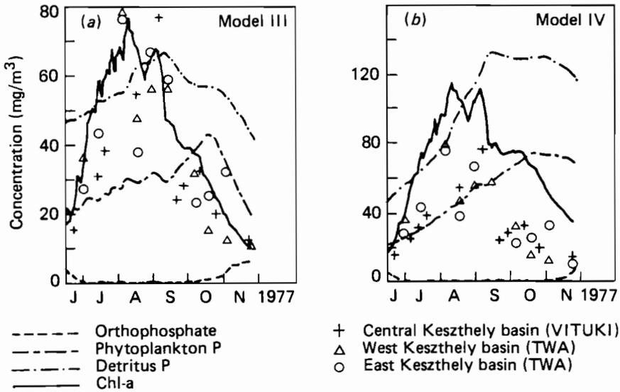
**Figure 13.4.** (a) Model III calibration; (b) model IV run using model III parameters (note the difference in scales).
