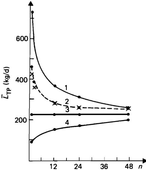
**Figure 6.13.** Influence of infrequent sampling on the estimate of the multiannual average total P load (Zala River, 1976-79): 1 and 4,  $\max(\bar{y}_n)$  and  $\min(\bar{y}_n)$ ; 2,  $E(\bar{y}_n) + 1.96 \sigma_n$ ; 3,  $E(\bar{y}_n)$ .
