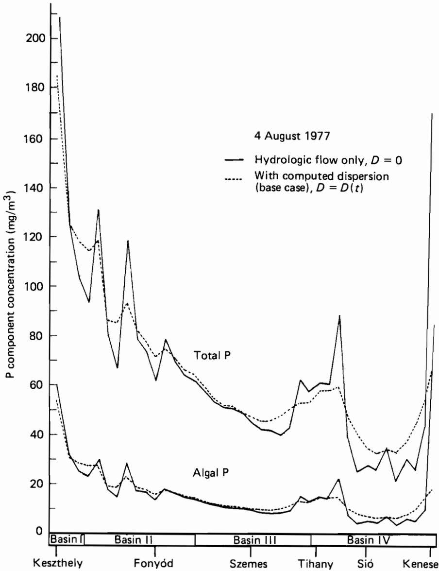
**Figure 10.7.** (a) Effect of model dispersion on predicted P distribution: comparison with zero dispersion.
