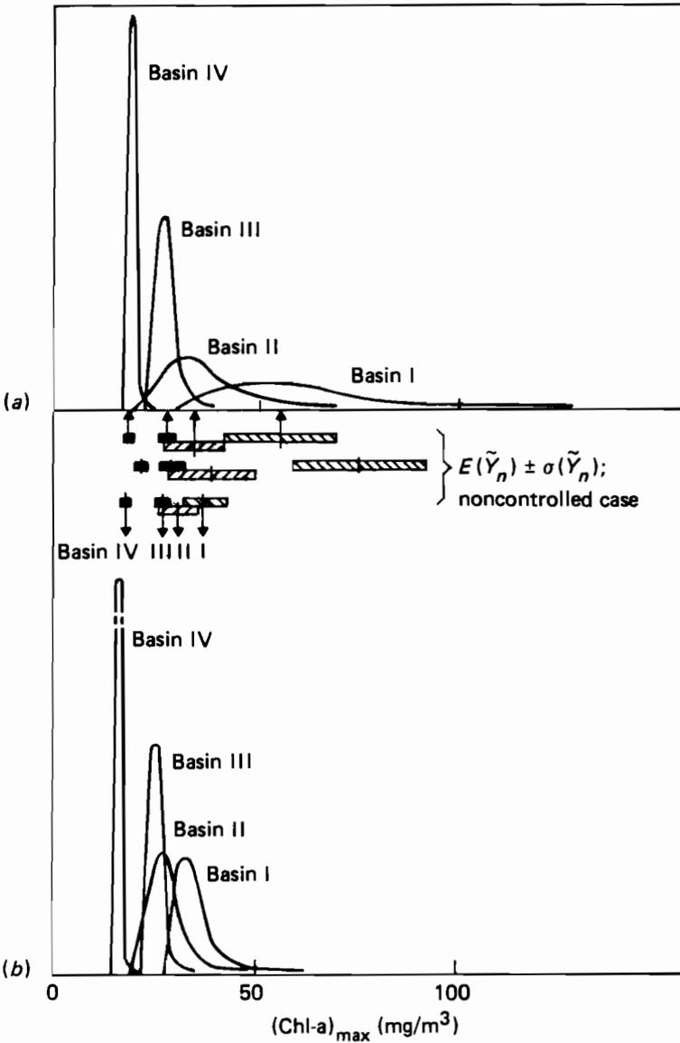
**Figure 4.16.** Probability density functions for two situations (a)  $C_{\text{TA}} = 2.5 \times 10^7$  Ft/yr, and (b)  $C_{\text{TA}} = 20 \times 10^7$  Ft/yr (from 1000 Monte Carlo simulations).
