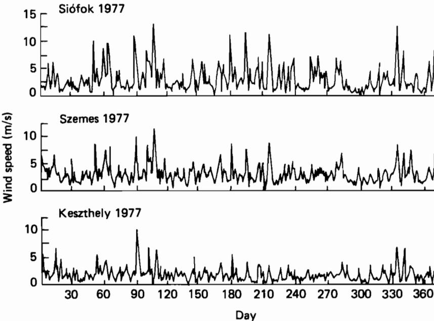
**Figure 9.6.** Comparison of observed daily average wind speeds at Siófok, Szemes, and Keszthely, 1977 (see Figure 9.4 for measurement station locations).
