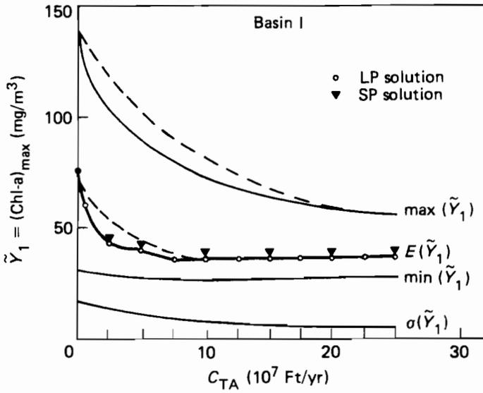
**Figure 4.12.** Water quality as a function of the total annual cost  $C_{TA}$  (solutions obtained from LP and SP models). — basic case; --- with prescribed effluent standard ( $2 \text{ g/m}^3$ ).
