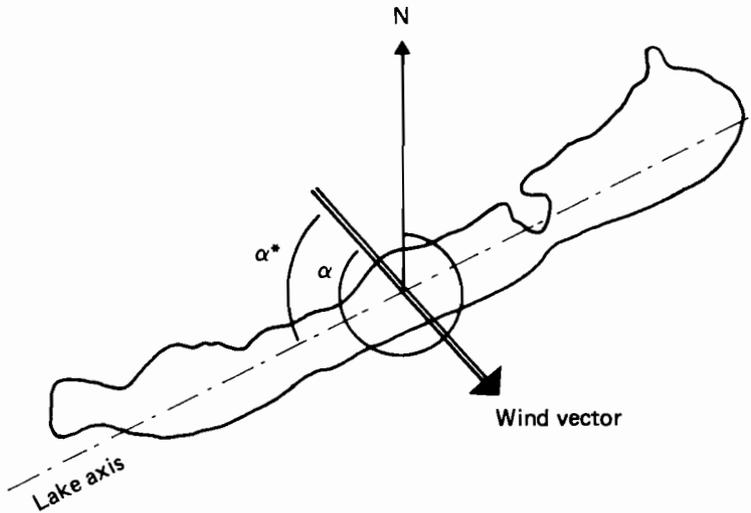
**Figure 9.14.** Definition sketch for wind direction measurements.
