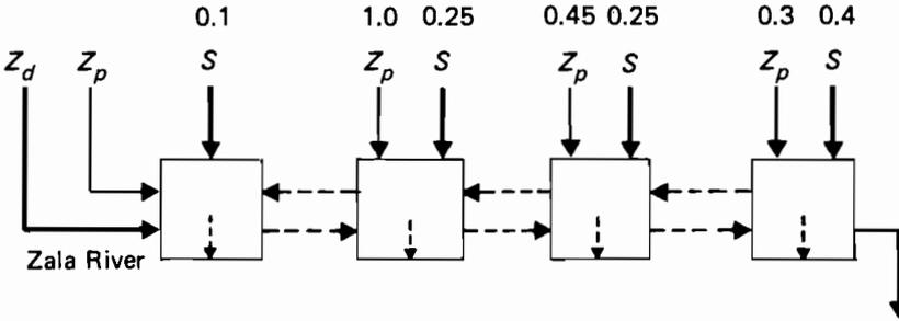
**Figure 11.4.** P load distributions. *S*, sewage;  $Z_p$ , Zala particulate P;  $Z_d$ , Zala dissolved P.
