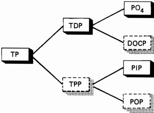
**Figure 11.2.** Reported P fractions for Lake Balaton. Direct measurements (solid boxes): TP, total P; TDP, total dissolved P;  $PO_4$ , orthophosphate; PIP, particulate inorganic P. Calculated (dotted boxes): TPP, total particulate P; DOCP, dissolved organic and condensed P; POP, particulate organic P.
