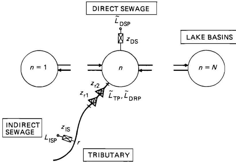
**Figure 4.8.** Development of the nutrient load model NLMP2.  $\tilde{L}_{TP}$ , total P load of tributaries;  $\tilde{L}_{DRP}$ , dissolved reactive P load of tributaries;  $L_{DSP}$ , direct sewage P load (considered deterministic);  $L_{ISP}$ , indirect sewage P load (considered deterministic).
