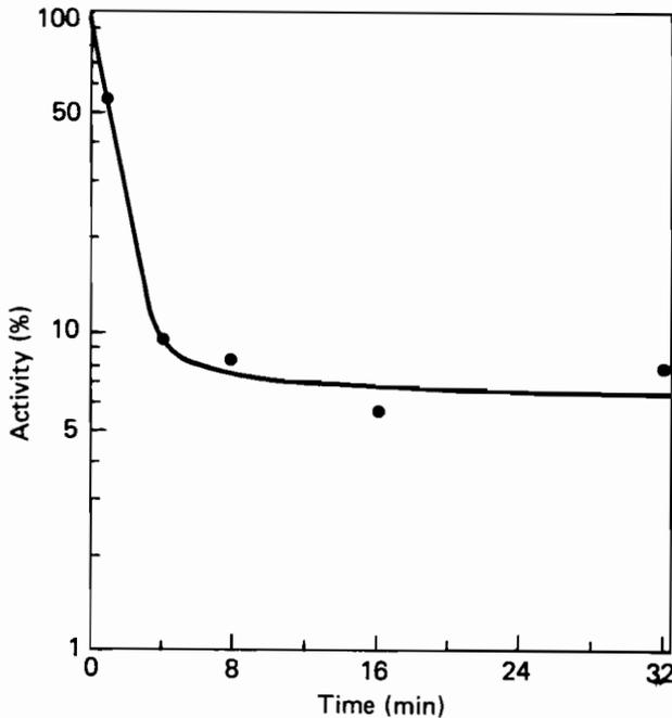
**Figure 8.9.** Decrease in radioactivity in solution after addition of  $^{32}\text{P}\text{O}_4^{3-}$  to a sample of lake water.
