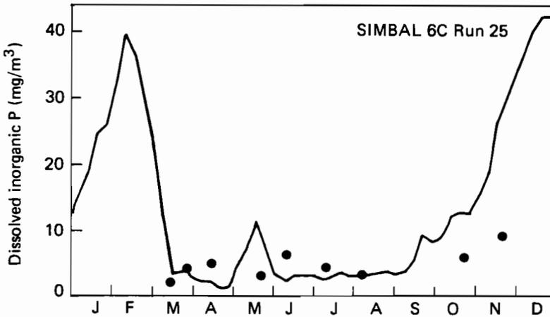
**Figure 11.7.** Typical result for model I. Comparison of simulation (solid line) with measurements (dots) for dissolved inorganic P in the Keszthely basin (basin I).
