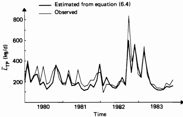
**Figure 6.8.** Validation of the regression model with the inclusion of the suspended solids load for the Zala River.
