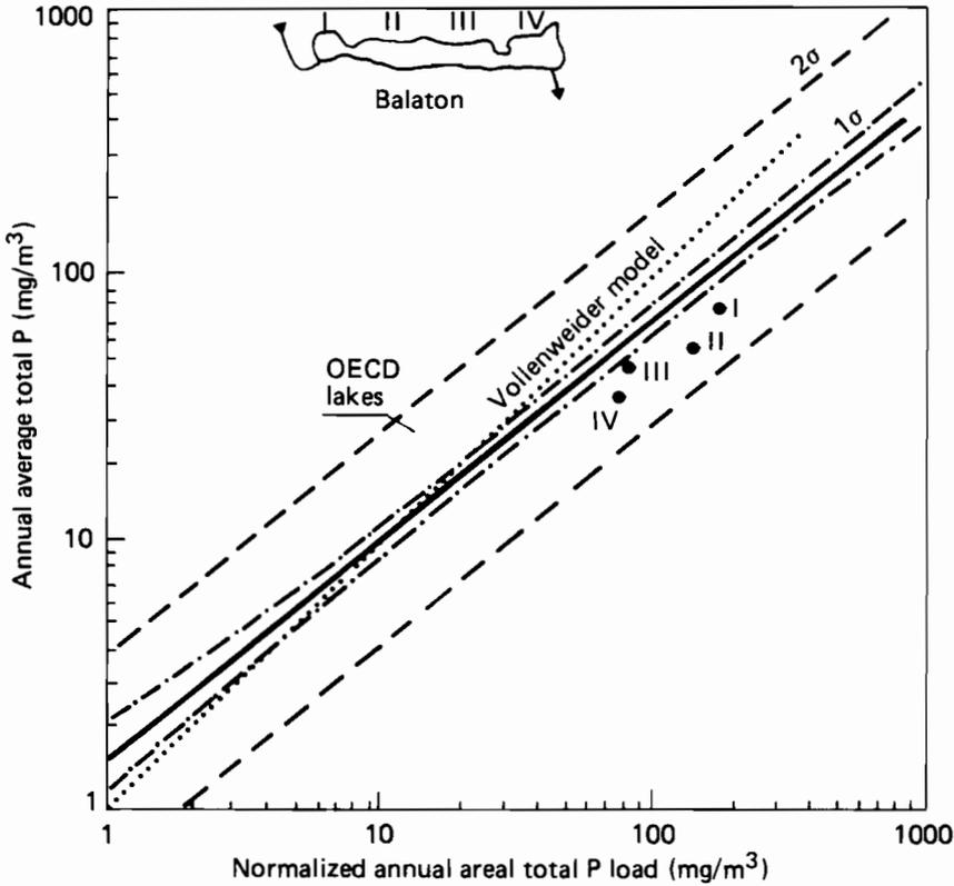
**Figure 3.1.** Empirical relationship between annual average total P concentration and normalized load for OECD lakes. — OECD best fit; - - - 1 $\sigma$  and - - - 2 $\sigma$  boundaries; .... Vollenweider model line [equation (3.1)]; • the four Balaton basins.
