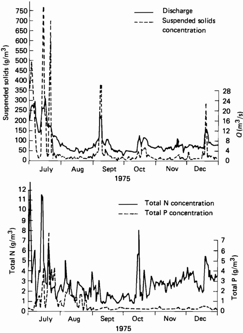
**Figure 14.2.** (a) Discharge and concentrations of suspended solids, total P, and total N for the Zala River, Fenékpuszta, 1975.
