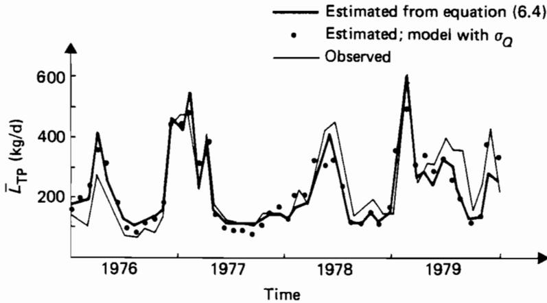
**Figure 6.6.** Calibration of the regression model with the inclusion of the suspended solids load for the Zala River.
