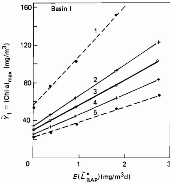
**Figure 4.7.** Aggregated lake eutrophication model: stochastic version. 3, mean; 2 and 4,  $\pm$  standard deviation; 1 and 5, extremes;  $E$ , operator of expectation.
