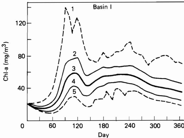
**Figure 4.5.** Influence of natural and controllable factors on water quality. 3, mean; 2 and 4,  $\pm$  standard deviation; 1 and 5, extremes (from 200 Monte Carlo simulations).
