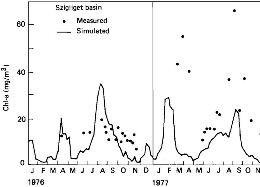
**Figure 12.3.** Measured and simulated Chl-a concentrations in Basin II (Szigliget basin), 1976–77.
