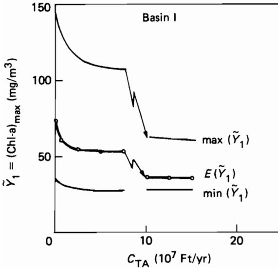
**Figure 4.17.** Model solution for capital recovery factor  $q = 0.05$  for reservoirs and  $0.1$  for sewage treatment plants.
