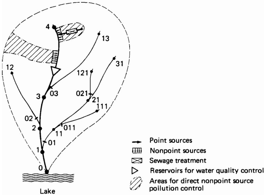
**Figure 6.10.** Development of nutrient load models for planning.
