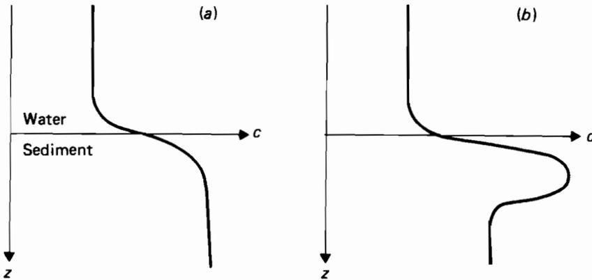
**Figure 7.3.** Concentration gradients in the sediments near the surface.
