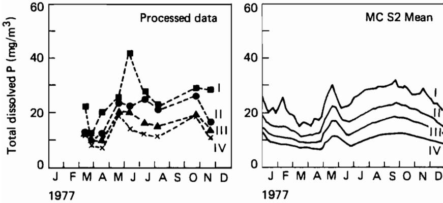
**Figure 11.3. (b)** Total dissolved P data (*left*) and average of the seven behavioral runs (series 2) for the four basins.
