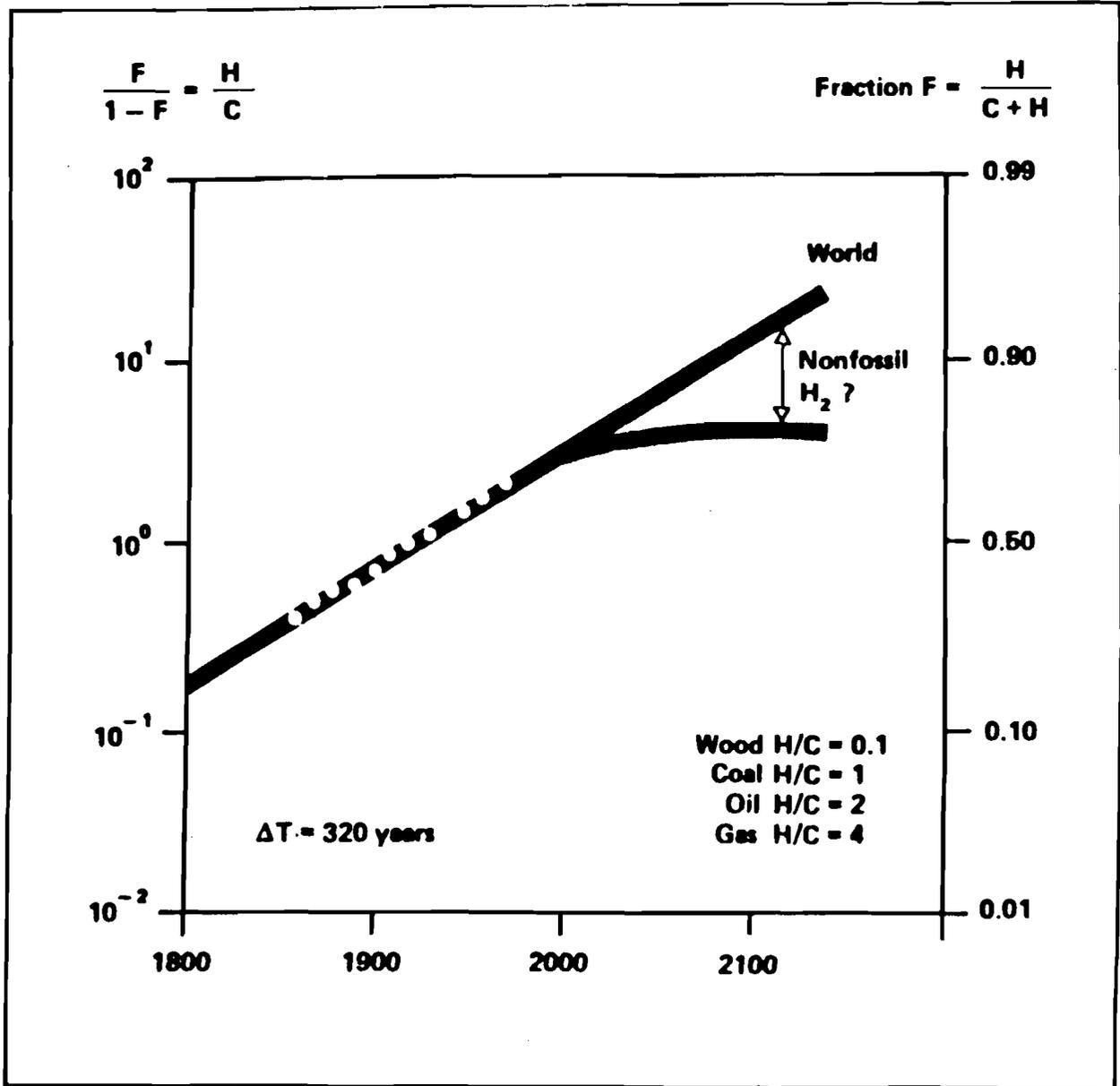
Figure 16. Evolution of the ratio of hydrogen (H) to carbon (C) in the world fuel mix. The figure for wood refers to dry wood suitable for energy generation. If the progression is to continue beyond methane, production of hydrogen fuel without fossil energy or with carbon removal is required (Marchetti, 1985).
