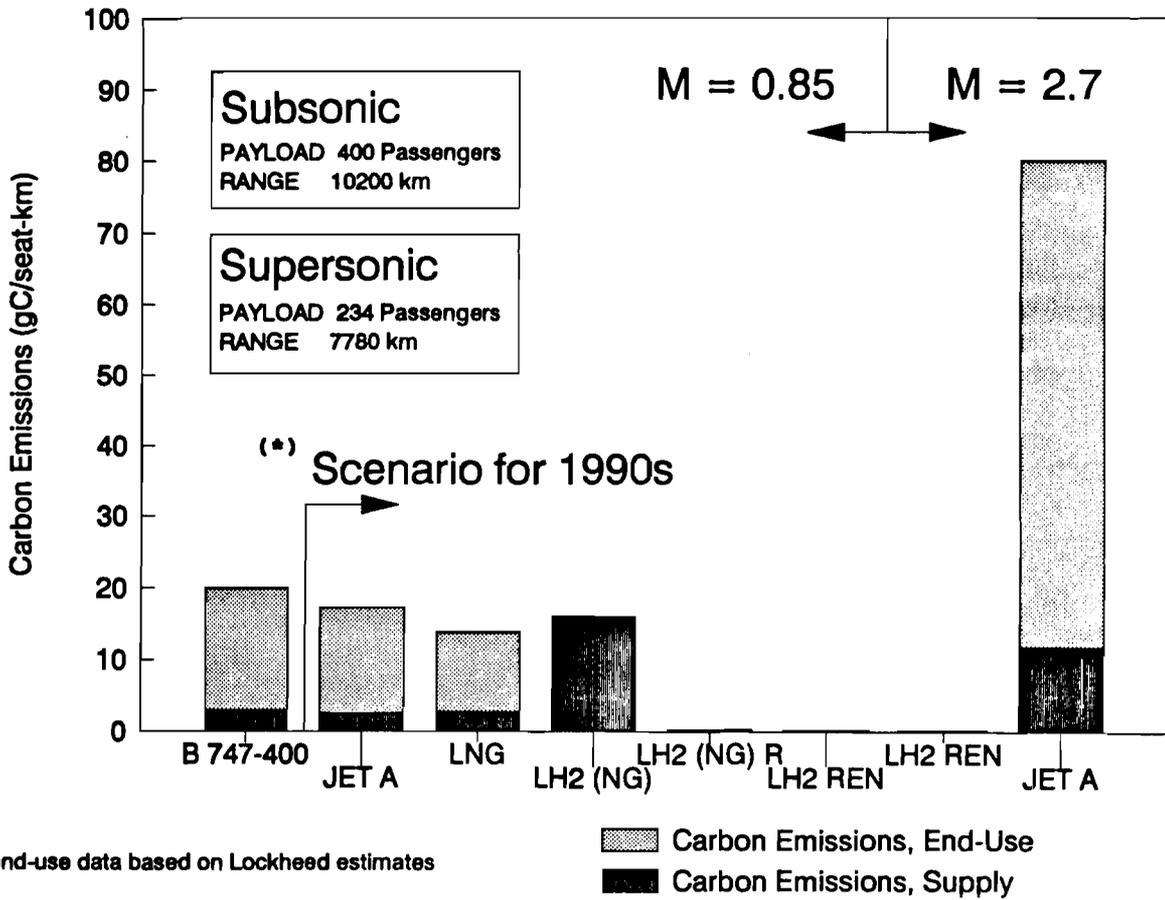
Figure 19. Carbon emissions for different transportation fuels. Boeing 747-400 powered by Jet A. Advanced subsonic aircraft: Jet A, LNG: liquefied natural gas, LH2 (NG) and LH2 (NG) R: liquefied hydrogen derived from natural gas by autothermal steam reforming and subsequent shift reaction of natural gas with carbon removal of the latter (R), LH2 (REN): liquid hydrogen from renewables. Supersonic aircraft powered by liquid hydrogen and Jet A.
