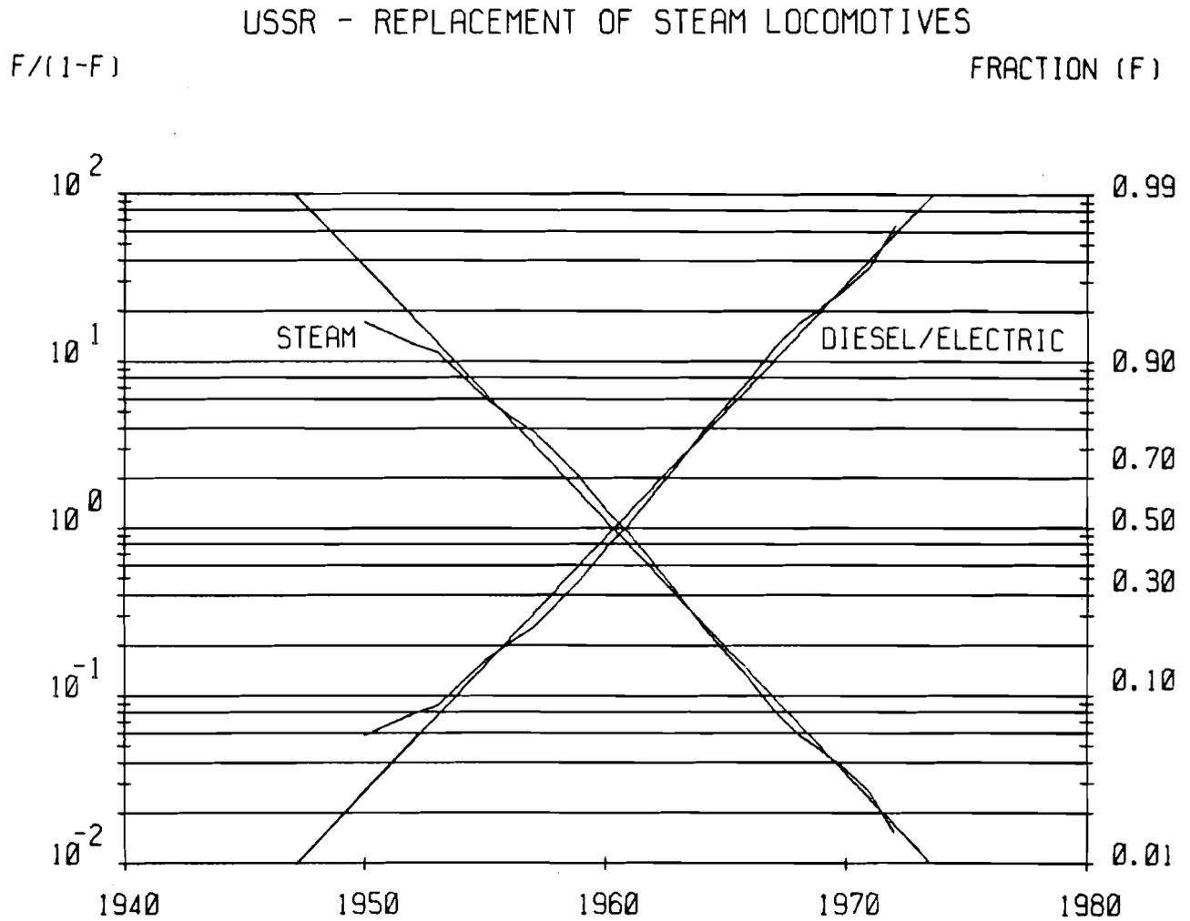
Figure 13. Substitution of steam by diesel and electric locomotives in the USSR. The shares of the two classes of locomotives are given in percent of the total number of locomotives in use. The replacement process lasted about two decades. Similar duration for replacement of the rolling stock and locomotives can also be observed for other countries.
