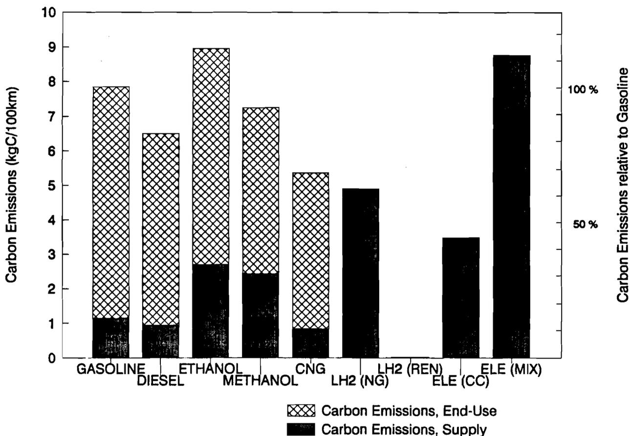
Figure 18. Carbon emissions for different transportation fuels. Gasoline, diesel, CNG: compressed natural gas, ethanol is assumed to be produced from sugarcane, methanol and hydrogen derived from natural gas (SR-NG: autothermal steam re-forming of natural gas), LH2 (REN): liquid hydrogen from renewables, ELE (CC): electric vehicle with electricity from a natural gas fired combined cycle power plant and ELE (MIX) from an average power plant with the current US fuel mix.
