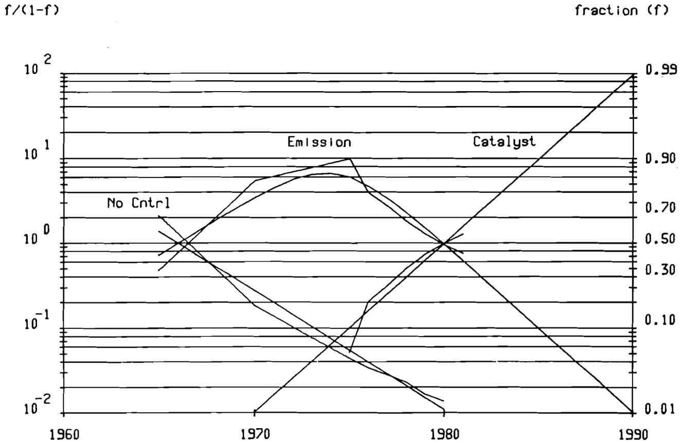
Figure 12. Substitution of automobiles with a catalytic converter and emission controls for older vehicles without any emission restraints in the US. The shares of each of three classes of vehicles are given in percent of the total fleet. The replacement of older vehicles by new types lasted about two decades in both cases. Similar duration of automobile fleet replacements can be also observed for other countries.
