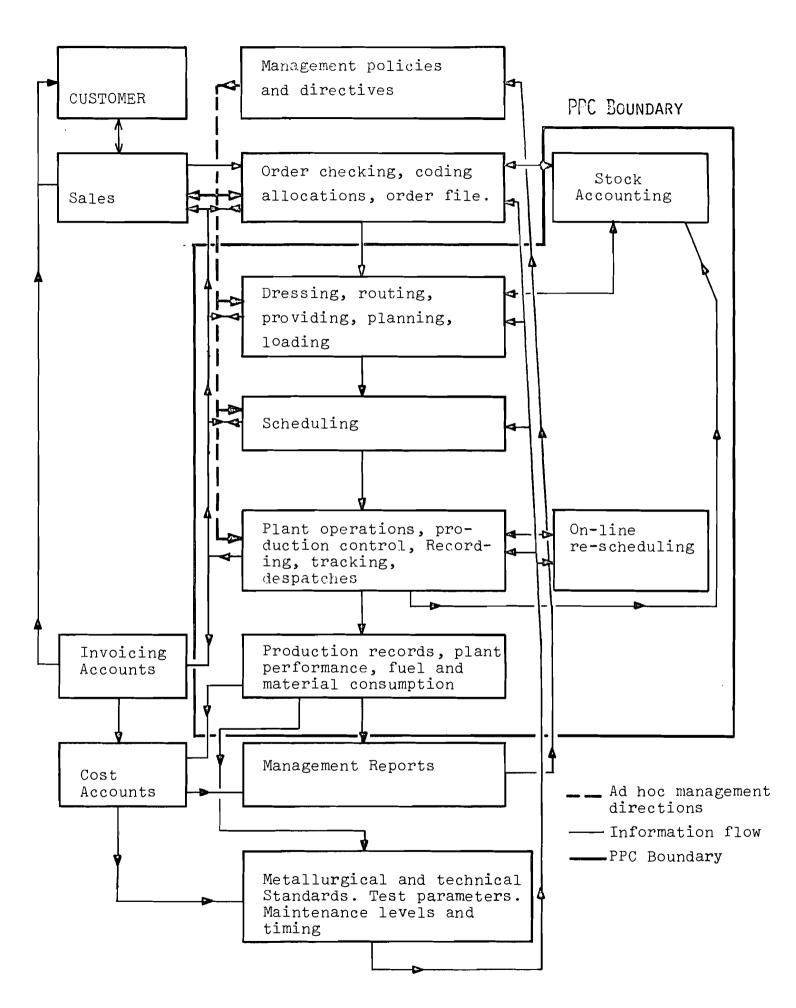
Fig. 1. PPC System - Main Components and Information Flows.
