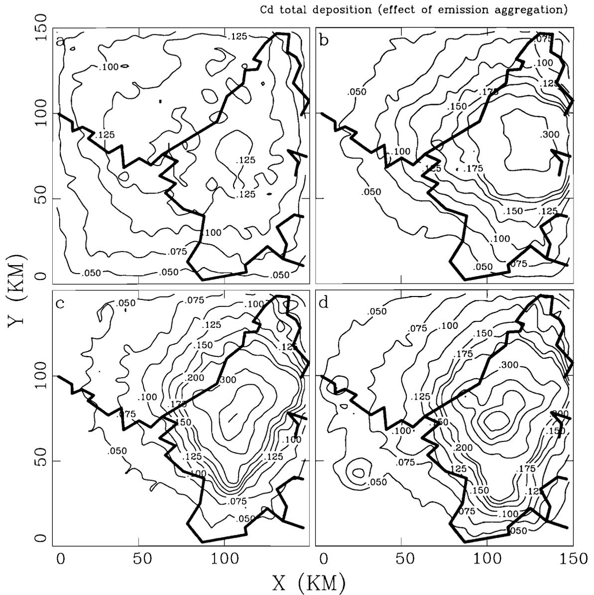
Figure 13: Total deposition of Cd [ $mg/m^2$ ] in 1992 calculated with different aggregation level of emission sources: a) a single  $150 \times 150 \times 0.5$  km volume source, b) a grid of  $50 \times 150 \times 0.5$  km volume sources, c) a grid of  $0 \times 10 \times 0.5$  km volume sources, d) a grid of  $5 \times 5 \times 0.05$  km volume sources and major point sources (reference simulation)
