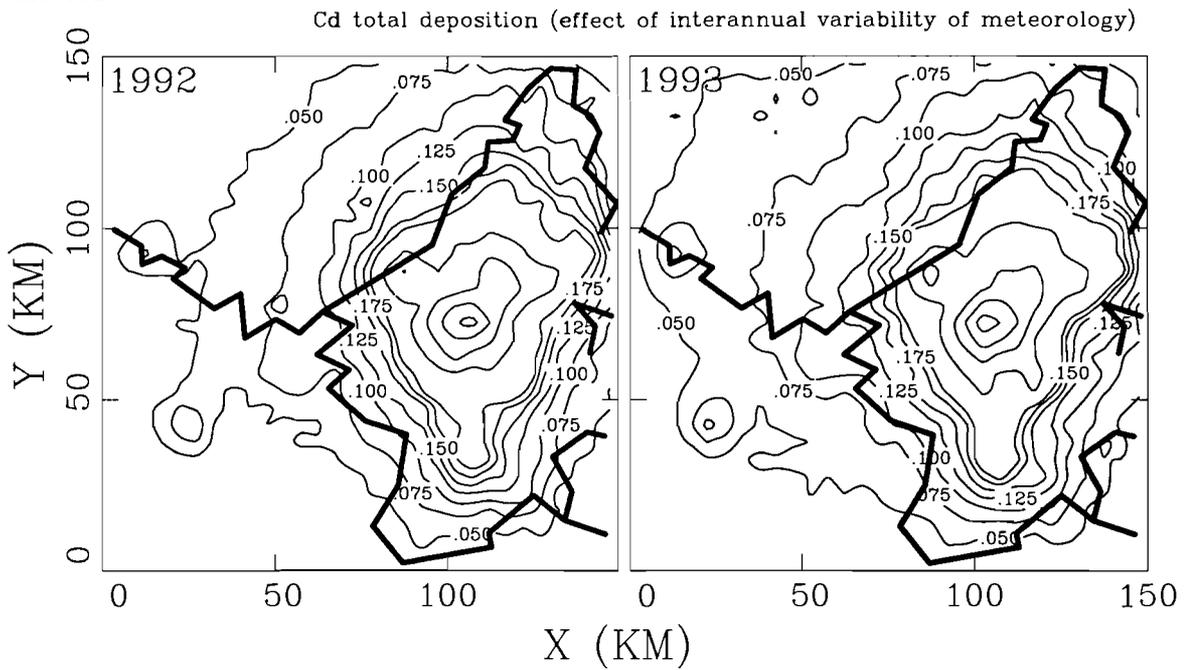
Figure 15: Total deposition of Cd [ $mg/m^2$ ] during nine months (April-December) of 1992 (left) and the same period of 1993 (right) calculated for the emission sources aggregated as in the reference simulation
