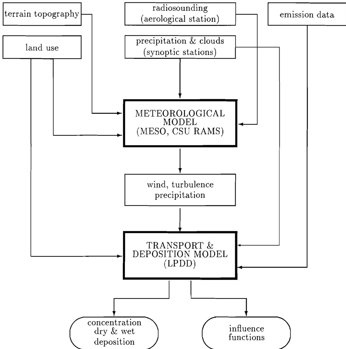
Figure 1: Data flow between mesoscale meteorological and transport/deposition models
