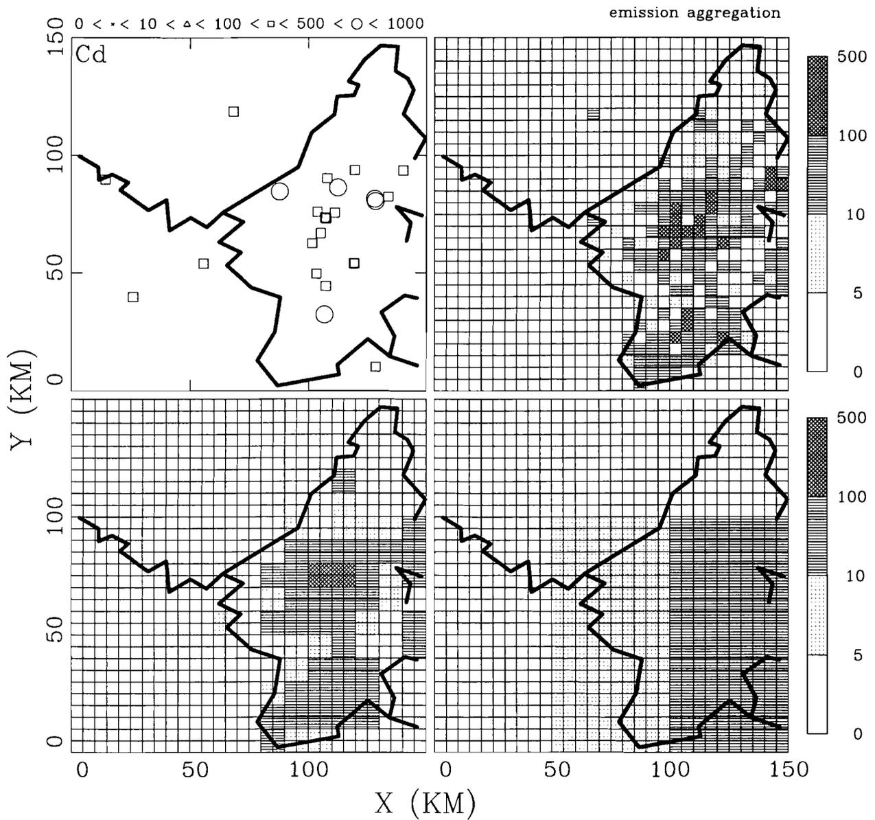
Figure 12: Aggregation of emission sources [kg/year] for Cd: a) major point sources and b) 5×5×0.05 km volume sources used in the reference simulation, c) 10×10×0.5 km volume sources, d) 50×50×0.5 km volume sources
