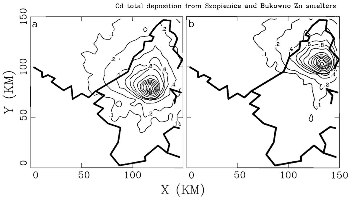
Figure 17: Total deposition of Cd [ $mg/m^2$ ] in 1992 calculated for two point sources located in (a) Szopienice and (b) Bukowno zinc smelters with the emission rate increased to 25  $ton/year$  of Cd each
