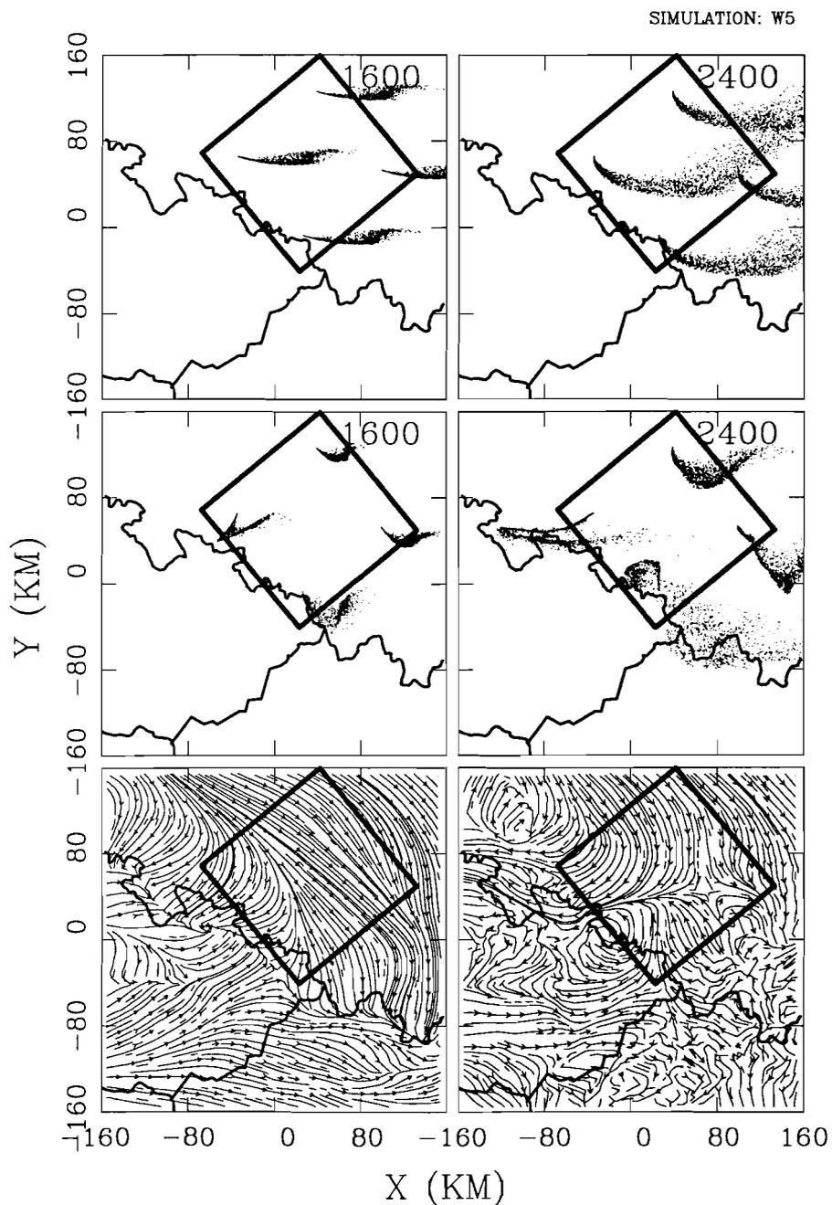
Figure 19: Plumes of passive tracer simulated using 1-dimensional (top) and 3-dimensional meteorological fields ( $\Delta x = 5$  km), and streamlines (bottom) at 200 m model level derived from the same 3-dimensional meteorological simulation at 16:00 (left) and 24:00 (right) GMT for  $U_g = 5$  m/s and  $V_g = 0$  m/s.
