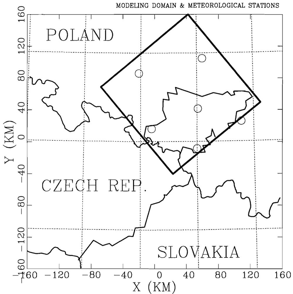
Figure 3: Modeling domain used in 3-dimensional meteorological simulations. The  $150 \times 150$  km square, (25,19) cell of the EMEP grid, covering the Katowice province in the southern Poland is the deposition modeling domain. Meteorological stations used to derive precipitation and cloud cover fields are marked by circles.
