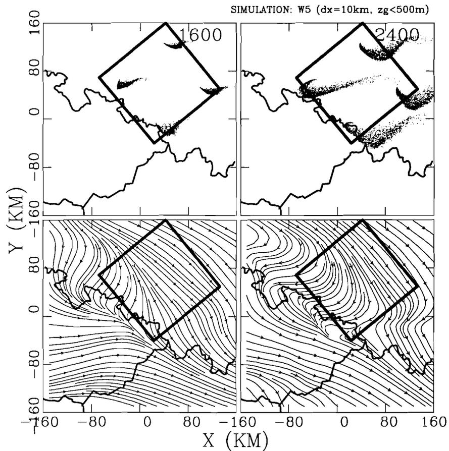
Figure 29: Plumes of passive tracer (top) and streamlines at 200 m model level (bottom) calculated with the aid 3-dimensional meteorological fields with a coarser horizontal resolution ( $\Delta x = 10 \text{ km}$ ) and terrain elevation reduced to 500 m above sea level at 16:00 (left) and 24:00 (right) GMT for  $U_g = 5 \text{ m/s}$  and  $V_g = 0 \text{ m/s}$ .
