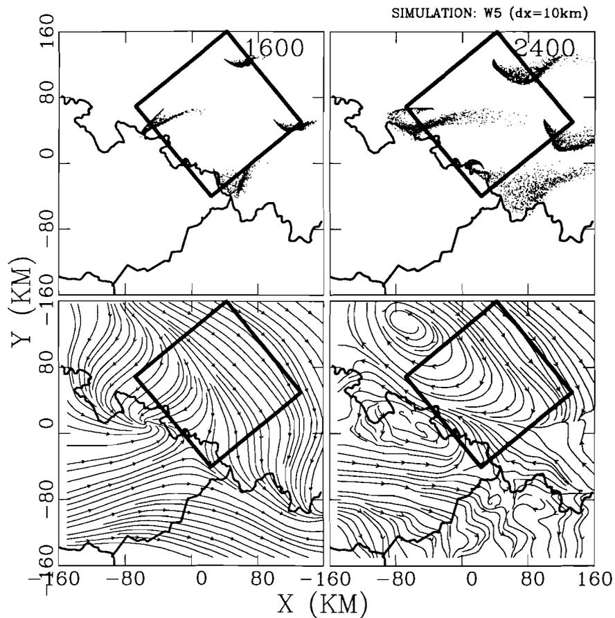
Figure 27: Plumes of passive tracer (top) and streamlines at 200 m model level (bottom) calculated with the aid 3-dimensional meteorological fields with a coarser horizontal resolution ( $\Delta x = 10 \text{ km}$ ) at 16:00 (left) and 24:00 (right) GMT for  $U_g = 5 \text{ m/s}$  and  $V_g = 0 \text{ m/s}$ .
