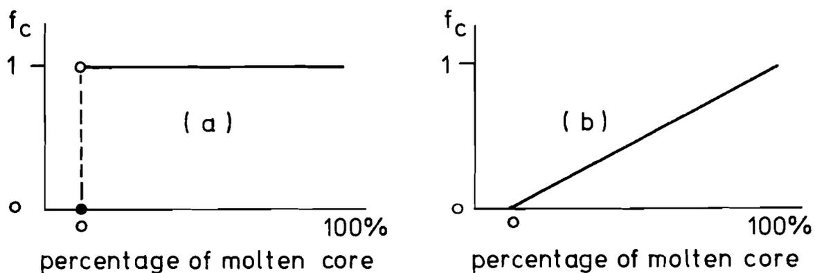
Fig. 4.2 (a): Characteristic function for the model in Reference (8)
