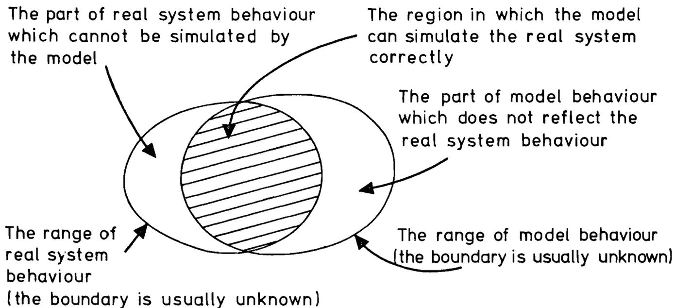
Fig. 4.2 The gap between the real system and the model
