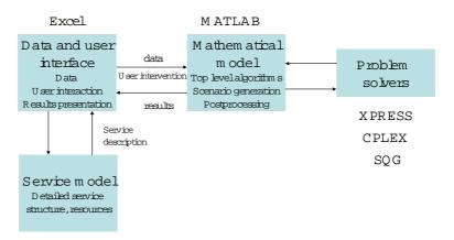
Figure 3: Architecture of decision support system for evaluation of business models of service provision
