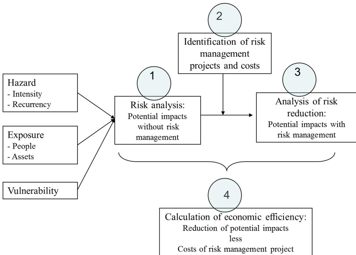
**Figure 1: Risk-based methodology for assessing the efficiency of disaster risk reduction**
