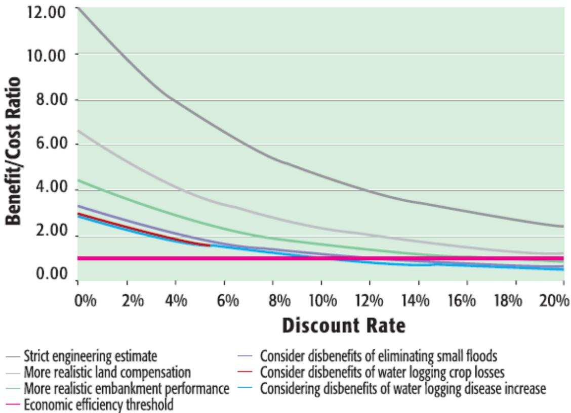
Figure 16: Evaluation of the performance of embankments along the Rohini River basin in India
