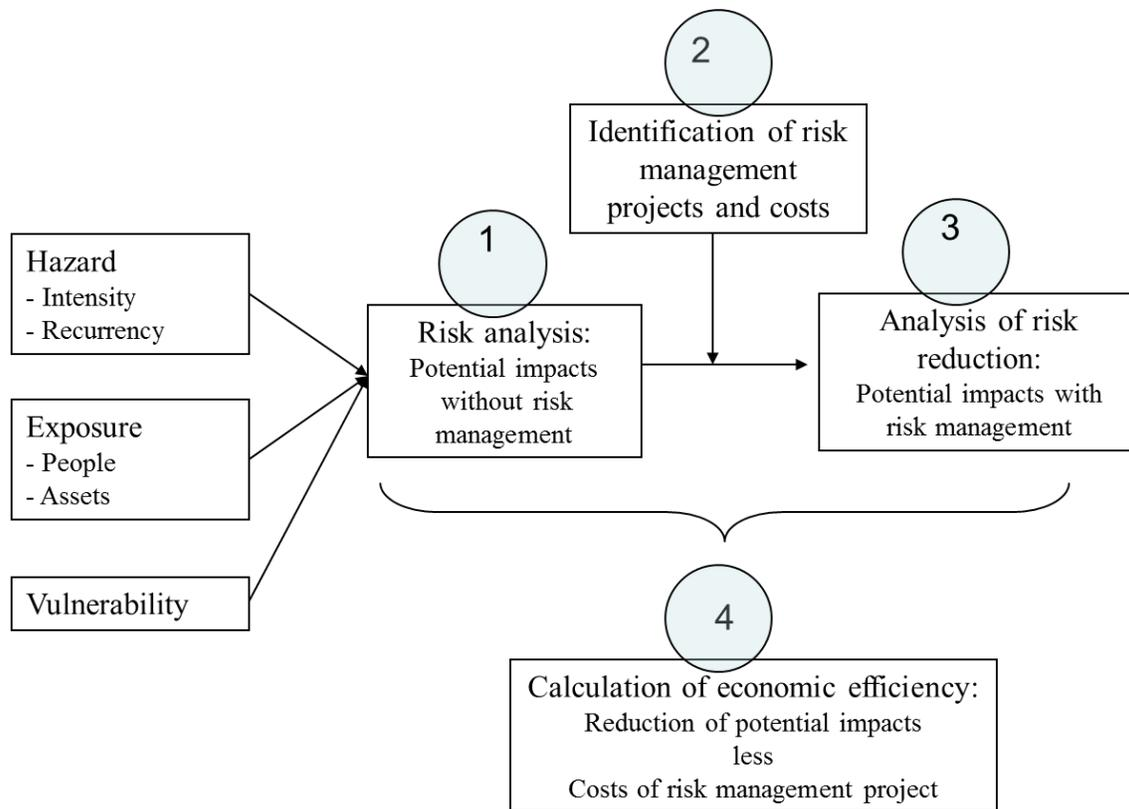
**Figure 7: Risk-based methodology for conducting CBA of disaster risk reduction**
