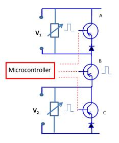
Figure 3: Sub-module with microcontroller and switching transistors.
