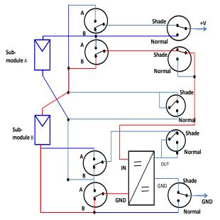
Figure 5: Schematic of the voltage compensation circuit.
