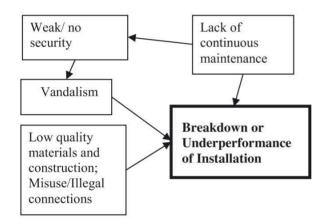
Figure 4: Interconnected factors leading to breakdown of Installation.
