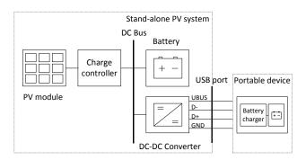
Figure 1: Stand-alone PV system with USB charging port configuration.
