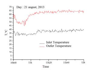
Figure 5: Dryer inlet and outlet air temperatures in case 25 % apertures opening
