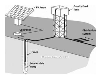
Figure 1: PV pumping schematic
