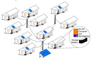
Figure 7: Distributed generation and distributed storage
