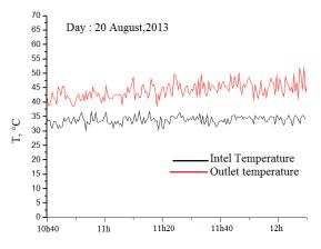
Figure 4: Dryer inlet and outlet air temperatures in case of 35 % apertures opening
