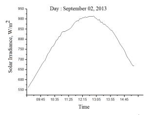
Figure 8: Measured global solar irradiance for the 2<sup>nd</sup> of September 2013
