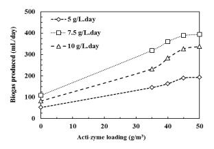
Figure 2: Biogas produced over varying Acti-zyme and sewage sludge loading.
