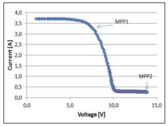
Figure 6: Two peaks in the I–V curve produced by hard shading a single cell.
