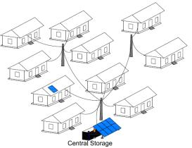
Figure 4: Centralized panel and centralized storage
