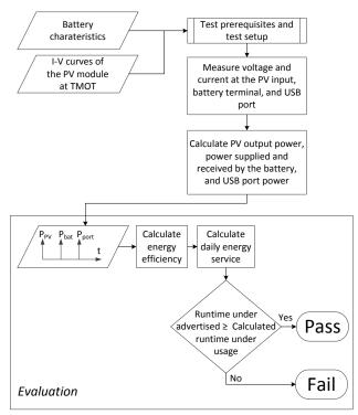
Figure 5: Energy-based test flow chart.
