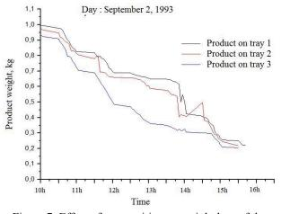
Figure 7: Effect of tray position on weight loss of the product as function of time for partially cloudy sky
