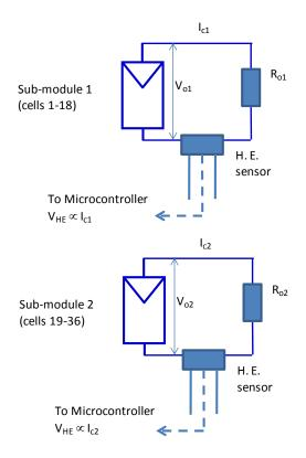
Figure 4: Shade detection circuit
