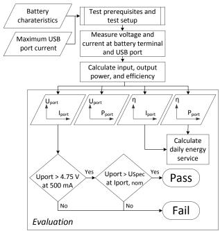
Figure 3: Steady state test flow chart.
