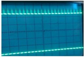
Figure 3: Output of the compact DC-DC converter without rectifier on analog oscilloscope [Scale: 5V/unit and 25 micro seconds].
