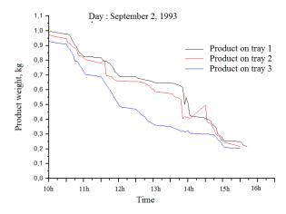
Figure 9: Effect of tray position on weight loss of the product as function of time for clear sky
