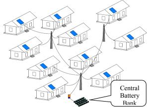
Figure 6: Distributed generation and centralized storage
