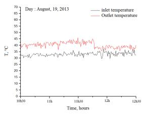
Figure 3: Dryer inlet and outlet air temperatures in case of totally opened apertures
