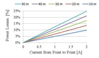
Figure 2: Power Losses due to voltage drop and droop
