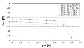
Figure 6: USB charging port voltage over current characteristic at different battery voltages.
