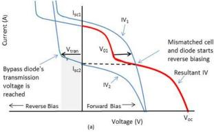
Figure 1: I–V characteristic of partially shaded module with two bypass diodes (Source: Vorster & Dyke, 2005)
