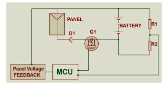
Figure 2: Logical block diagram for solar charge controller of compact DC-DC converter.
