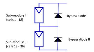
Figure 2: Conventional PV module
