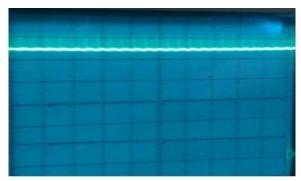
Figure 4: Output of the compact DC-DC converter with rectifer and LC filter on analog oscilloscope [Scale: 5V/unit and 25 micro seconds].
