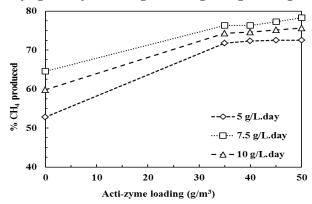
Figure 3: Bio-methane composition in sewage sludge at varying Acti-zyme loading and sewage sludge loading.
