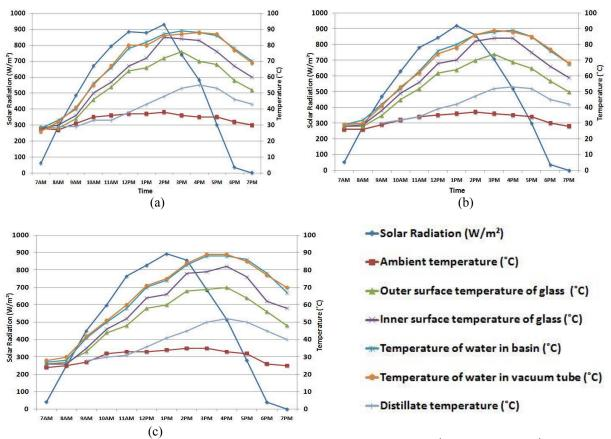
Figure 3: Hourly variations of solar radiation and various temperatures on (a) 11<sup>th</sup> May 2014 (b) 10<sup>th</sup> June 2014 and (c) 12<sup>th</sup> July 2014, for Bangalore location
