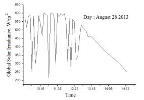
Figure 6: Measured global solar irradiance for the 28th of August 2013
