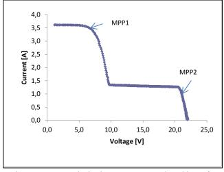
Figure 7: Two peaks in the I–V curve produced by soft shading
