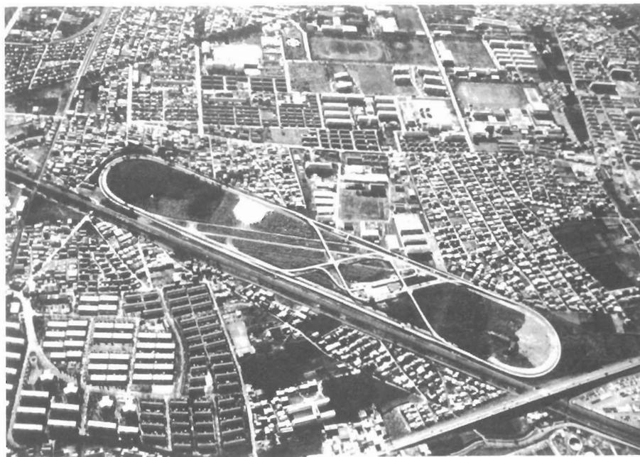
FIGURE 19.1 CVS Higashimurayama experimental site, which is 800 m long and 160 m wide. The white line in the photograph shows a CVS guideway 4.8 km long. The outer oval-shaped guideway is called superway and the center diamond-shaped part is called path.
