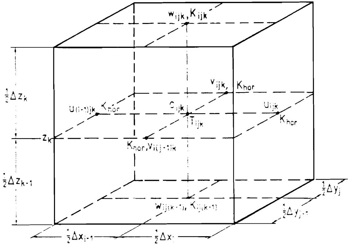
Figure 1. A staggered grid system used by the flux-correction method.
