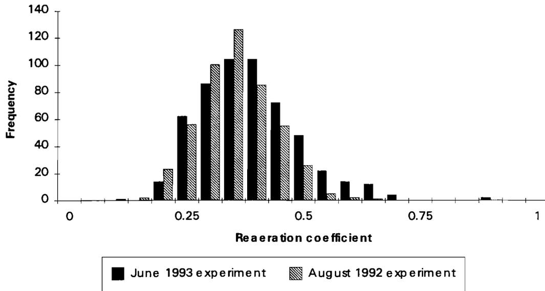
**Figure 10.** The frequency plots for the reaeration coefficient estimation PDFs for the upper stretch of the Nitra River. The June 1993 and August 1992 experiments.
