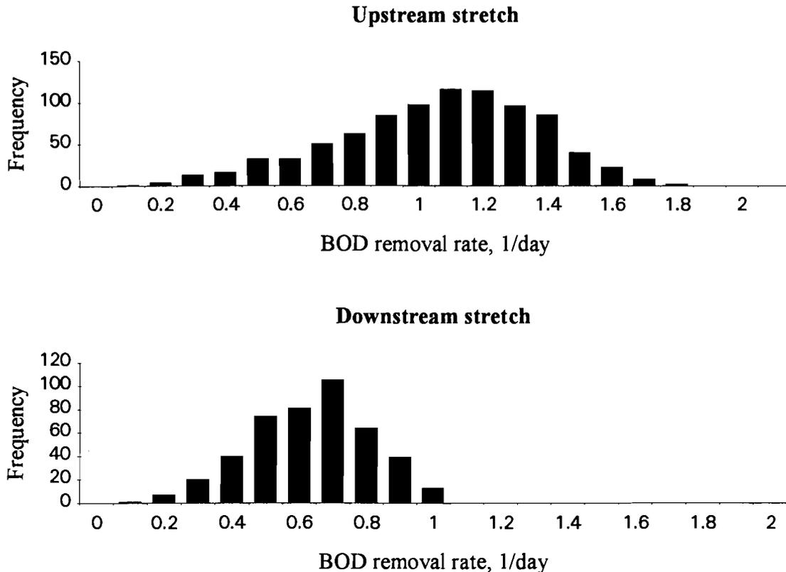
**Figure 3.** Frequency plots for the BOD removal rate in the upstream and downstream stretches of the Nitra River obtained with HSY technique (August 1992 experiment).
