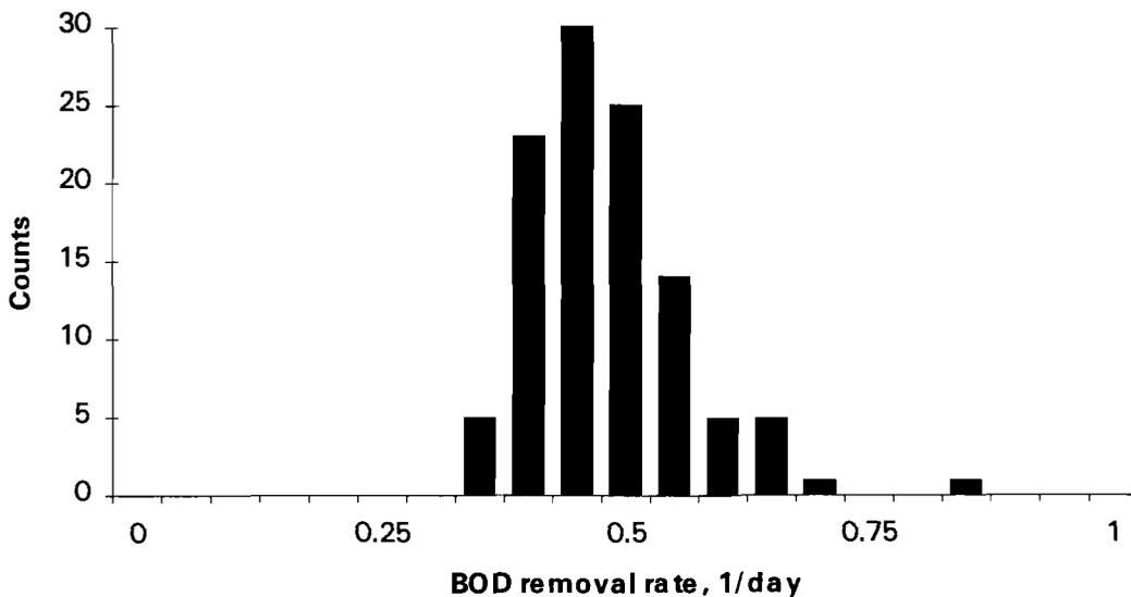
**Figure 9.** Frequency plot for the BOD-5 removal rate estimate for the upper stretch of the Nitra River (the June 1993 experiment).
