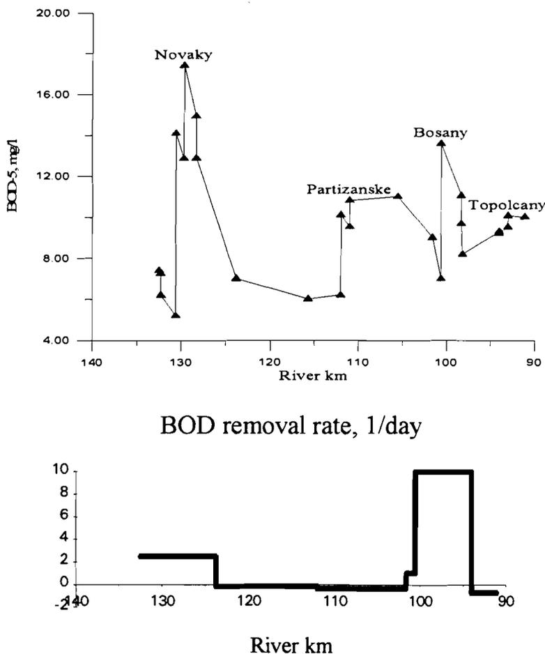
**Figure 1.** Longitudinal profile and the evaluation of the removal rate of BOD-5 (upper part of the Nitra River).
