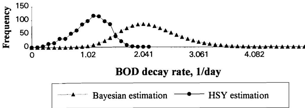
**Figure 8.** Probability density plots for the BOD removal rate obtained from the HSY technique and Bayesian estimation (upper stretch of the Nitra River).
