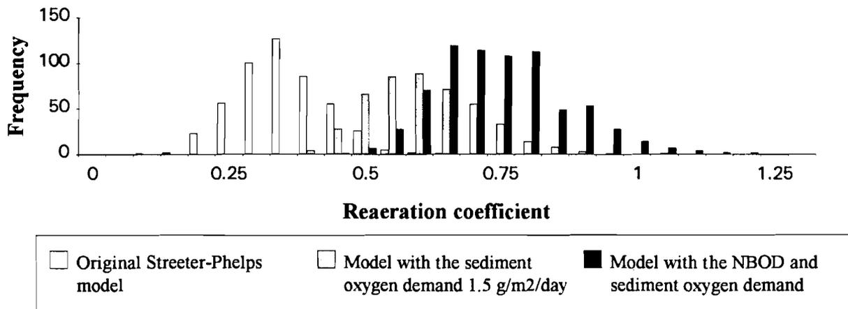
**Figure 4.** Frequency plots for the reaeration coefficient of the three DO water quality models (upper part of the Nitra River).
