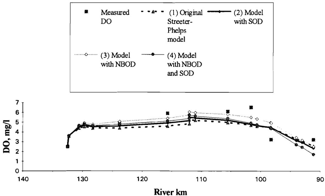
**Figure 6.** Simulation of DO for the upper stretch of the Nitra River by a sequence of calibrated models.
