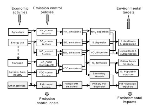
Figure 3.1: A schematic diagram of the information flow in the RAINS model
