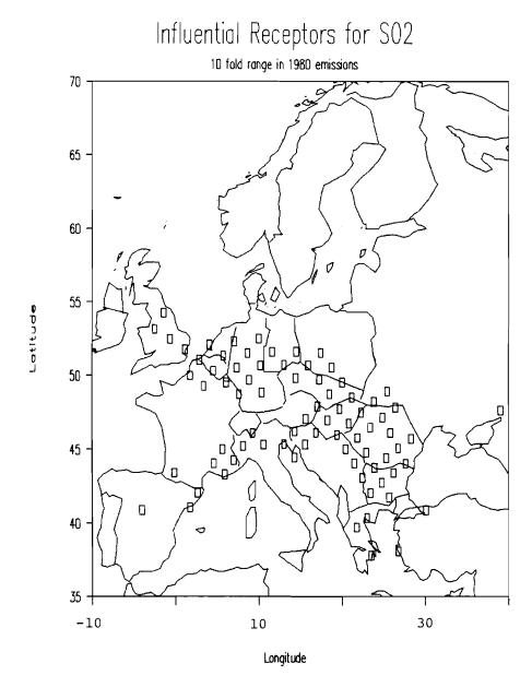
Figure 3b. Locations of influential receptors for  $S0_2$  concentrations for 10-fold range of feasible emissions. Squares indicate receptor locations.
