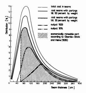
Figure 2. Distribution of the reserves in situ and of the output of the Ruhr coal mining industry 1929 and 1974 according to seam thickness including partings.
