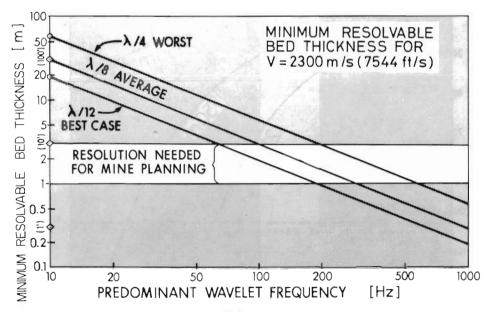
Figure 10. Minimum resolvable coal bed thickness as a function of predominant reflection frequency. Resolution needed for coal mine planning and high quality exploration studies is between 1 and 3 m. For the average one-eighth wavelength detectability criterion this means frequencies between 100 and 300 Hz are required.
