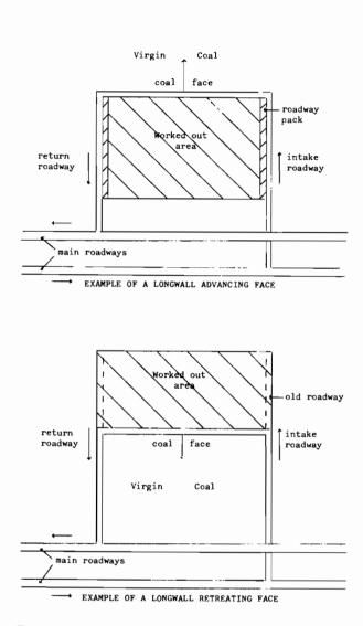
Figure 3. Examples of longwall advancing and retreating faces.
