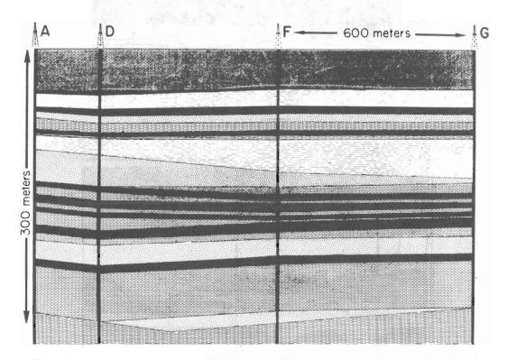
Figure 6. Geological interpretation made by using core hole information only. Without seismic reflection information between holes, simple hole to hole interpolation fails to reveal troublesome problem areas as seen by comparison with Figure 5.
