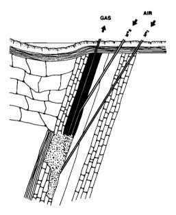
Figure 1. Gasification of a steep seam through inclined boreholes.
