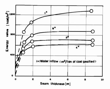
Figure 3. Variation of the heating value of the gas in function of the thickness of the seams and water inflow.
