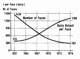
Figure 5. Concentration of underground coal mining operations.
