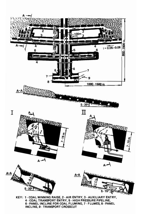
Figure 3. The technology of hydraulic coal mining: I - with hydraulic monitors, II - with mechanical and hydraulic shearers.
