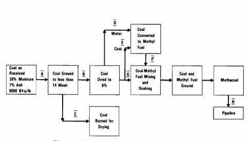
Figure 2. Schematic flow diagram of the Methacoal process.
