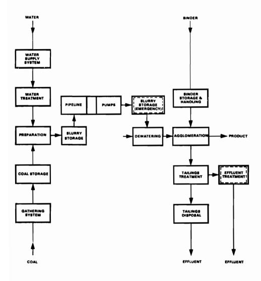
Figure 3. Elements of the complete slurry pipeline system.
