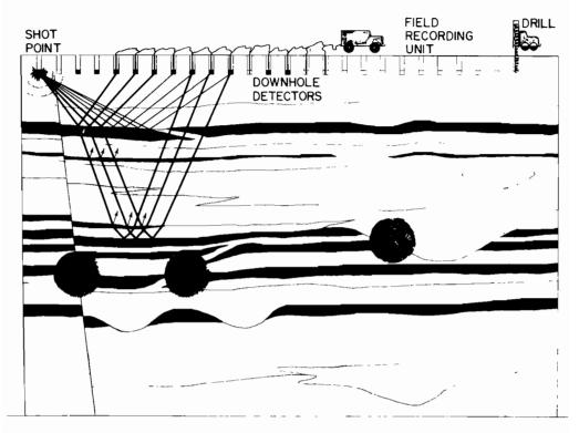
Figure 2. Diagrammatic cross section showing fundamentals of reflection profiling and type of field equipment used. Also illustrated are typical subsurface disturbances such as faults, sand channels and seam pinchouts which can present problems in the extraction of coal.
