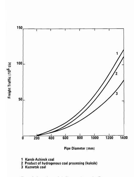
Figure 6. Dependence of pipeline capacity on pipe diameter.
