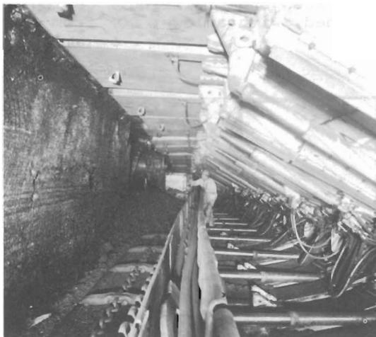
Figure 8. Shield supports.
