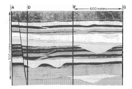
Figure 5. The interpretation derived from the seismic data in Figure 3 with patterns representing different geological formations. Core holes have been added representing a hypothetical coal drilling program which just misses all disturbing features.
