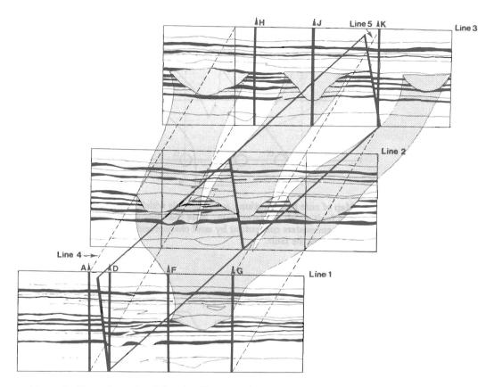
Figure 9. Three dimensional drawing illustrating how seismic cross sections permit tracing of fault planes and sand channels. For clarity only east-west lines are shown, but north-south lines would appear in similar manner fixing subsurface locations.
