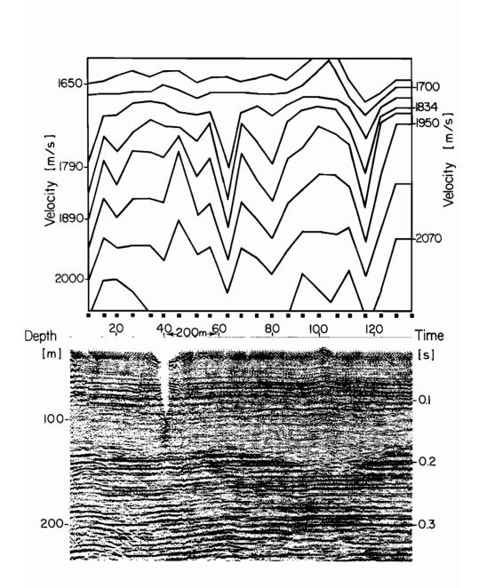
Figure 15. Constant velocity graph positioned over data from which it was derived. Horizontal scales are approximately the same for both graph and section. Note correspondence of low velocity anomalies and old river channel as well as near surface fault.
