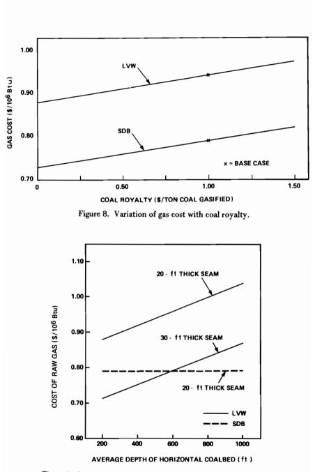
Figure 9. Estimated raw gas costs for LVW gasification related to coal bed geometry and compared to the SDB case shown.
