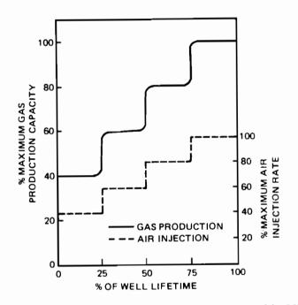
Figure 4. Gas production and air injection patterns assumed for LVW case (the same units are implied for air and gas rates).
