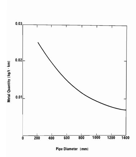
Figure 2. Dependence of metal quantity on pipe diameter.
