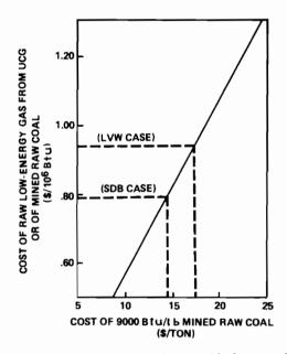
Figure 10. Comparison of mined raw coal costs with the cost of raw lowenergy gas from UCG on an equal energy basis (assuming 9000 Btu/lb coal heating value).
