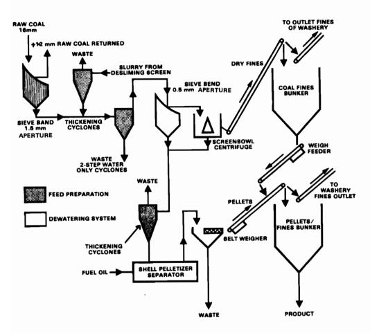
Figure 6. Process flow scheme of Fryston pilot plant.
