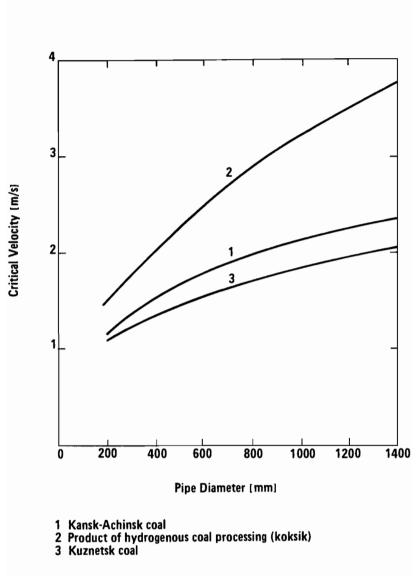
Figure 1. Dependence of critical velocity on pipe diameter.
