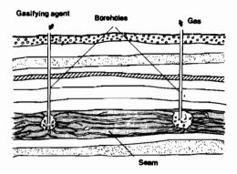
Figure 2. Underground gasification by filtration.
