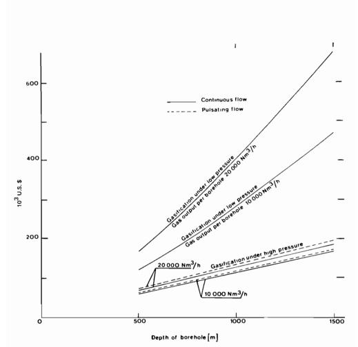
Figure 6. Evolution of the cost of the boreholes in function of the pressure and the depth.
