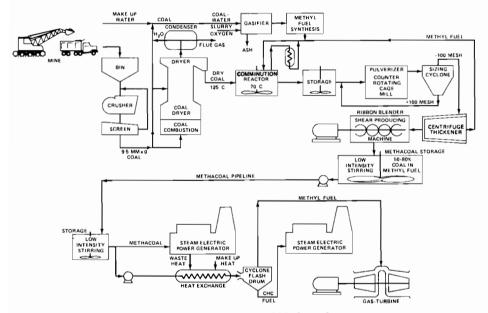
Figure 1. Simplified diagram of Methacoal concept.
