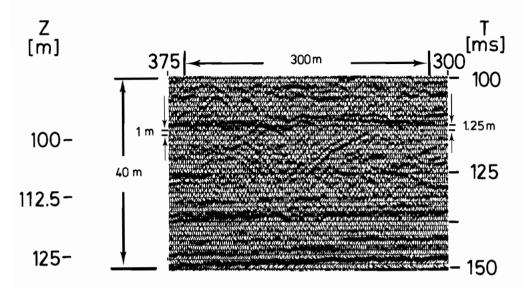
Figure 17. Example of high resolution data from the new techniques showing fine stratigraphic detail within individual beds. Temporal sampling is 1/4 ms while spatial sampling is 5 m, or 16-1/2 ft. Horizontal lines are approximately 1 m apart at typical coal section velocities.
