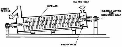
Figure 5. Section through Shell Pelletizer Separator (SPS).
