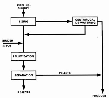
Figure 4. Process scheme for coal slurry dewatering.
