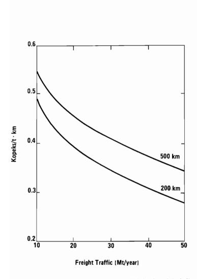
Figure 7. Cost of hydraulic transport of Kansk-Achinsk coal (including preparation for transport).
