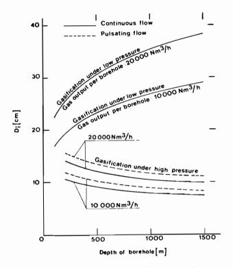
Figure 5. Evolution of the useful diameter of the boreholes in function of the pressure and the depth.
