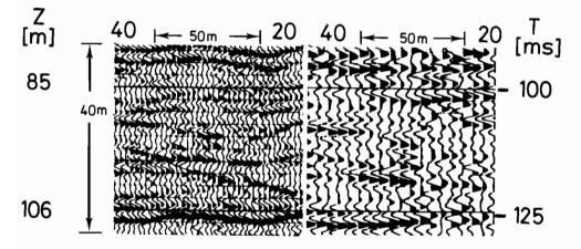
Figure 14. The increased resolution obtained when temporal and spatial sample rates are doubled. Note reflection periods of approximately 1 ms (1000 Hz) on data to left.
