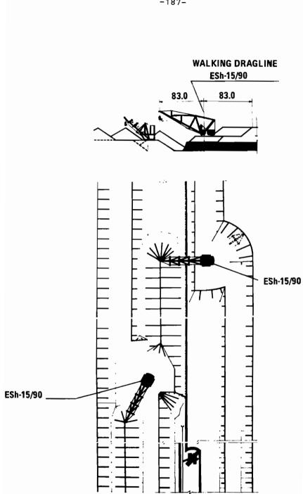
Figure 2. The transportless technology of mining with walking draglines.
