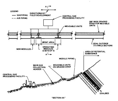
Figure 7. The conceptual SDB gasification site (not to scale).
