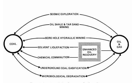
Figure 2. Some interrelations between coal and petroleum extraction technologies.
