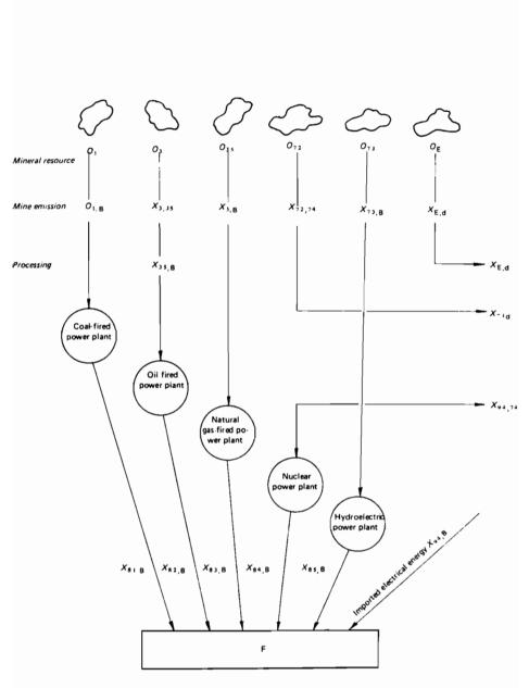
Figure 2. Power generating systems with different energy carriers.
