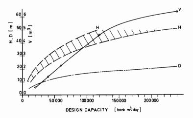
Figure 1. Bucket volume, V, digging height, H, and wheel diameter, D, for various design capacities.
