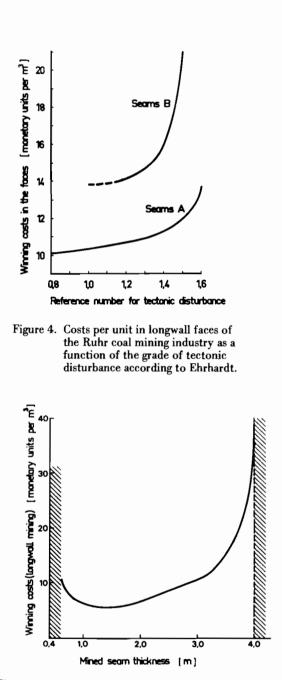
Figure 5. Costs per unit in longwall faces of the Ruhr coal mining industry as a function of mined seam thickness in single-slice mining according to Steinbauer.
