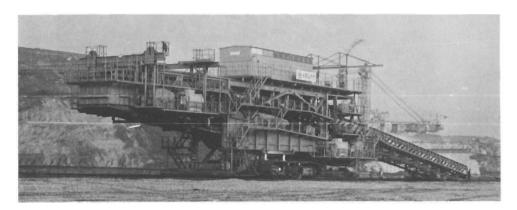
Figure 3. Drive terminal for conveyor system.
