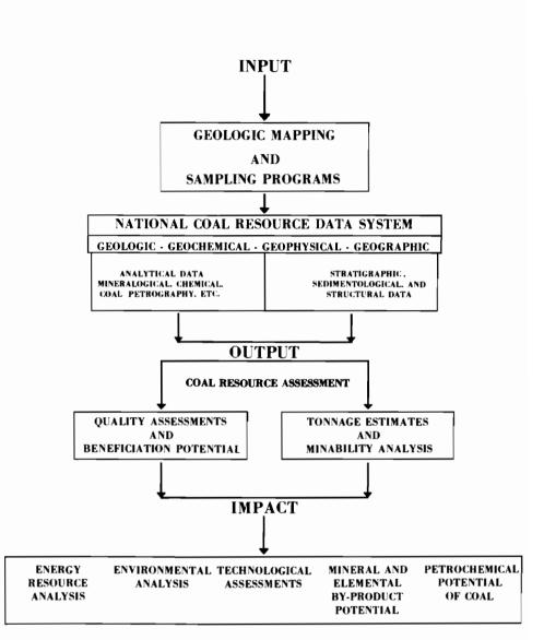
Figure 2. Flow diagram depicting the interrelationship of geological mapping, sampling, National Coal Resources Data System, and coal resource assessment and subsequent impacts on coal quality, quantity, and utilization.
