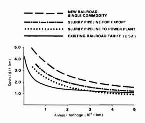
Figure 7. Cost comparison of slurry pipeline with railways.
