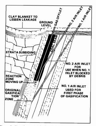
Figure 2. Use of two air inlet boreholes in a steeply sloping seam. Source: [5]
