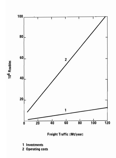
Figure 4. Dependence of investments and operating costs on freight traffic volume for a slurry preparation plant.
