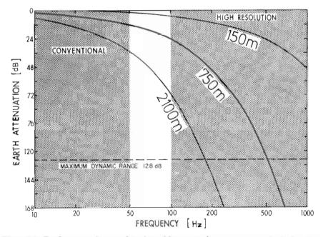
Figure 11. Earth attenuation as a function of frequency for an average geological section. It can be seen that as depth increases, attenuation reduces the signal levels to a point where dynamic range is exceeded, thereby eliminating higher frequency components in the reflection signals. V = 3050 m/s; a = 0.5 dB/ $\lambda$ .
