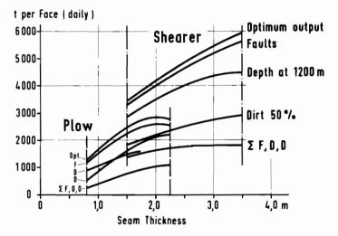
Figure 10. Output from shield faces under different geological conditions.
