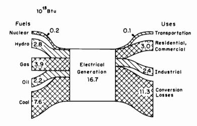
Figure 11. Balances in conversion to electrical energy.
