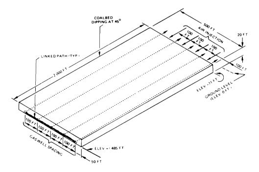
Figure 6. One SDB gasification module showing major dimensions (not to scale).
