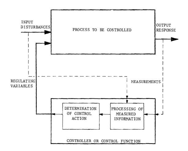
Figure 1. A framework for analysis: basic components of a process control system (dashed lines indicate measurements).
