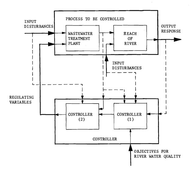
Figure 4. A hierarchical control scheme: controller (1) specifies the desired performance (objectives) for controller (2) (dashed lines indicate measurements).
