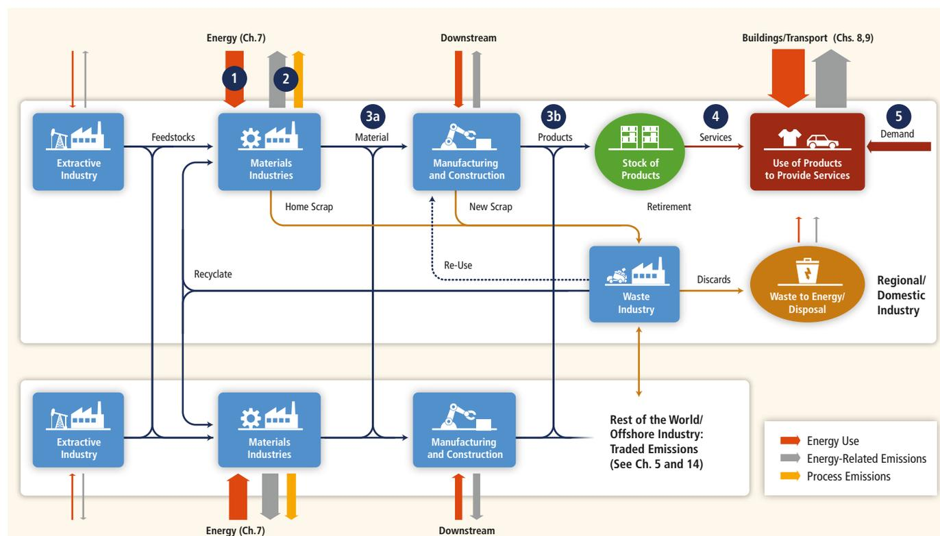
**Figure TS.25** | A schematic illustration of industrial activity over the supply chain. Options for mitigation in the industry sector are indicated by the circled numbers: (1) energy efficiency; (2) emissions efficiency; (3a) material efficiency in manufacturing; (3b) material efficiency in product design; (4) product-service efficiency; (5) service demand reduction. [Figure 10.2]
