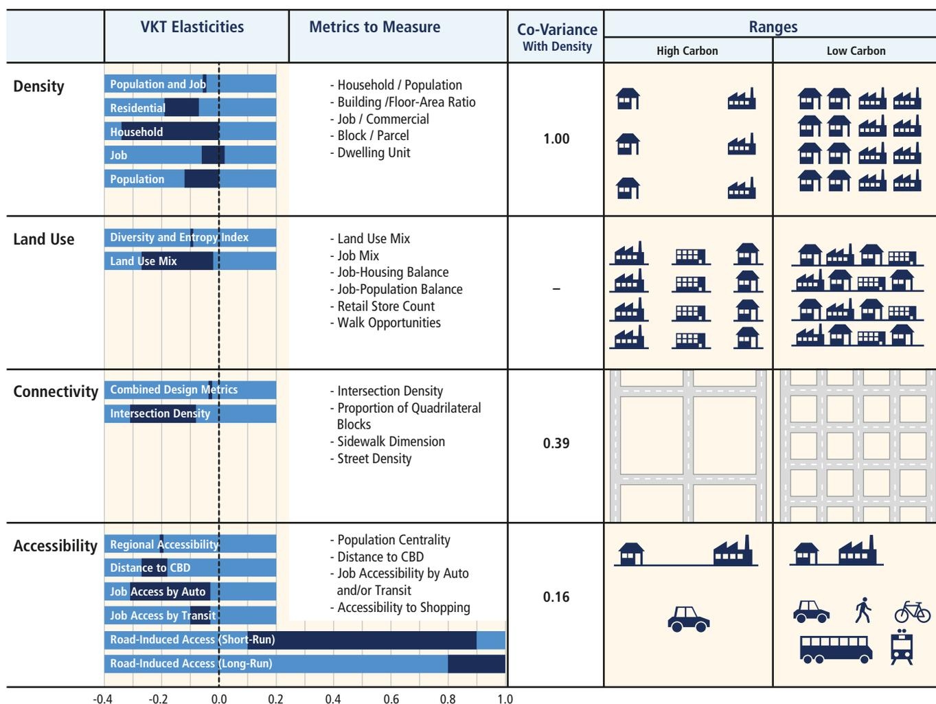
**Figure TS.33** | Four key aspects of urban form and structure (density, land-use mix, connectivity, and accessibility), their vehicle kilometers travelled (VKT) elasticities, commonly used metrics, and stylized graphics. The dark blue row segments under the VKT elasticities column provide the range of elasticities for the studies included. CBD: Central business district. [Figure 12.14]
