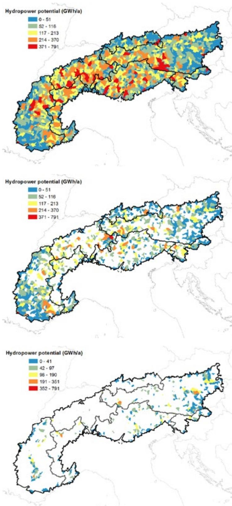
A DSS was applied to identify the economic potential of hydropower plants. A business-as-usual scenario would contribute to increasing the capacity of hydropower stations by 10% up from the actual capacity, with new power stations being set up across the Alps. With a view to cost minimisation
