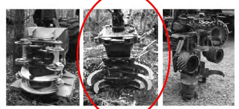
Figure 6. Felling and harvester heads used in the study. From the left the Bracke C16.a disc saw head, the Log Max 4000B harvester head and the Naarva-Grip 1500–40E guillotine head. Photo: Helmer Belbo
