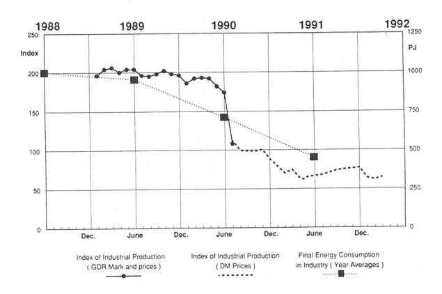
Figure 4. Evolution of industrial output (value index) and energy consumption (PJ) in the former GDR.
