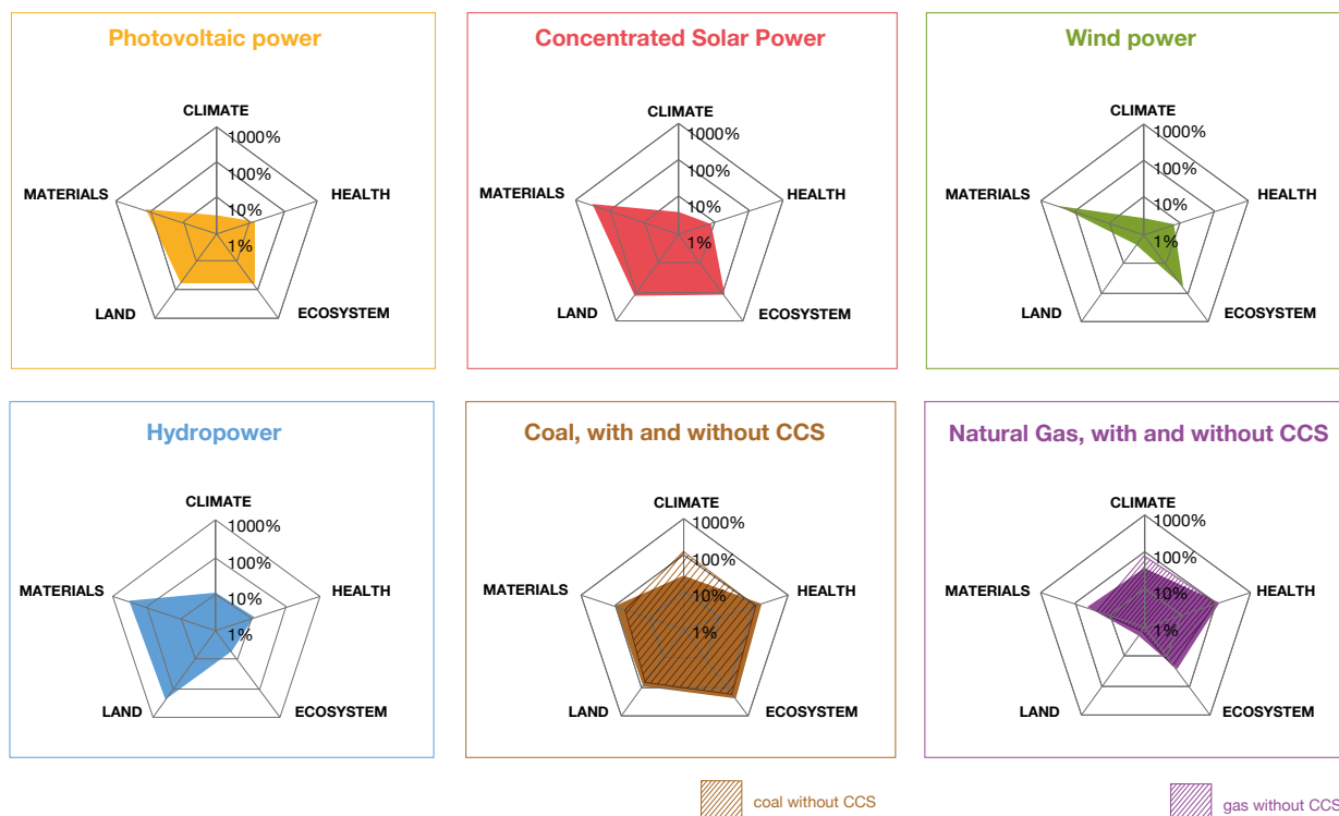
Figure 7: An overview over the life cycle results of different technology groups compared to the global average mix of electricity production technologies. The indicators are the use of the bulk materials (cement, iron and steel, copper, and aluminium), land occupation, greenhouse gas emissions, and the endpoint indicators for human health and ecosystems (excluding the contributions of climate change and land use, but including the production of materials.)
