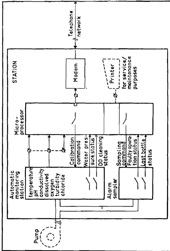
Figure 3. Principle of an automatic quality monitoring station (Philips)
