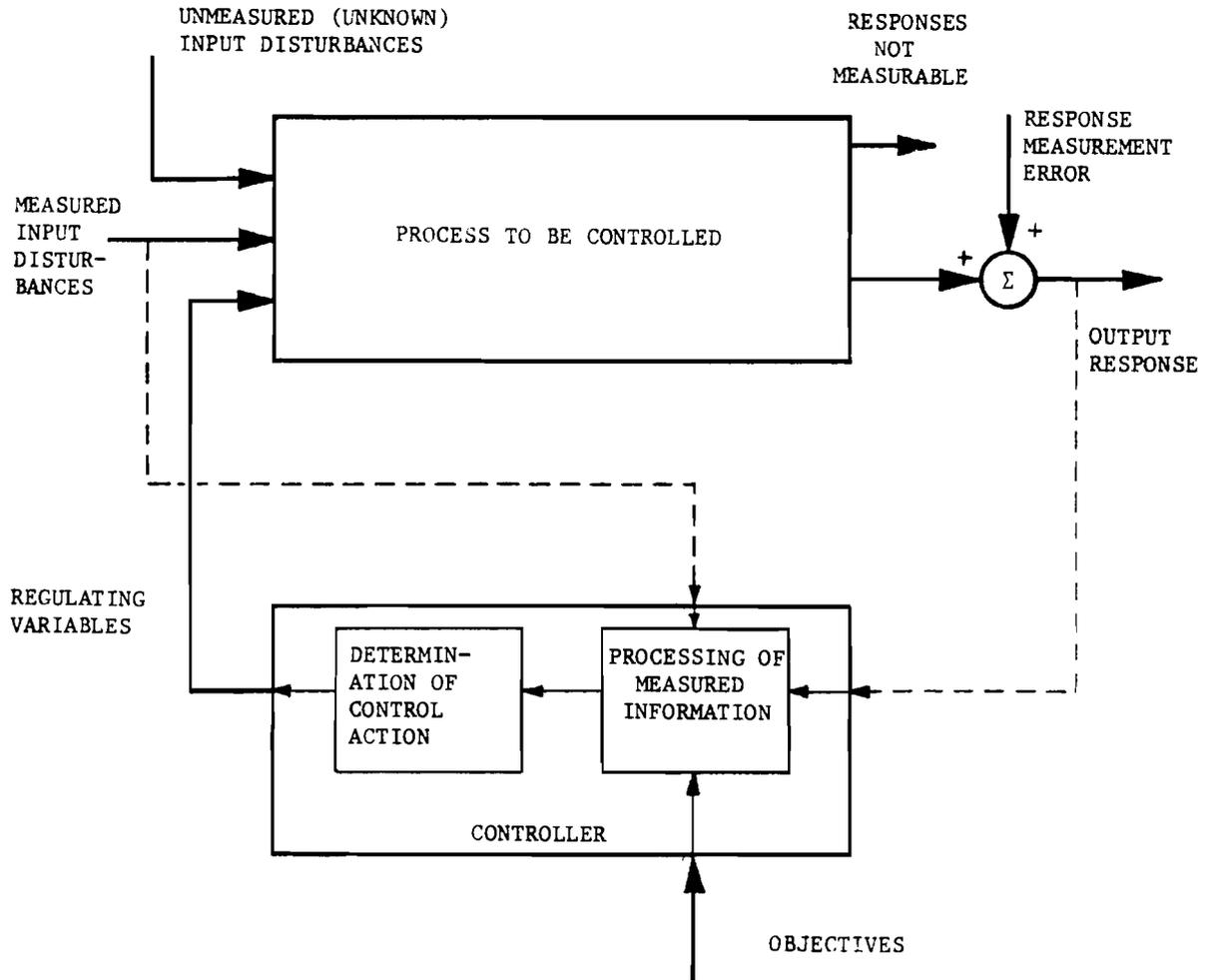
Figure 6. Management with feedback (dashed lines indicate measurements).
