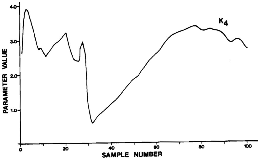
Figure 8. Recursive Estimate of Ammonia Decay Coefficient and Measured Flow at Tempsford
