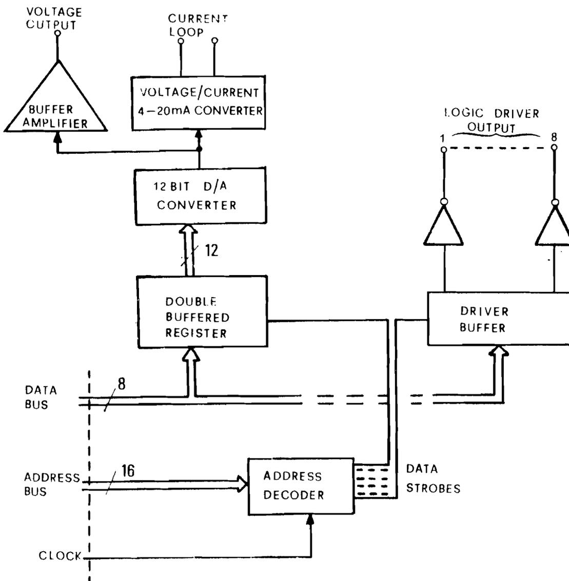
Figure 4. Schematic diagram of a Digital/Analog converter. The particular output port is selected via the address bus and a timed decoding circuit. Buffered registers are required to load 12-bit variables via an 8-bit data bus. Voltage and current outputs should be provided in case current-loop actuators have to be driven. Logic output is also useful in the case of stepping devices, for example, when stepping motors are provided as actuators.
