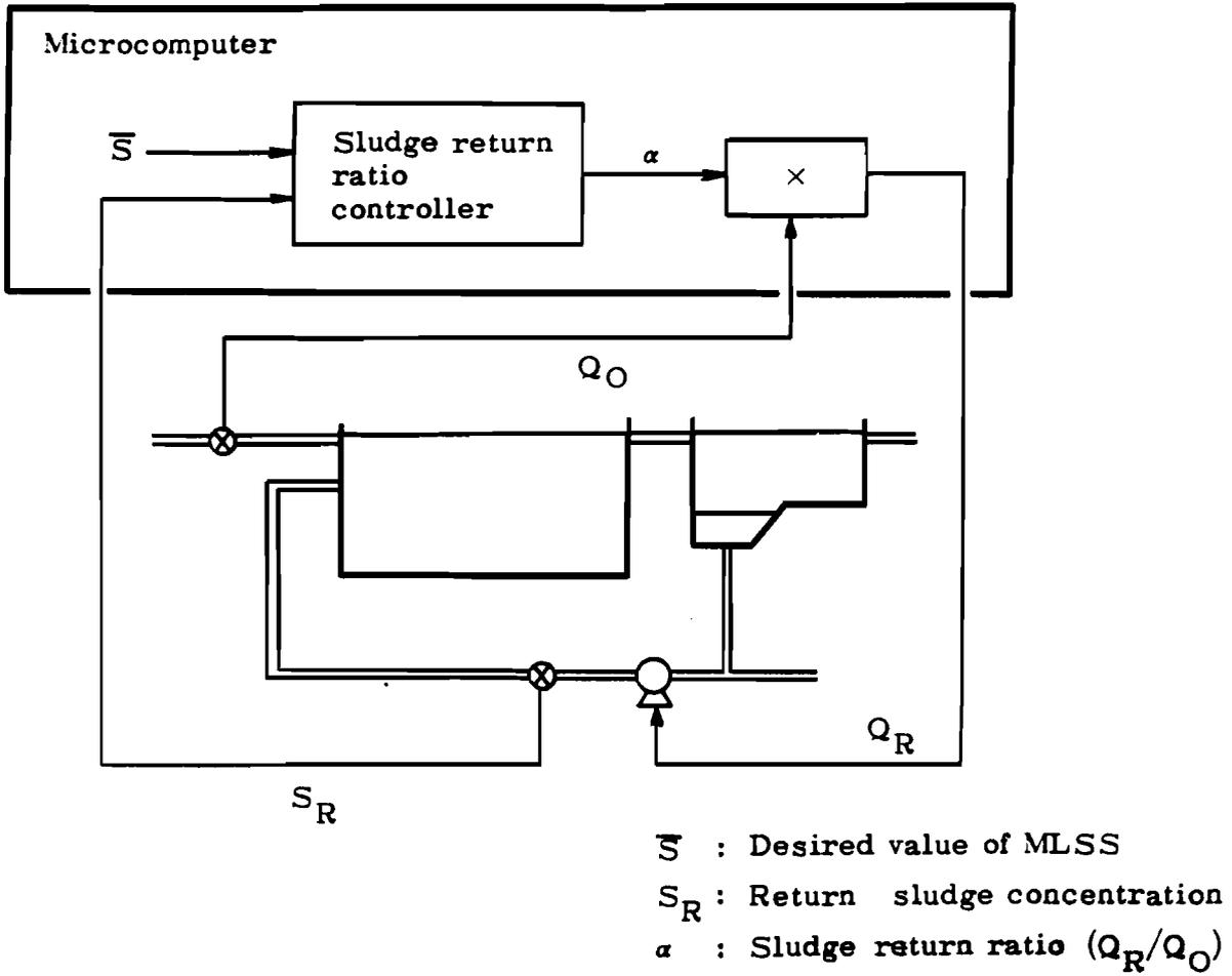
Figure 6. Block diagram for MLSS controller
