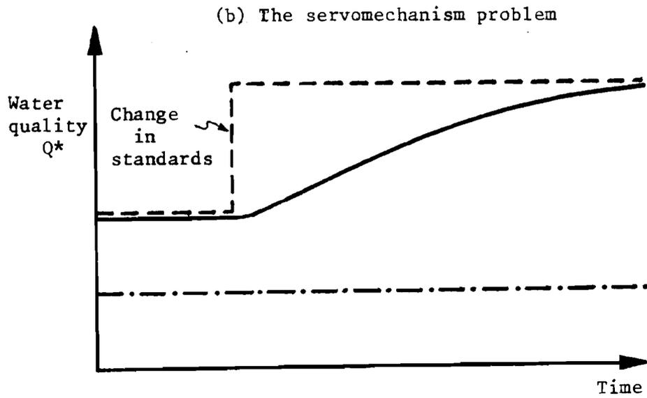
Figure 3. Two types of control problem: (a) the regulator problem; (b) the servomechanism problem.
