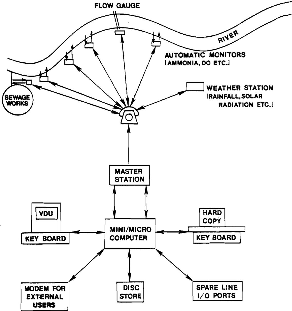
Figure 6. Monitoring, Telemetry and mini/micro Computing System Operational Management
