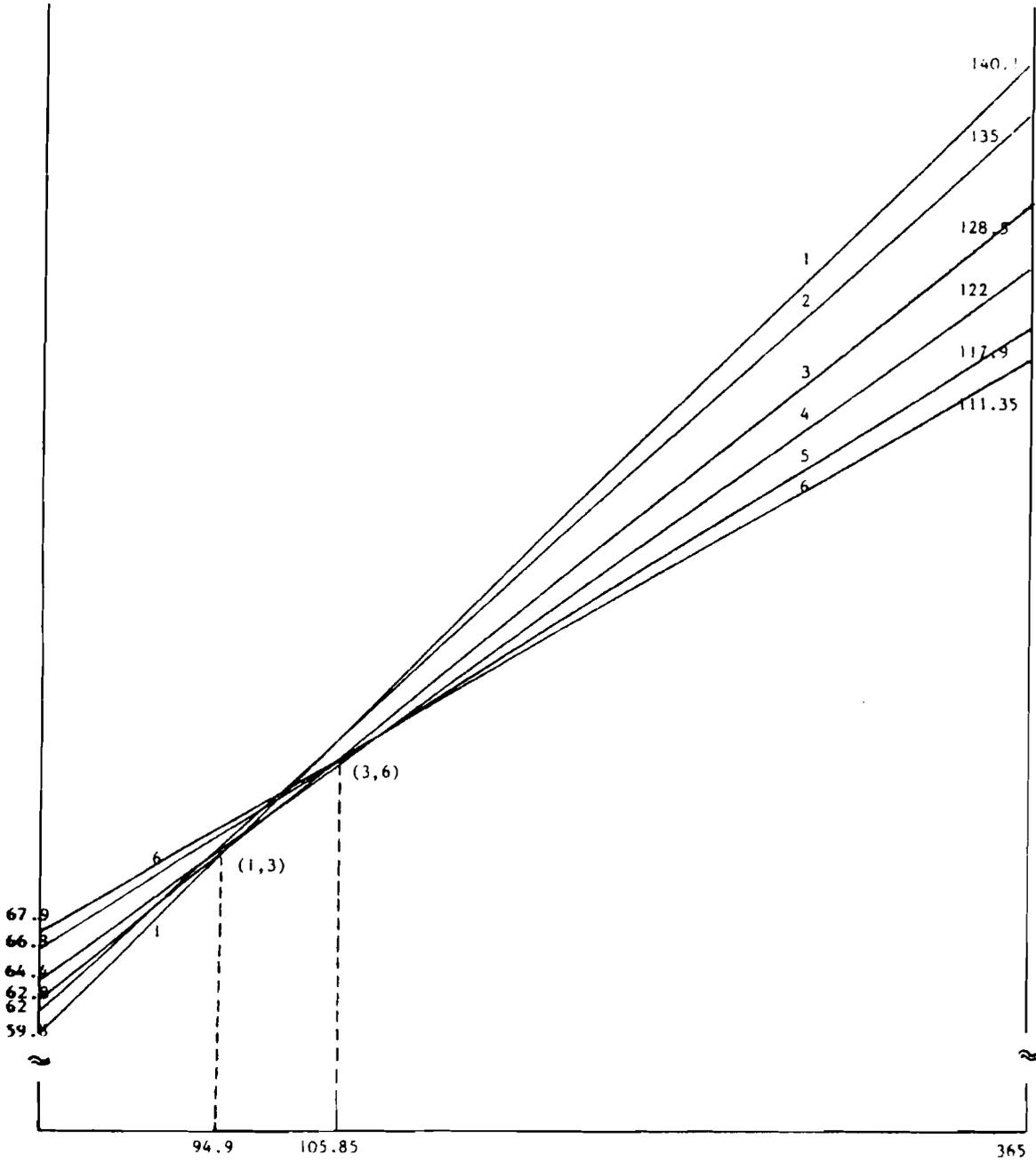
Figure 11. Annual cost as a function of the plant utilization.
