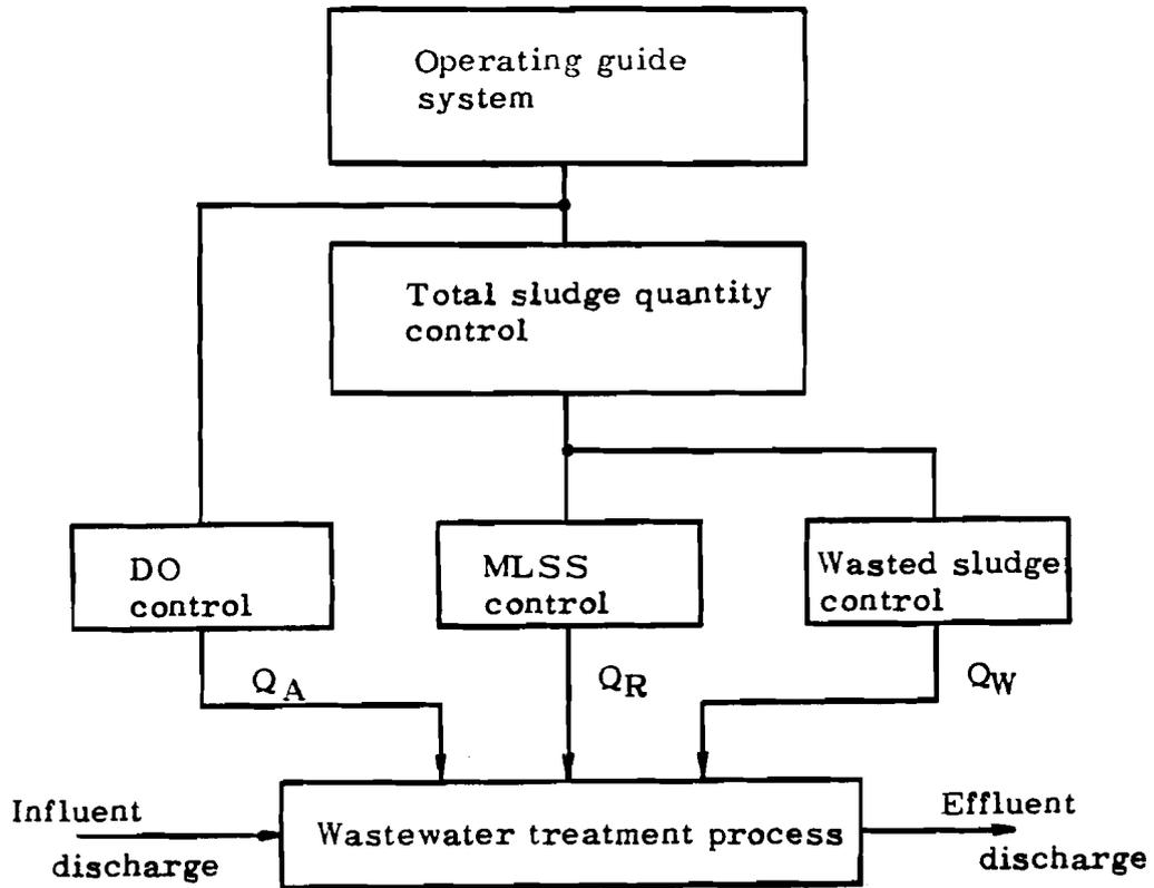
Figure 2. Organization of the wastewater treatment control system
