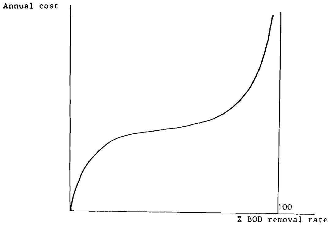
Figure 6. Annual cost as a function of the BOD removal rate.
