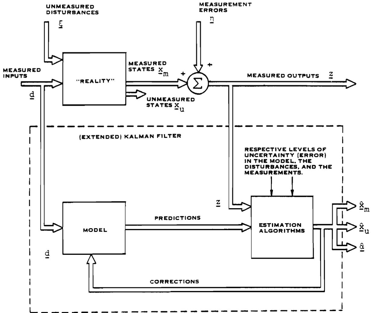
Figure 2. The (extended) Kalman Filter, an algorithm for estimation and forecasting;  $\hat{\underline{x}}_m$ ,  $\hat{\underline{x}}_u$ , and  $\hat{\underline{d}}$  are respectively estimates of the measured state variables, the unmeasured state variables and the model parameters.
