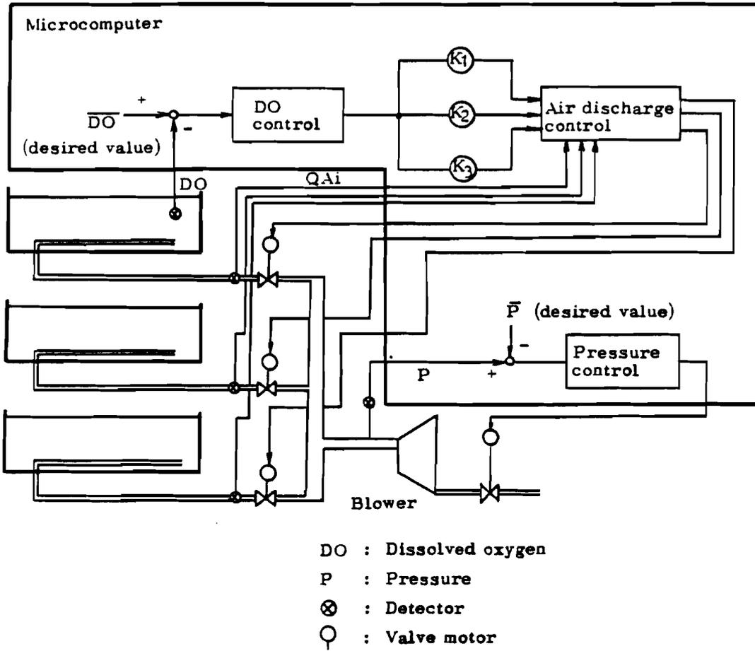
Figure 3. Block diagram of DO control
