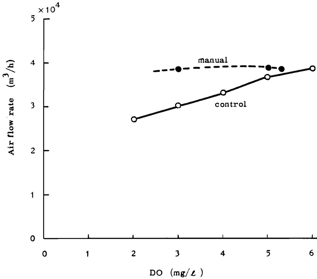
Figure 5. Effect of DO control on air flow rate reduction
