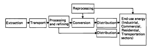
FIGURE 33 The general structure of the reference energy system used in the demand/supply balance approach.
