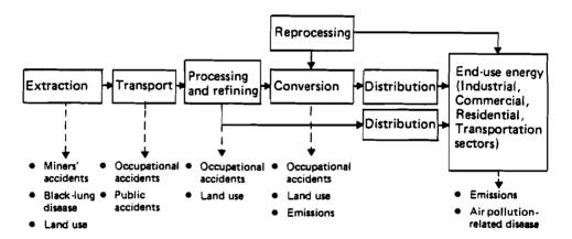
FIGURE 38 Typical environmental impacts associated with each point in the fuel chain.
