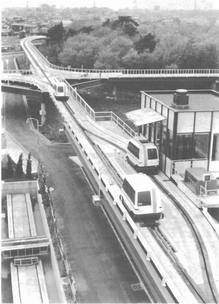
FIGURE 19.3 A CVS off-line station is called *stop* and is composed of a passenger berth and a container berth; a personal car has stopped at the passenger berth. The photograph also shows an automatic handling machine (far right-hand side) and an at-grade crossing (top).
