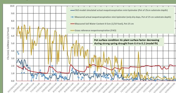
Figure 4: Greenroof (AKH, Vienna): daily minilysimeter based and simulated water balance parameters (June-December 2022, calibrated)
