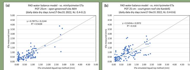
Figure 3a-b: Comparison of daily actual evapotranspiration measured by minilysimeter vs. simulated by the FAO method (calibrated)
