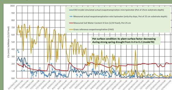
Figure 4: Greenroof (AKH, Vienna): daily minilyimeter based and simulated water balance parameters (June-December 2022, calibrated)
