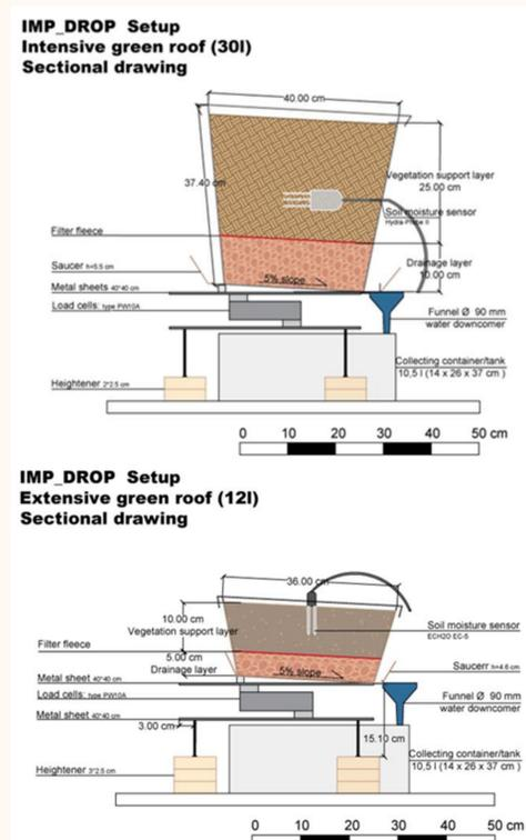
Figure 1: Sectional drawing of the experimental setup of the lysimeter for the investigation of an intensive (top) and extensive (below) green roof
