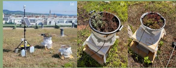
Figure 2a-c: Final setup of the experimental units covered up with white foil at the non-irrigated setups at the site (a) AKH Vienna and Kandlgasse with intensive (b) and extensive (c) green roofs
