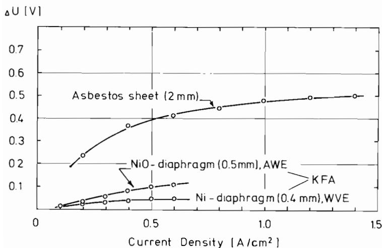
FIGURE 4 Ohmic voltage losses at diaphragms as a function of current density.
