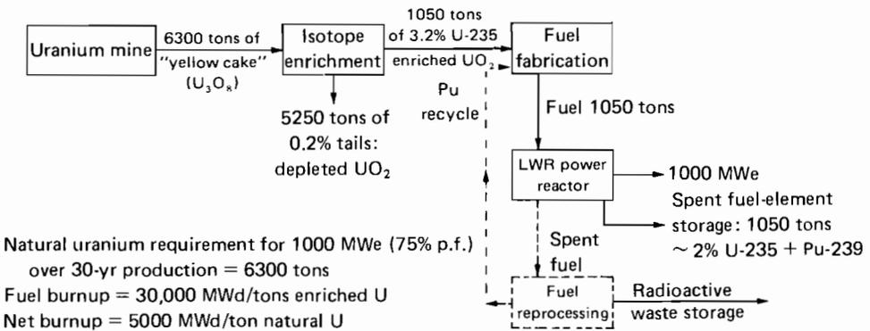
FIGURE 8 The conventional LWR nuclear fuel cycle.
