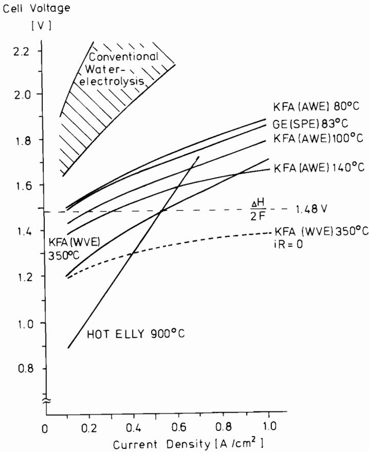
FIGURE 2 Current density versus cell voltage characteristics for various electrolytic procedures for water splitting.
