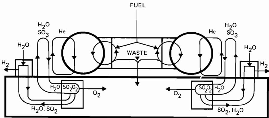
FIGURE 5 A cross section of a reactor+chemical-plant barge for the energy island. The thick circles refer to the toroidal reactor vessel and the chemical flows refer to the Westinghouse process (Farbman, 1976) for splitting water. Reprocessing and fuel refabrication in an on-board process are also indicated. The linear size of the barge is about 300 m.
