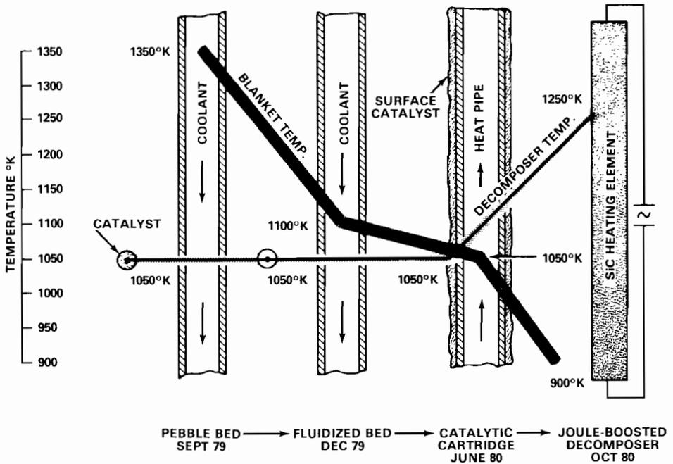
FIGURE 10 Progress in lowering the blanket temperature and raising the decomposer temperature for syngas applications.
