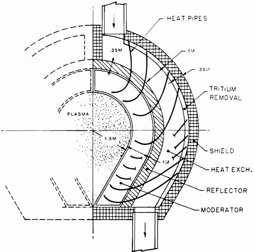
FIGURE 11 A heat-pipe blanket module.
