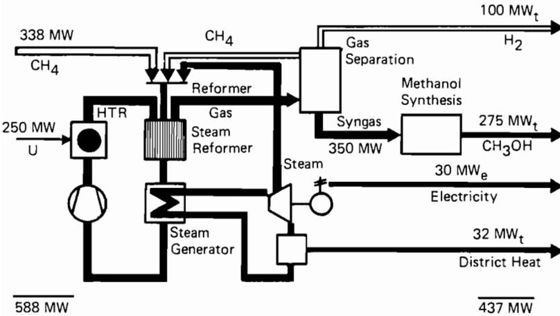
FIGURE 11 A schematic process for converting methane to methanol using an HTR.
