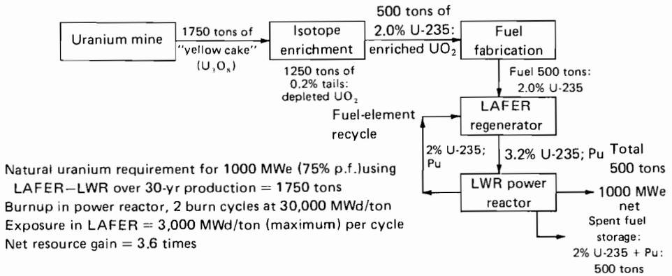
FIGURE 9 A LAFER fuel cycle with no reprocessing.
