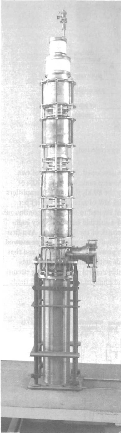
FIGURE 15 The test klystron VE07SK. With a power capability of 1.5 MW and an efficiency of 70% the klystron is a development step towards the SNQ series production klystron.
