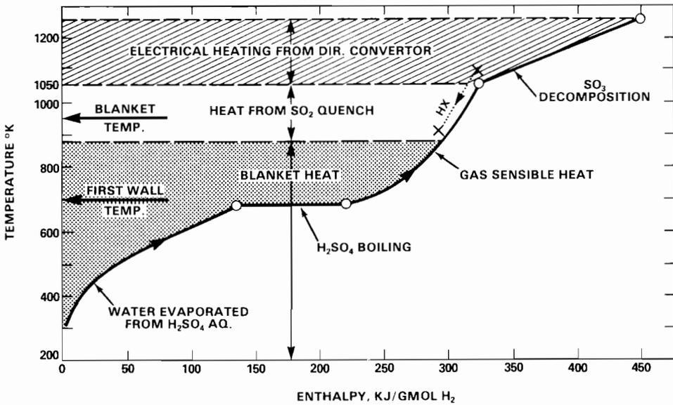
FIGURE 9 The heating curve for the  $\text{H}_2\text{SO}_4$  process step.
