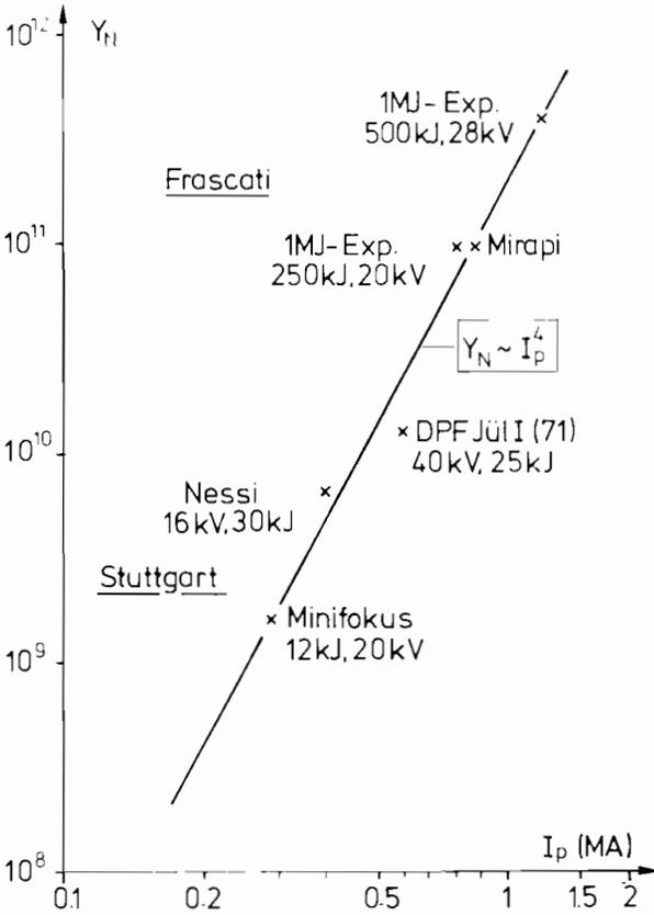
FIGURE 4  $^2\text{H}-^2\text{H}$  neutron yield as a function of plasma current.
