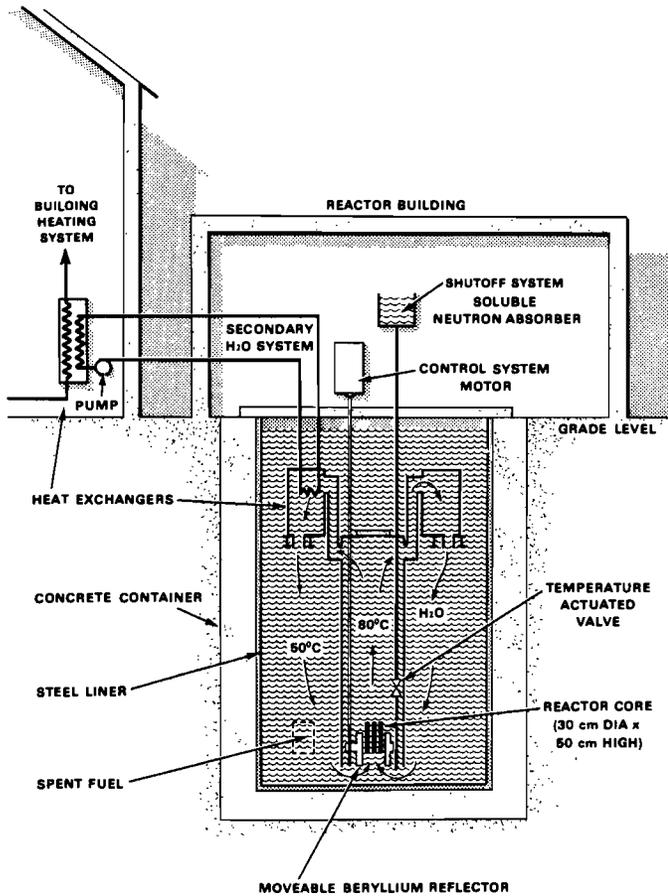
FIGURE 2 A 2-MW SLOWPOKE heating reactor.
