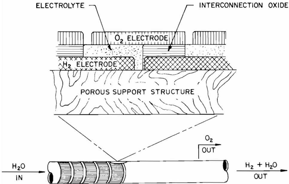
FIGURE 6 HTE cell design (the Westinghouse fuel cell).
