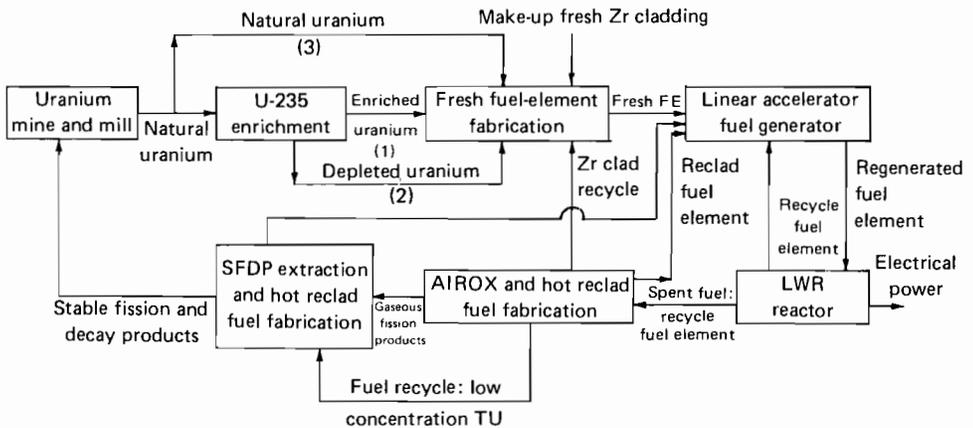
FIGURE 14 The APEX LAFER-LWR fuel cycle and waste management (spent-fuel storage): FE, fuel elements; SFDP, stable fission and decay products; TU, transuranics. Note that fuel elements can be fabricated with enriched uranium, depleted uranium, or natural uranium.
