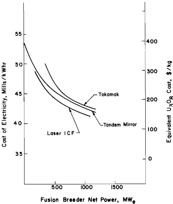
FIGURE 5 Estimated economics of various types of fusion driver (with thorium fission-suppressed blanket).
