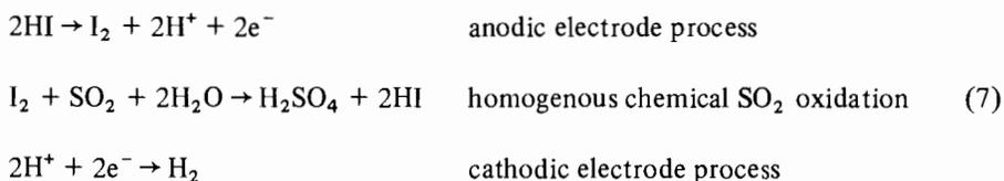
The sulfuric acid is then concentrated from 58 to 70 wt.%, separated from very small residual amounts of HI by distillation, and subsequently decomposed as in the first
