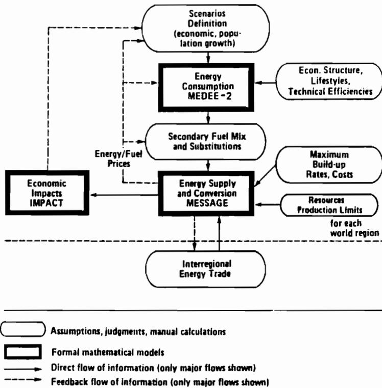
FIGURE 4 IIASA's set of energy models: a simplified representation.
