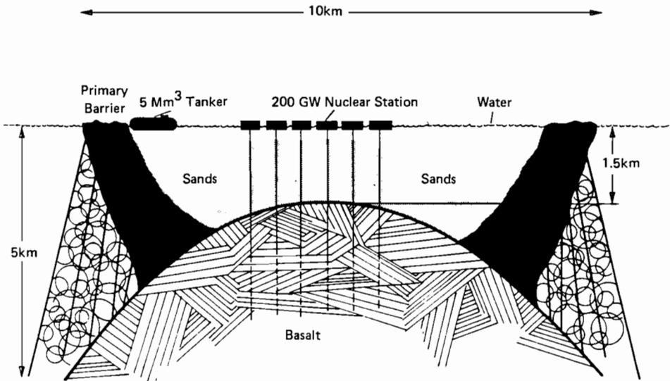
FIGURE 7 A scale cross section of Canton "Energy Island" with its presumed geological structure. The full lines under the power station barges represent permanent radioactive-waste sink holes and the broken extensions represent the free trajectories of the sinking capsules.
