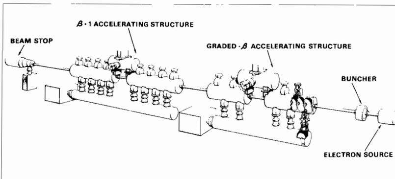
FIGURE 5 The Chalk River Nuclear Laboratories electron test accelerator for experiments on the acceleration of intense beams with a large accelerating gradient at 100% duty factor in a coupled-cavity linac typical of the high-energy section of an accelerator breeder.
