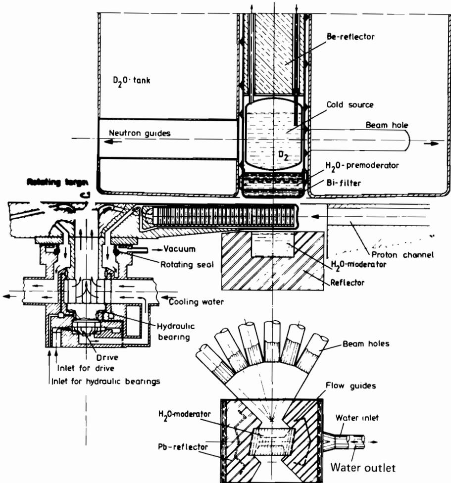
FIGURE 17 The hybrid moderator concept proposed for the target station DIANE. A large volume of high neutron flux, housing the cold neutron source and irradiation facilities (not shown), is arranged above the target to facilitate access from above. The  $H_2O$  moderator below the target is surrounded by a lead reflector on three sides and is viewed by 12 beam tubes.
