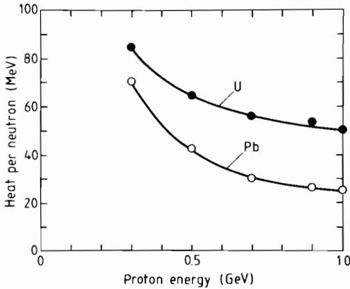
FIGURE 7 Heat release per neutron for lead and uranium as a function of proton energy (from Bartholomew and Tunnicliffe, 1966).
