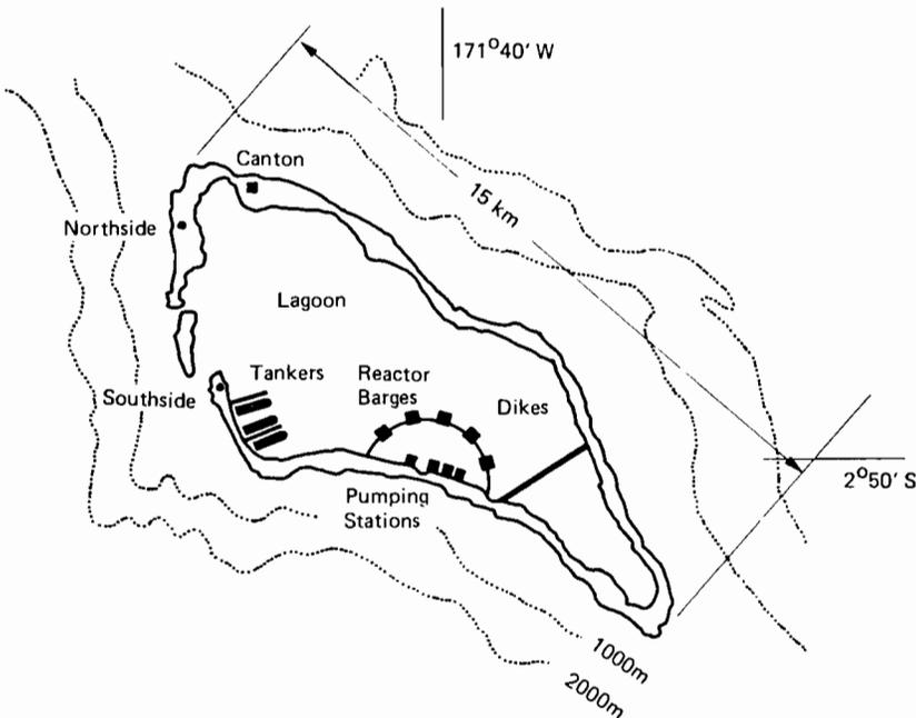
FIGURE 6 A plan view of Canton Island, with the installation drawn to scale. Each barge represents 200 GWth of primary energy. The island is located in the central equatorial Pacific ( $171^{\circ} 40' \text{ W}$ ,  $2^{\circ} 50' \text{ S}$ ).
