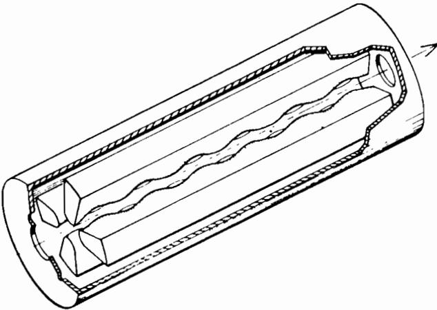
FIGURE 3 A cutaway view of an RFQ accelerating structure (reprinted with permission from Crandall et al., 1979). The RFQ would be the low-energy accelerating structure in an accelerator breeder.
