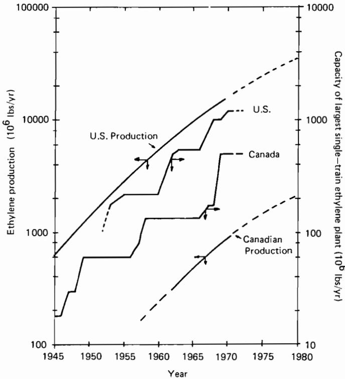
FIGURE 1 The size of the largest production units (stepped curves) and the size of the market (smoothed curves) for ethylene in the United States and in Canada. Technology is obviously "hunting" the market.
