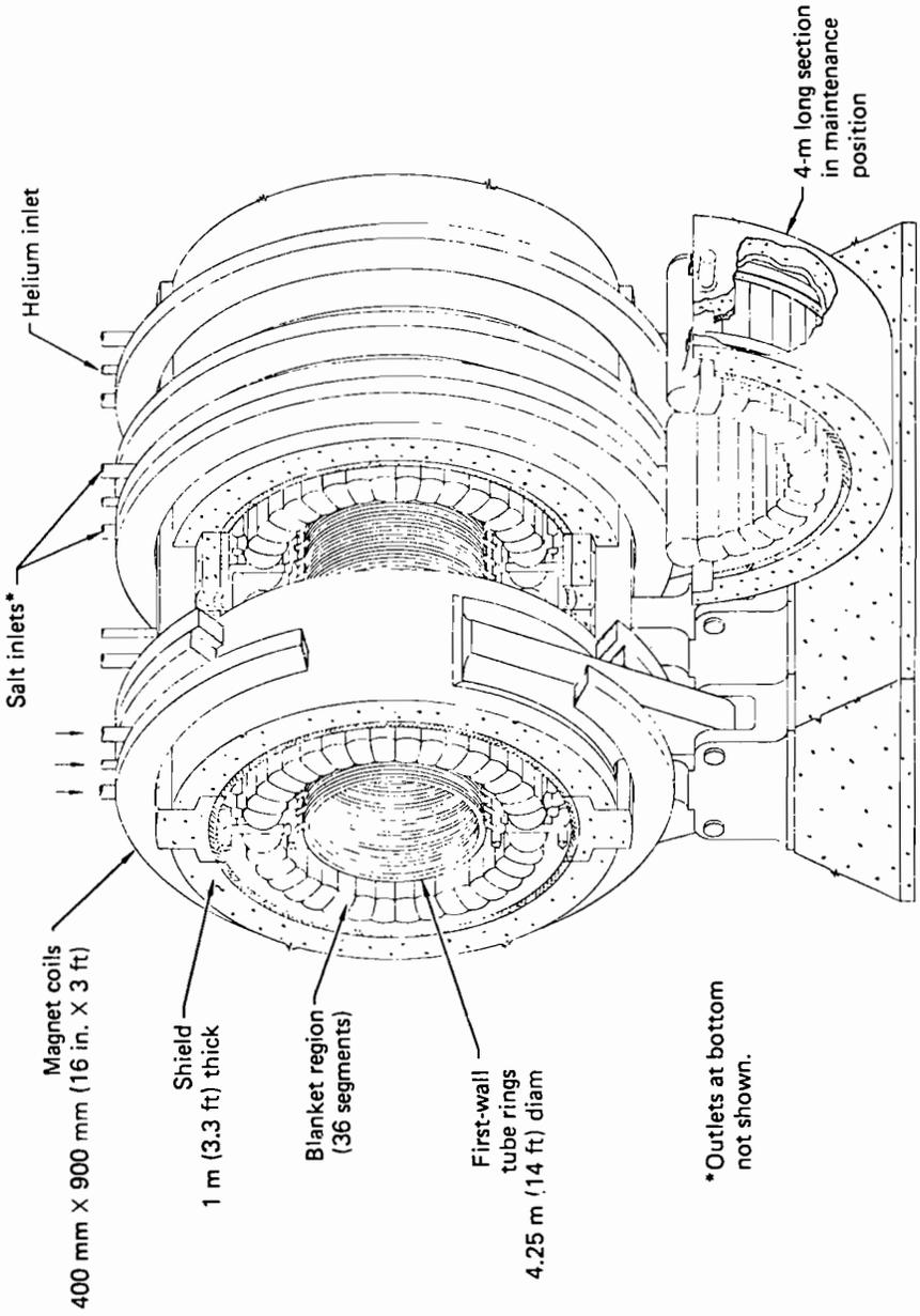
FIGURE 3 Mechanical layout of a central cell module for a tandem-mirror device with a beryllium/molten salt blanket.
