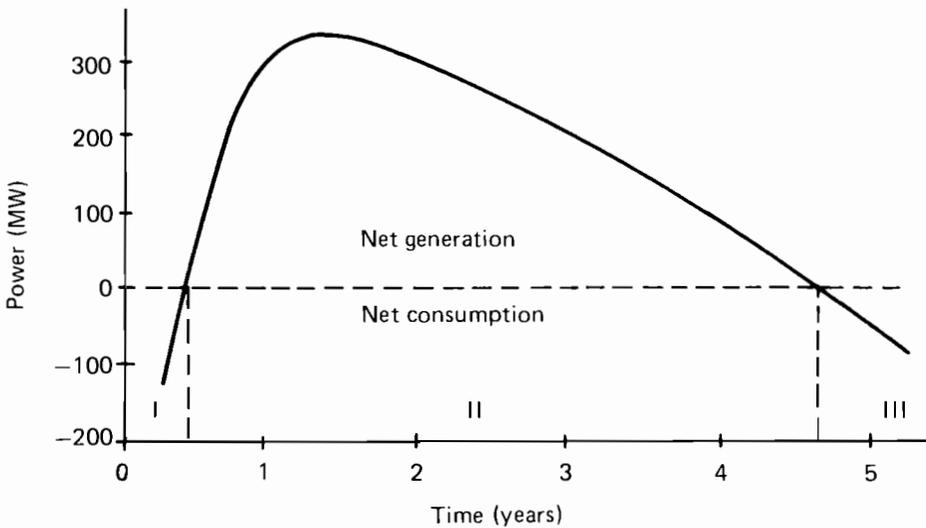
FIGURE 1 The temporal cycle of system operation for the proposed hybrid: I, initial stage; II, working stage; III, final stage.
