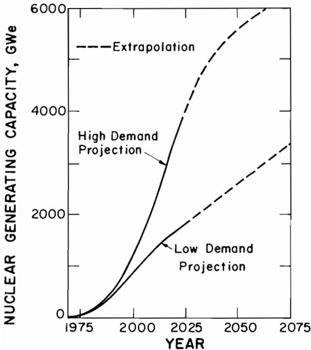
FIGURE 1 Projected world nuclear capacity (excluding areas with centrally planned economies) (INFCE, 1979); the low demand projection was used in this study.
