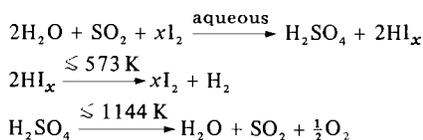
*Sulfur cycle (part electrochemical) (Westinghouse Electric Corporation)*
