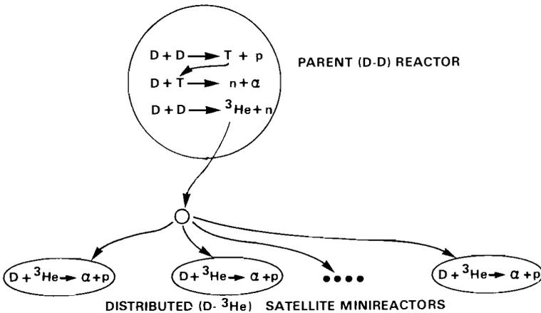
FIGURE 2 A depiction of a set of D- ${}^3\text{He}$  fusion minireactors supported by a  ${}^3\text{He}$ -breeding fusion reactor.
