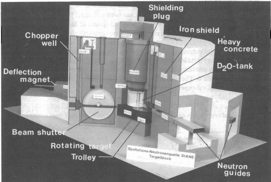
FIGURE 18 A cutaway model view of the target block of the target station DIANE.
