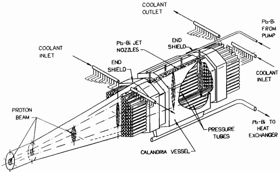
FIGURE 4 An HWR-type target assembly.
