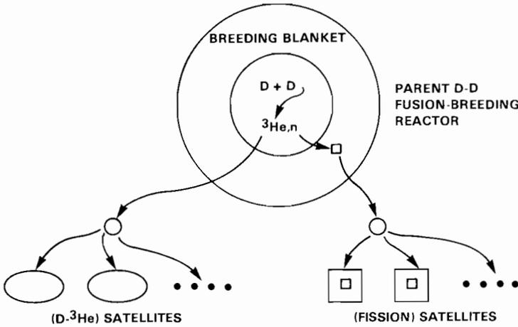
FIGURE 3 An illustration of a D-D-fueled hybrid reactor supporting both fusion and fission mini-reactors.
