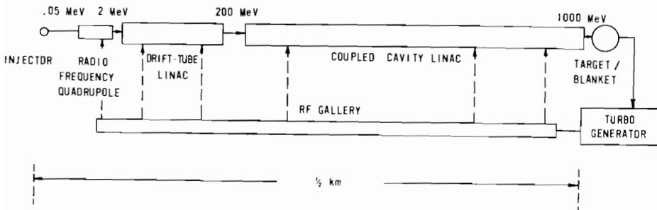
FIGURE 1 A schematic diagram of the main components of an accelerator breeder.
