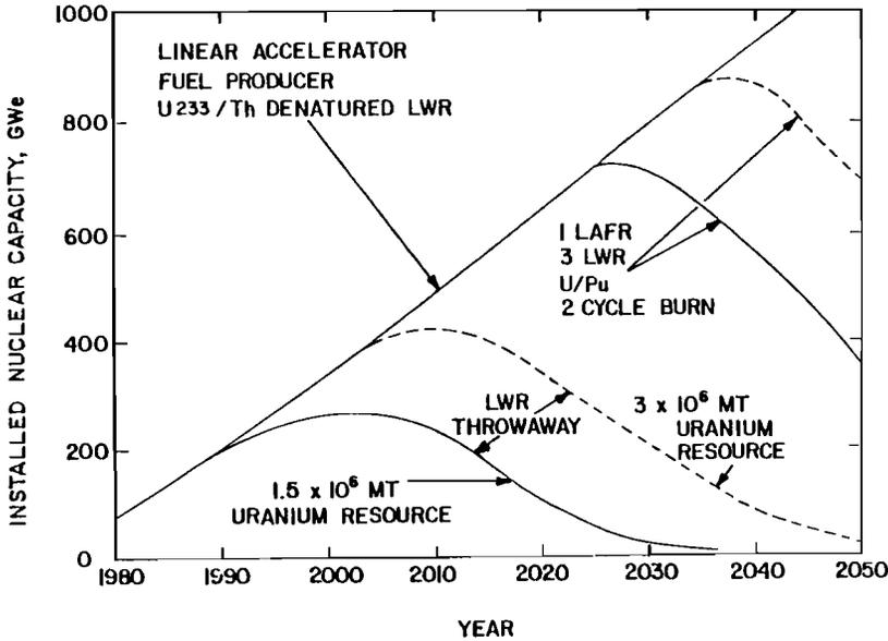
FIGURE 13 Nuclear power growth patterns: the effect of LAFER systems (small  $U_3O_8$  supply) for a capacity growth rate of  $15 \text{ GWe year}^{-1}$ .
