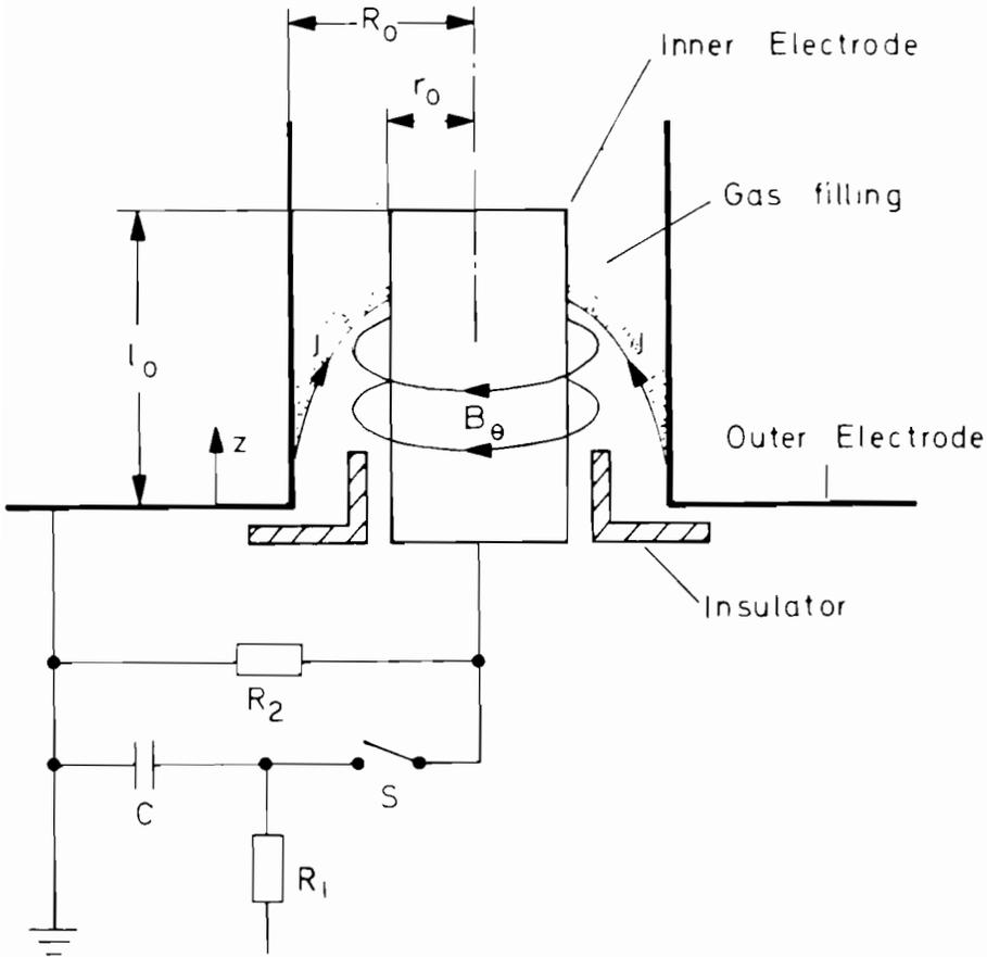
FIGURE 1 The start-up of a plasma focus discharge (schematic).
