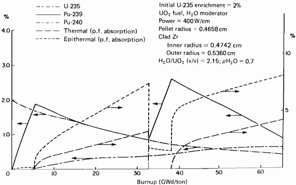
FIGURE 10 The concentration of U-235, Pu-239, and Pu-240 neutron absorption due to fission products in a LAFER.
