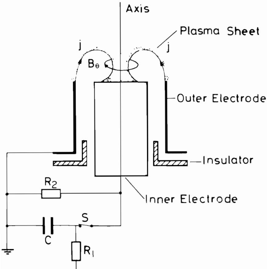
FIGURE 2 The final phase of a plasma focus discharge (schematic).
