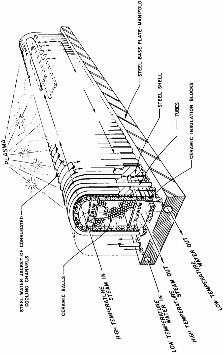
FIGURE 5 A representative HTE process module for a 5000-MW reactor.
