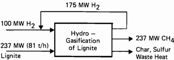
FIGURE 12 A schematic process for converting lignite to methane.
