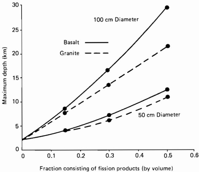
FIGURE 11 Capsules of various diameters, containing fission products of initial age six months, melt the surrounding rock by nuclear decay heat and thus sink. The final depth of penetration is shown as a function of the fraction by volume of fission products, for each combination of capsule diameter and surrounding rock.
