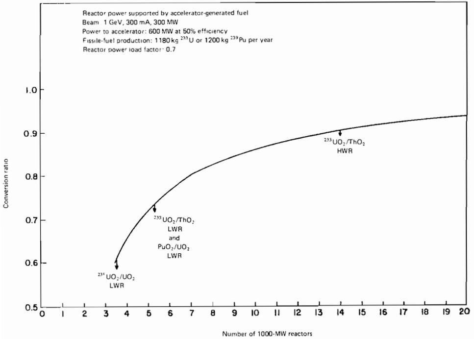
FIGURE 12 The reactor power supported by accelerator-generated fuel.
