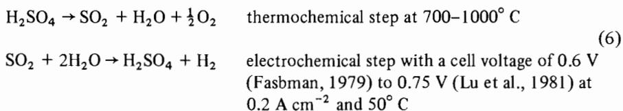
As can be seen, one complete cycle involves two molecules of water, of which one is split. The components of the  $SO_2/H_2SO_4$  system are not consumed but only cycled.
