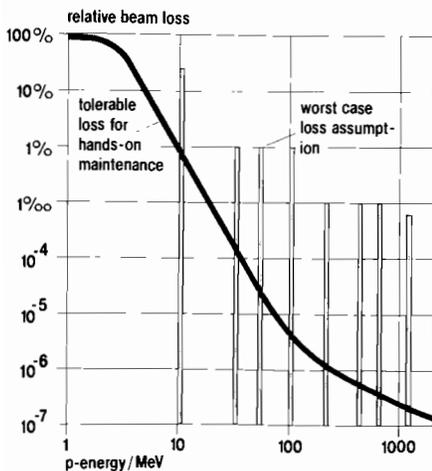
FIGURE 10 Beam loss versus proton energy. The upper limit of beam loss (fractions of total beam per meter of length) permissible for hands-on maintenance of the accelerator decreases steeply with proton energy (curve). The shaded bars show sources of point losses assumed as worst cases for the design of buildings, accelerator components, and handling systems.
