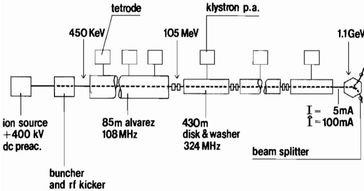
FIGURE 9 The schematic arrangement of the SNQ linac.
