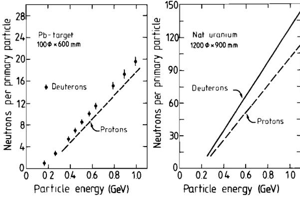
FIGURE 5 Neutron yield per primary particle for protons and deuterons on lead (100φ × 600 mm) and natural uranium (1200φ × 900 mm) targets (after Barashenkow et al., 1974); φ denotes diameter (mm).
