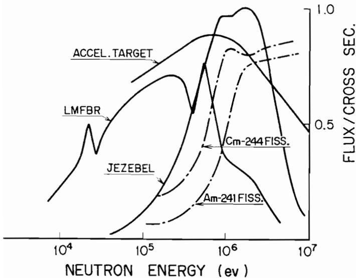
FIGURE 2 Neutron spectra and fission cross-sections.
