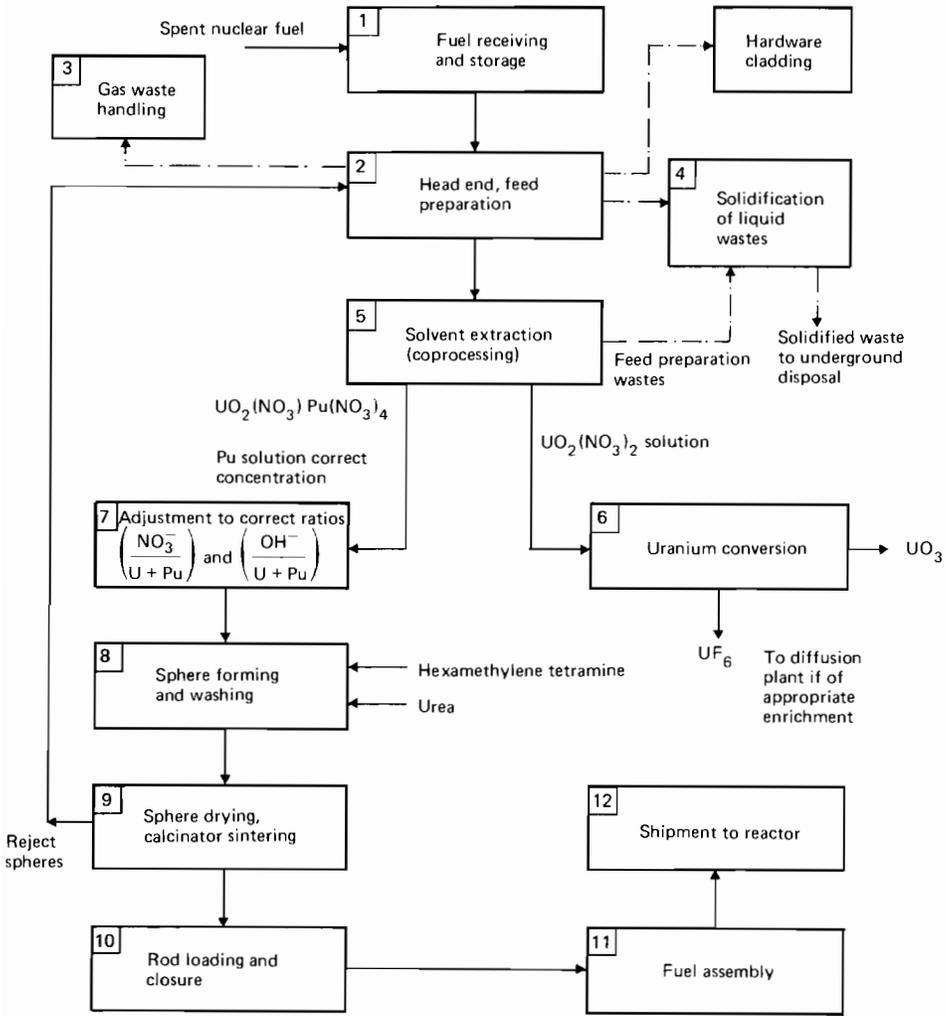
FIGURE 1 Generalized fuel-cycle flow sheet.
