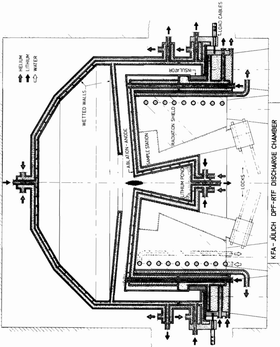
FIGURE 6 Conceptual design of a plasma focus as a neutron source.
