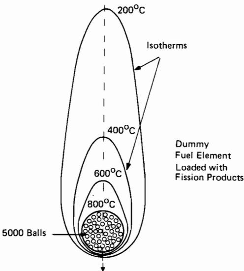
FIGURE 10 A “cooperative” sinking capsule, proposed because of the difficulty of building a large sphere capable of mechanically and chemically resisting the hard environment of molten rock under pressure: a large sphere is replaced by a large bunch of small spheres made, with the same technology, of the fuel elements of a pebble-bed nuclear reactor.
