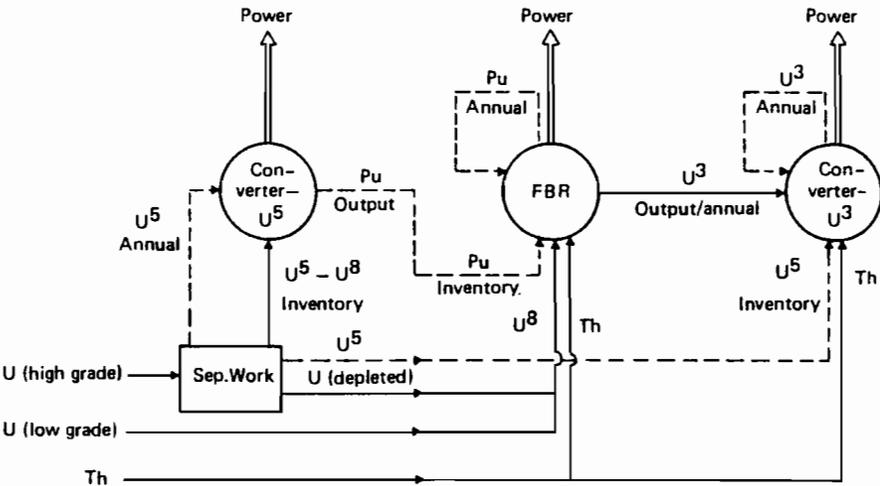
FIGURE 9 A converter-breeder system.
