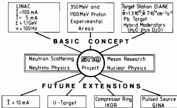
FIGURE 3 The basic concept, fields of research, and optional future extensions of the SNQ project.
