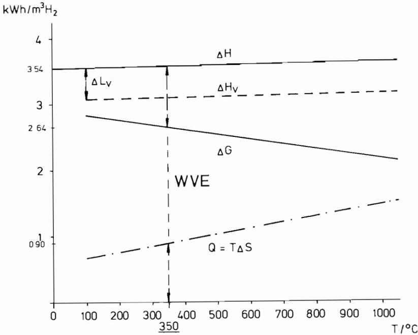
FIGURE 3 Thermodynamic functions of water electrolysis.  $\Delta H = \Delta G + T\Delta S$ , where  $\Delta H$  is the thermoneutral enthalpy,  $\Delta G$  is the free enthalpy supplied as electricity (in the absence of overvoltages and ohmic losses), and  $Q = T\Delta S$  is the enthalpy increment contributed as heat. The position (corresponding to case III in Table 2) for the WVE operated at 350° C is indicated.
