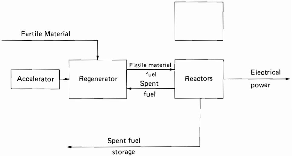
FIGURE 6 The scheme of the LAFER.
