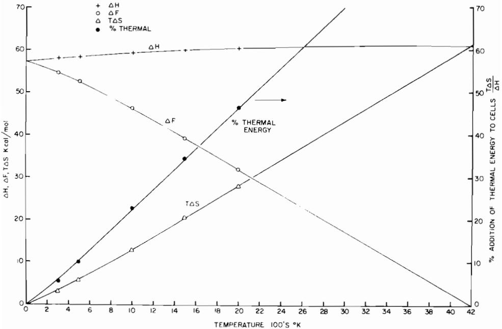
FIGURE 2 Fusion–HTE–synthetic-fuels thermodynamics of water decomposition (steam)  $H_2O(g) = H_2(g) + \frac{1}{2}O_2(g)$ .
