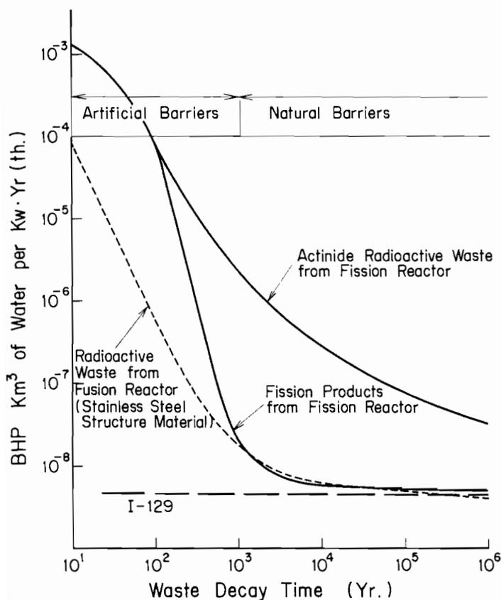
FIGURE 1 Decay and hazard characteristics of radioactive waste from fusion and fission reactors.
