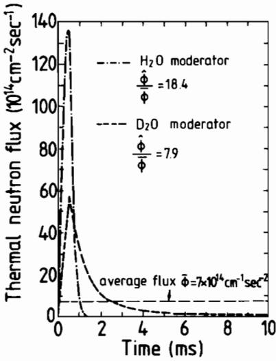
FIGURE 19 The time structure of the thermal neutron flux in the moderators of DIANE as derived from measured data.
