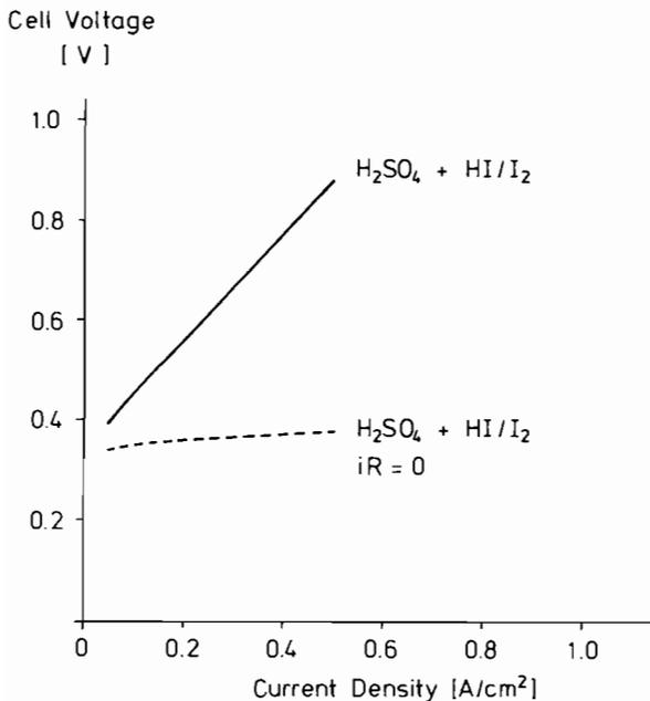
FIGURE 5 The current density versus cell voltage characteristics of the electrolytic step of the advanced sulfuric acid hybrid cycle. The broken curve corresponds to the measured performance without diaphragm ( $iR = 0$ ).
