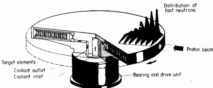
FIGURE 16 A schematic representation of the rotating target arrangement with individually canned target pins cooled by water which flows in and out through the hub of the wheel. The diameter of the wheel is 2.5 m and the height of the target material is 10 cm. The distribution of fast neutron leakage as calculated with the HFT code is indicated for the upper surface.
