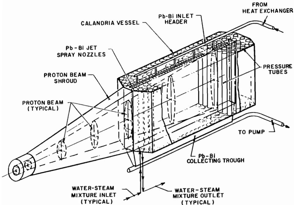
FIGURE 3 A PWR target assembly.
