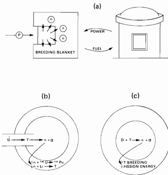
FIGURE 3 A schematic depiction of nuclear energy systems concepts combining (a) accelerators and fission processes, (b) accelerators and fusion processes, and (c) fusion and fission processes.
