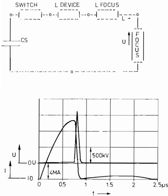
FIGURE 5 (Top) Auxiliary circuit of a plasma focus device. (Bottom) Voltage across and corresponding current in the power-amplifier compressor:  $W = 1 \text{ MJ}$ ;  $C = 32 \text{ } \mu\text{F}$ ;  $L_{\text{tot}} = 7 \text{ nH}$ ;  $U = 250 \text{ kV}$ .
