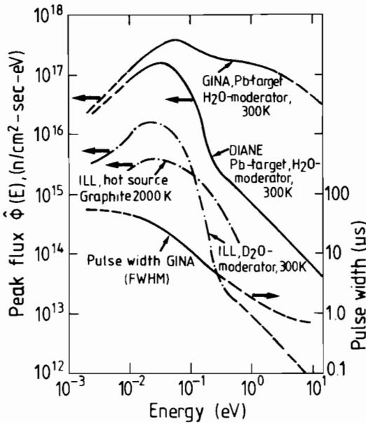
FIGURE 20 Peak neutron flux at DIANE as a function of energy in comparison to the steady-state flux at the HFR, Grenoble. The pulse width at DIANE is about 500  $\mu$ s for all energies and the time-average flux is a factor of 18–20 below the peak flux. The curve labeled GINA is for the option of a pulsed source as outlined in the text.
