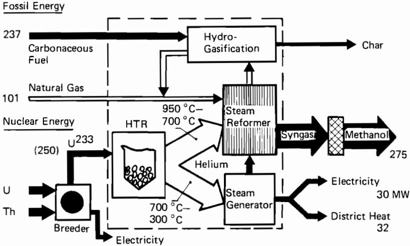
FIGURE 13 A zero-emission energy system for the conversion of dirt into secondary energy.
