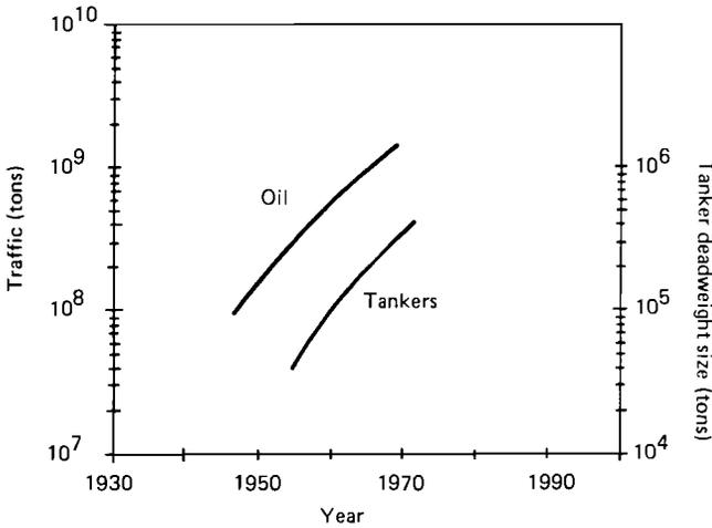
FIGURE 4 The evolutions of “largest-size” tankers and of the overseas oil market, showing a remarkable tuning. The number of tankers is actually to a large degree independent of the level of traffic.
