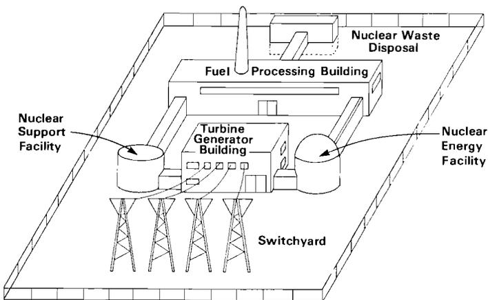
FIGURE 7 A schematic representation of a synergetic nuclear energy system. As indicated, one facility is optimized for energy production while another provides a support capacity. As suggested here, intrinsically safe fertile materials only would be transported into this energy park and energy is supplied to a power grid.
