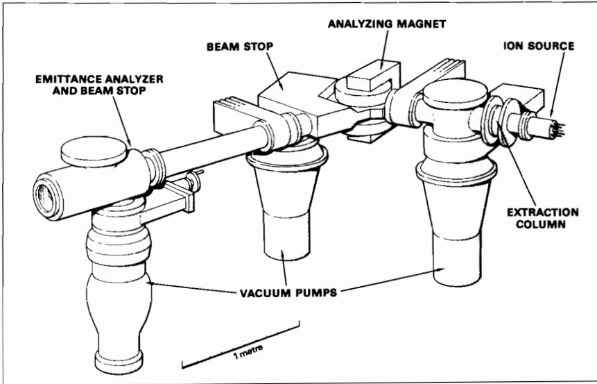
FIGURE 2 The Chalk River Nuclear Laboratories injector test experiment for experiments on ion sources and beam-formation columns for the accelerator breeder.
