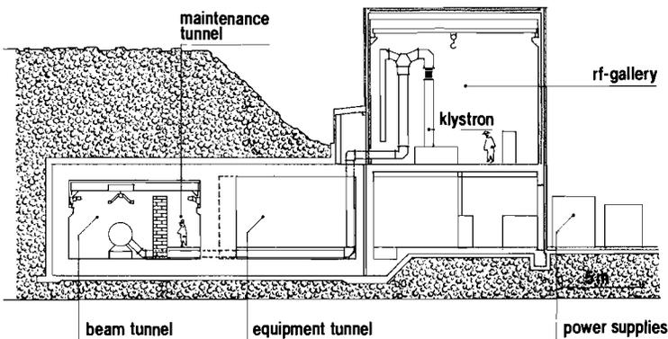
FIGURE 11 A cross section of the DAW accelerator. Zones of different accessibility are delimited from each other; the building of the RF gallery is freely accessible during machine operation.
