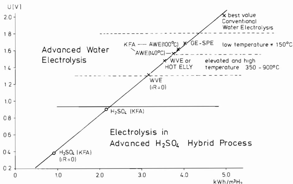
FIGURE 6 Relationship between required electricity in kilowatt-hours per cubic meter of  $H_2$  and cell voltage  $U$ . The points inserted for various electrolytic procedures refer to a current density of  $0.53 \text{ A cm}^{-2}$ .
