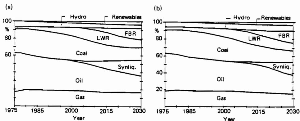
FIGURE 6 Global primary energy: shares by source for two supply scenarios, 1975–2030. (a) High scenario; (b) low scenario.
