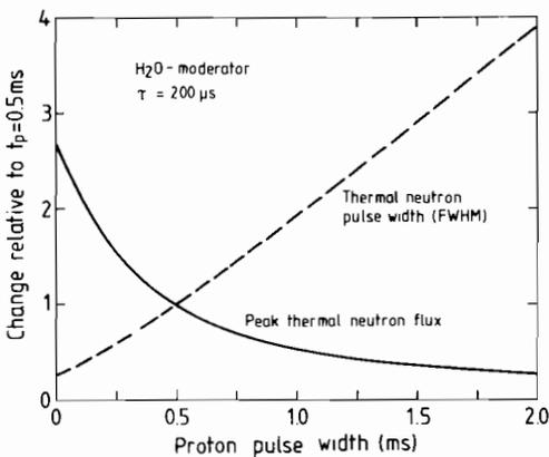
FIGURE 8 The change in peak thermal neutron flux and thermal neutron pulse width with proton pulse duration at constant source strength and repetition rate ( $H_2O$  moderator, with a decay time  $\tau$  of the thermal neutron field of  $200\mu s$ ). The FWHM at  $t_p = 0.5\text{ ms}$  is  $0.516\text{ ms}$ .
