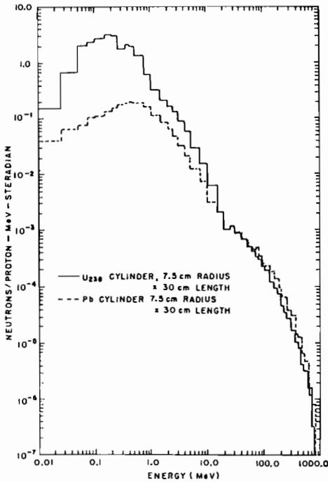
FIGURE 2 Neutron energy spectra produced by 800-MeV protons incident on lead and U-238 targets.
