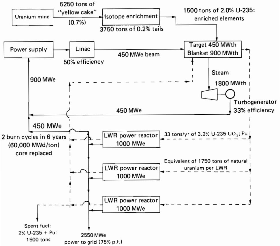
FIGURE 11 A system of three LWRs supplied by one LAFER.
