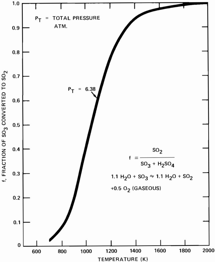
FIGURE 3 The  $\text{SO}_3$ - $\text{SO}_2$  equilibrium curve.
