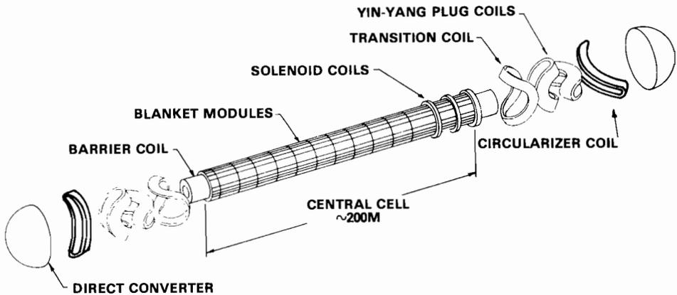
FIGURE 8 The tandem-mirror reactor.
