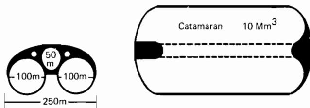
FIGURE 9 Vertical and horizontal cross sections of a possible  $\text{LH}_2$  tanker.
