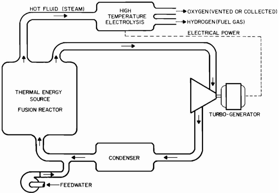
FIGURE 4 The general HTE process with a conventional power cycle.
