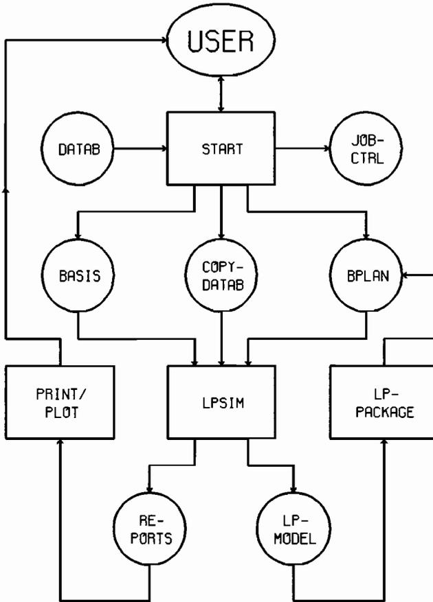
Figure 2 Interconnection of programs and files of CAP
