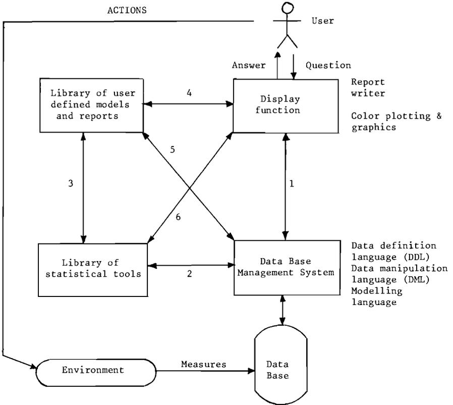
Fig. 1. The main functions of OPTRANS
