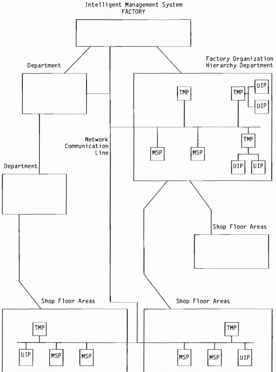
Figure 3-1: IMS System Architecture
